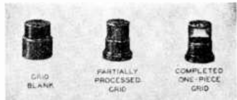
Fig. 8—Fabrication of one-piece grid.
