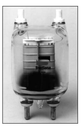
he Svetlana<sup>TM</sup> 833A is a medium-mu power triode intended for use in RF amplifier, oscillator, or class B modulator service. The Svetlana 833A features rugged construction for high power RF transmitter applications. The envelope is fabricated from hard glass intended specifically for the high-temperature operation of transmitting tubes.
