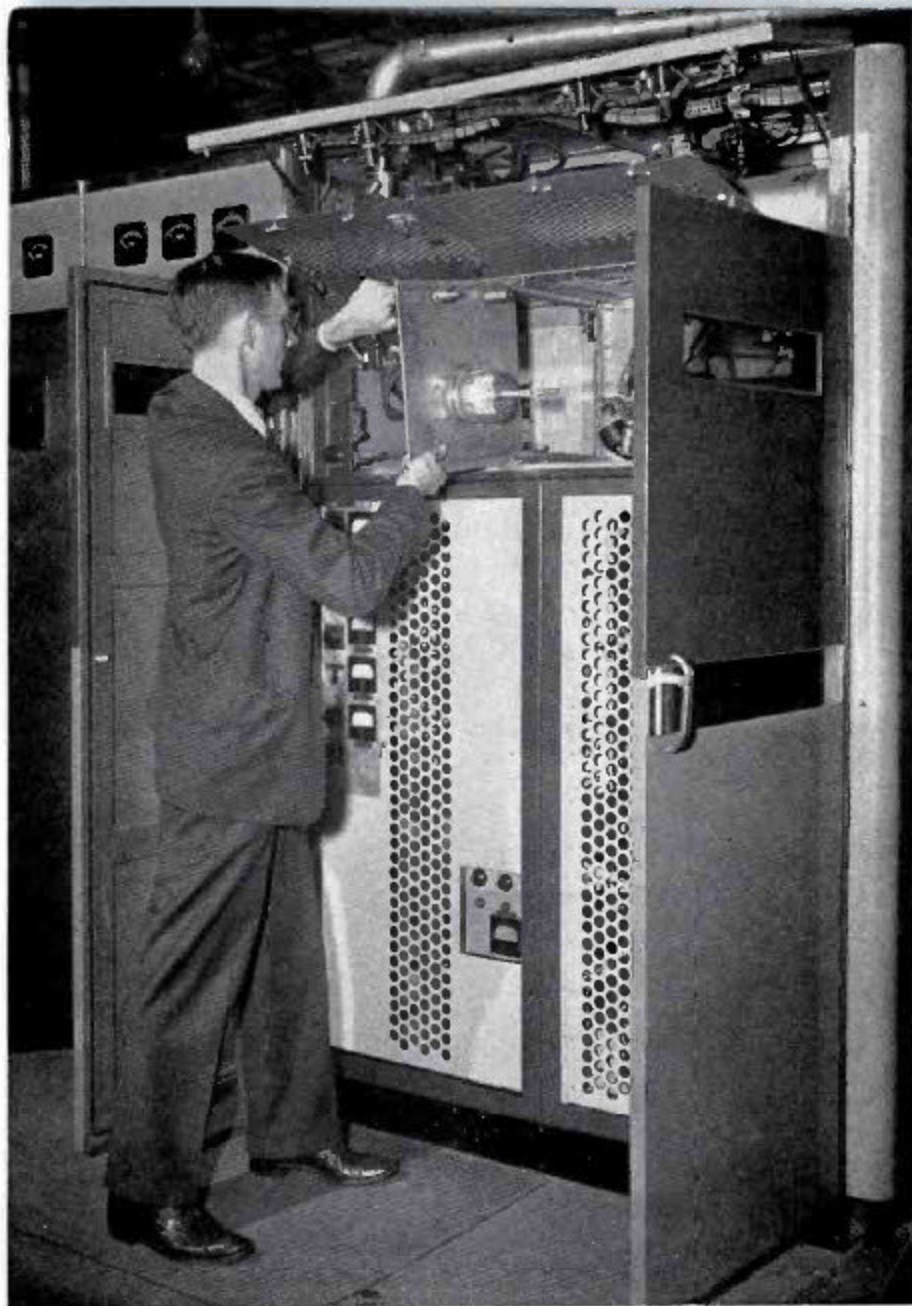
FIG. 1. The 8D21 tubes in the TT-5A transmitter are mounted on "tube plates" which can be easily removed whenever it is necessary to make a quick tube change.
