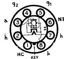
The BRIMAR type 35L6GT is an indirectly heated beam tetrode for use in the output stages of A.C./D.C. equipments where the operating voltages are low.
