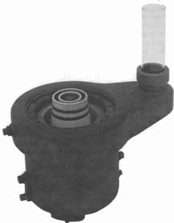
Figure 70. 4CV35,000A tetrode mounted in BR-200 boiler.
