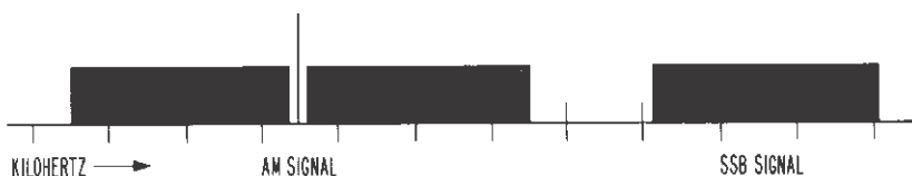
Figure 43. Relative spectrum space occupied by AM signal and SSB signal modulated by frequencies of 200 to 3000 Hz.
