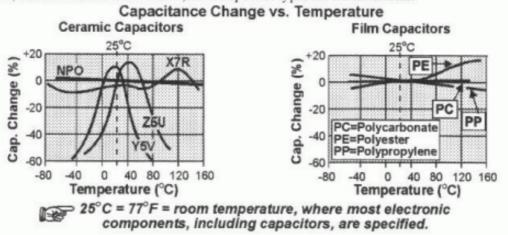
Title: Handyman's Guide to Capacitors Author: Paul Harden NA5N Page 3 of 6 GQRP Club Datasheet The most common ceramic/monolithic ceramics are X7R, Z5U and Y5V. The Z5U and Y5V have a large temperature coefficient (and a large dissipation factor -- see below) and should not be used in frequency critical circuits or for coupling between stages. They are suitable for other general purpose applications and for DC and bypassing caps.
