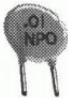
**Disk Ceramics** consist of two metallic plates separated by a ceramic dielectric, whose area and spacing determines the capacitance. These caps are low cost and suitable for many applications. Their main disadvantage is high capacitance changes
