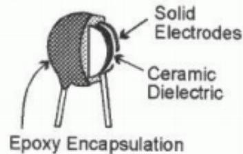
with temperature (high temperature coefficient), except for the "NPO" varieties that are temperature stable. These caps are the most commonly used for general purpose circuits, but the *non-NPO* types should be avoided in frequency determining circuits.
