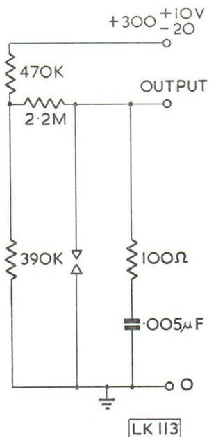
In order to prevent spurious counting due to contact bounce, it is essential to precede the integrated pulse drive LK.105 with a quenching circuit.
