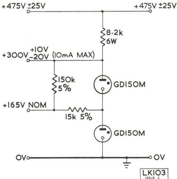
The above circuit uses two GD.150M tubes to provide a stabilized +300 V supply from +475 V. The +165 V supply is used for trigger bias with GTE.175M trigger tubes in Dekatron coupling circuits.
