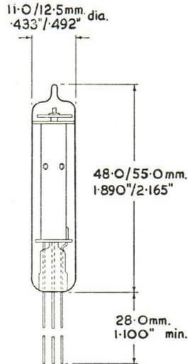
*N.B.*—To prevent damage to the tube, the leads should not be soldered or bent nearer than 5 mm. ( $\frac{1}{4}$ " ) to the glass seal.
