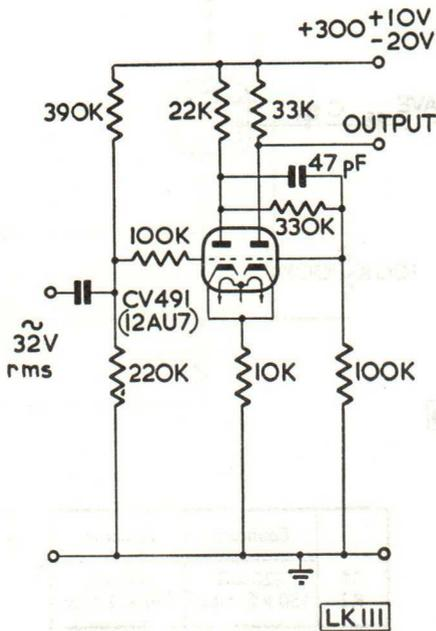
In the continuous sine-wave drive circuit LK.104 the correct phase relationship is not achieved until a few cycles have elapsed. In order to count trains of sine-waves it is necessary to convert them into pulses suitable for the integrated pulse drive LK.105. The above circuit fulfils this requirement.
