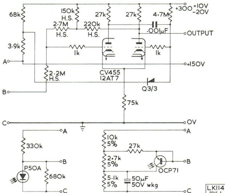
This circuit has been designed for use with either a P50A, germanium junction photo-cell, or an OCP71, photo-transistor. A positive going pulse is produced at the output whenever the light focused on the cell is interrupted. This pulse is suitable for driving the cold-cathode coupling circuit LK.108. The 150 V supply rail should be stabilized and may be obtained from the stabilizing circuit LK.103.
