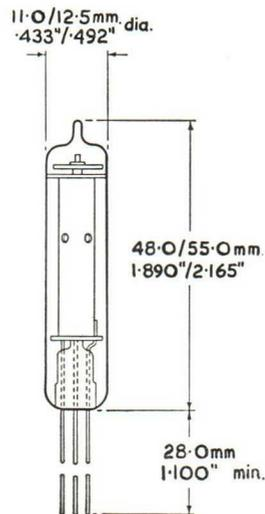
N.B.—To prevent damage to the tube, the leads should not be soldered or bent nearer than 5 mm. ( $\frac{1}{4}$ " ) from the glass seal.
