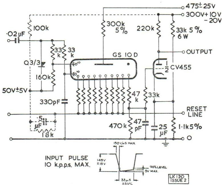
The grid and cathode of the pulse amplifier are used as a limiting diode for the GS10D output cathode voltage.
