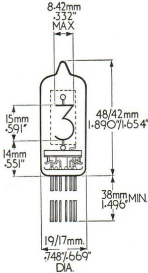
N.B.—To prevent damage to the tube, the leads should not be soldered or bent nearer than 5 mm ( $\frac{1}{4}$ " ) from the glass seal.
