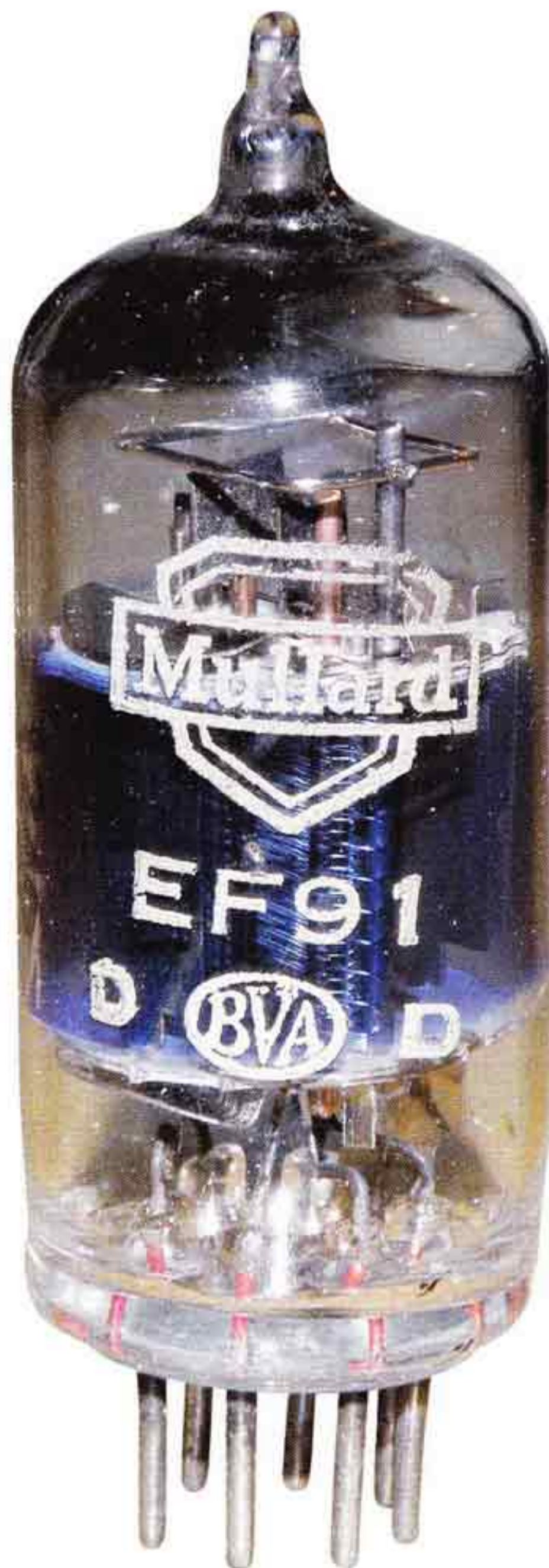
Figure 2: The 'classic' pose of the Mullard EF91, showing the bluish colour band around the anode structure of the valve.
