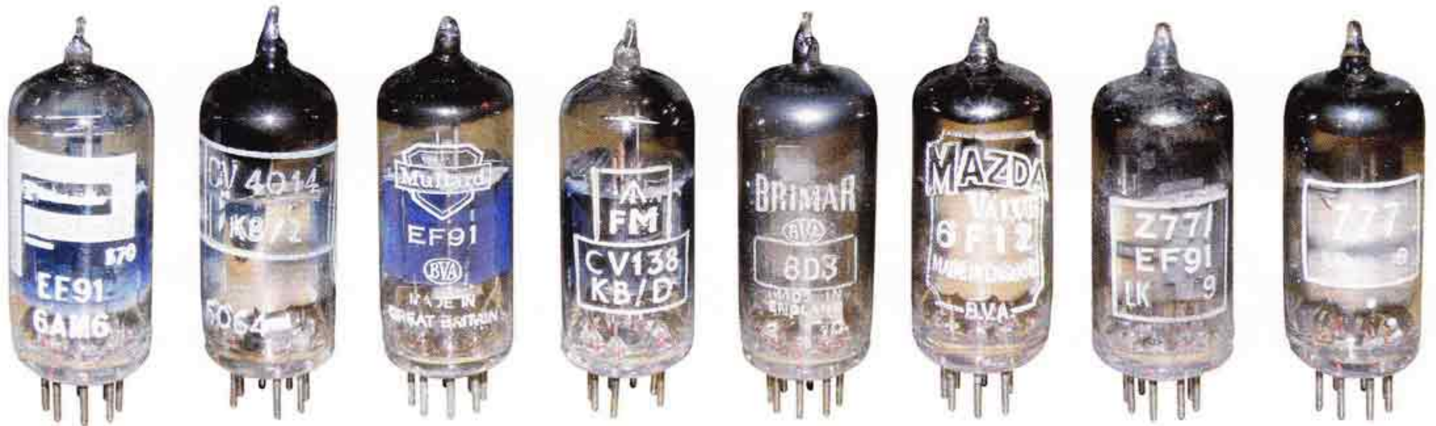
Figure 1: An 'identity parade' line up of EF91s and several of its aliases, including the CV138 and CV4014 service equivalents.
