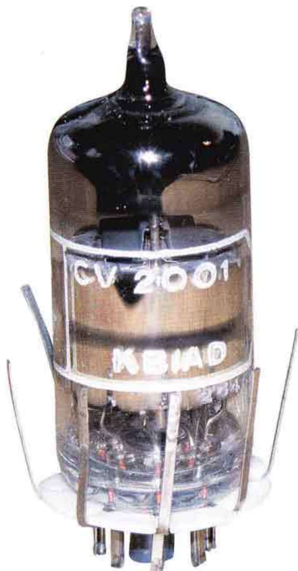
Figure 11: Photo of the CV2001 valve, or more accurately this seems to be the code for the valve-plus-socket assembly.
