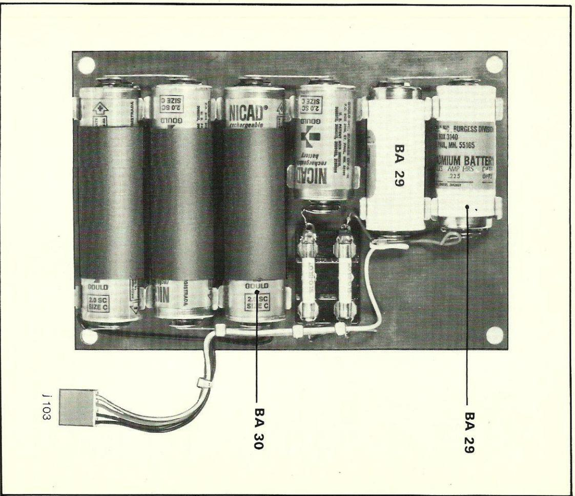
Figure 6 - Ensemble batteries rechargeables
