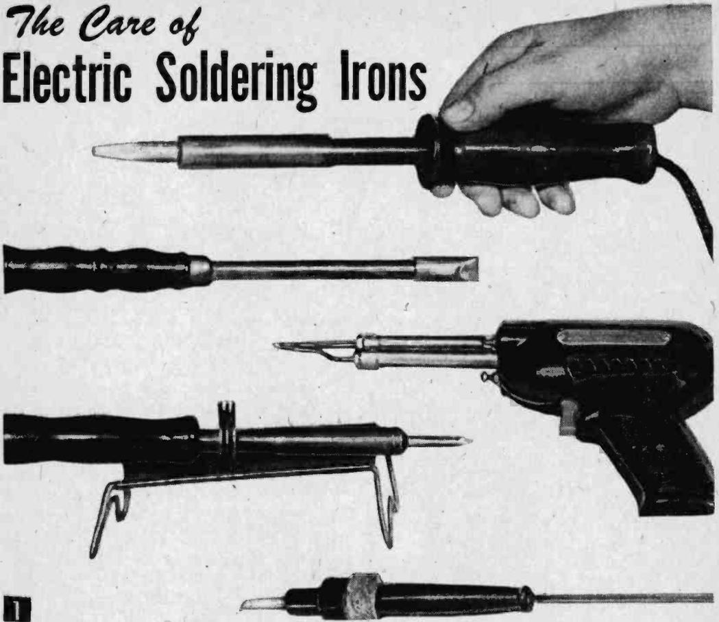
An assortment of irons; ratings range from 20 to 135 watts. All have universal shaped tips, or chisel points, except the gun-type (right center) which has a shorted turn, alloy-wire tip. Dual-rated for 100-135 watts, the gun-type iron is designed for instant-heat electronics work. The pencil iron (lower right) is for use in cramped quarters.
