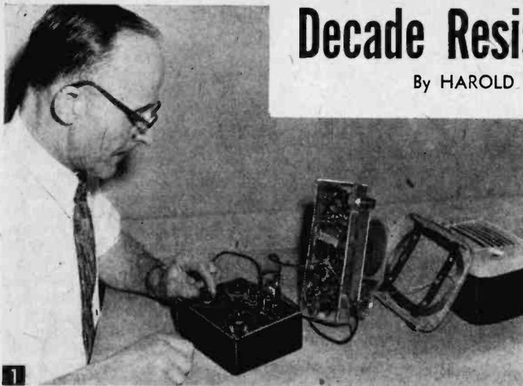
Decade resistance box in use in radio servicing job. Various values of resistance are being applied across terminals where a defective resistor was formerly soldered, and which is now unidentifiable due to extreme heating.
