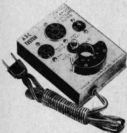
A radio and television tube filament checker such as the one shown above will test TV picture tubes as well as ordinary vacuum tubes.
