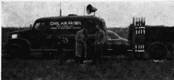
An excellent example of CAP ability to adapt material at hand for maximum versatility is this combination ambulance-radio station-equipment trailer maintained by the O'Hare CAP Squadron for emergency use in the Chicago area.
