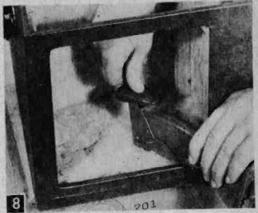
8 Attaching fiber glass insulation to insides of speaker compartment with stapler-tacker. Insulation on sides extends only up to baffle board supports.
