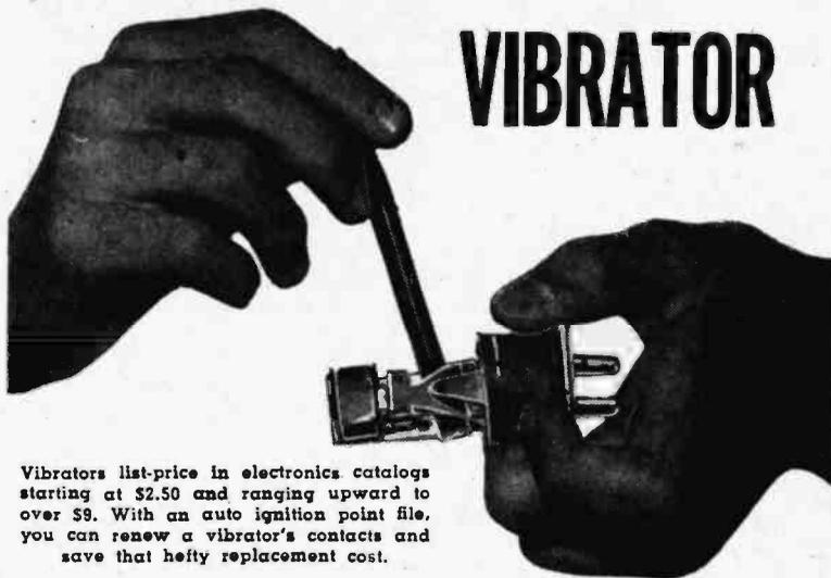
Vibrators list-price in electronics catalogs starting at \$2.50 and ranging upward to over \$9. With an auto ignition point file, you can renew a vibrator's contacts and save that hefty replacement cost.
