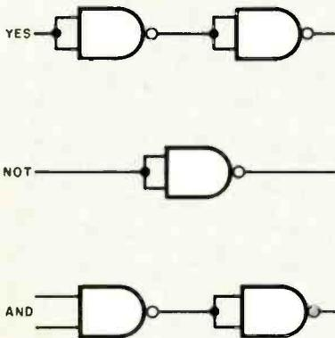
Fig. 3. Using NAND gates to simulate other gates. At top, YES; middle, NOT; bottom, AND.
