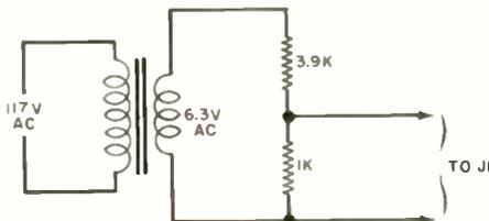
Fig. 5. Schematic diagram of a suitable test source to verify proper circuit operation.
