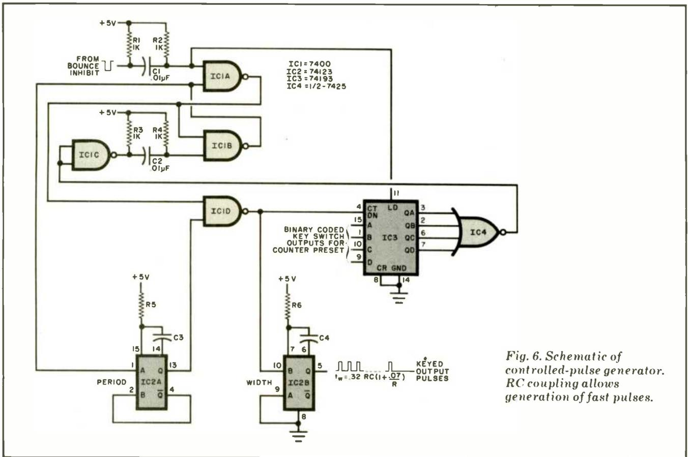
Fig. 6. Schematic of controlled-pulse generator. RC coupling allows generation of fast pulses.
