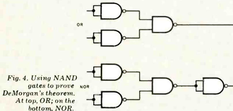
Fig. 4. Using NAND gates to prove DeMorgan's theorem. At top, OR; on the bottom, NOR.
