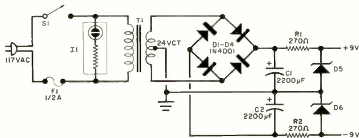
Fig. 2. Ac power supply features zener diode regulation.
