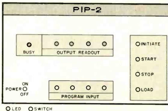
Fig. 2. Front-panel arrangement to facilitate operation of PIP-2.
