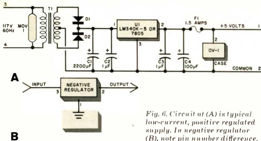
Fig. 6. Circuit at (A) is typical low-current, positive regulated supply. In negative regulator (B), note pin number difference.
