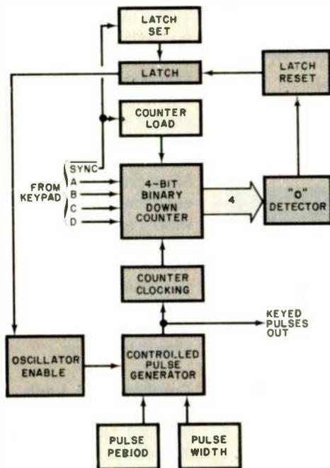
Fig. 5. Function diagram for a controlled-pulse generator.
