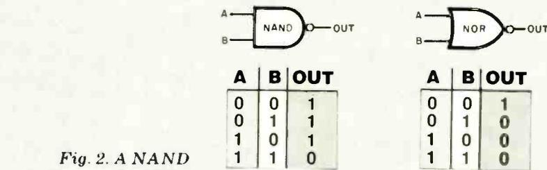
Fig. 2. A NAND gate and a NOR gate, with their respective truth tables below.
