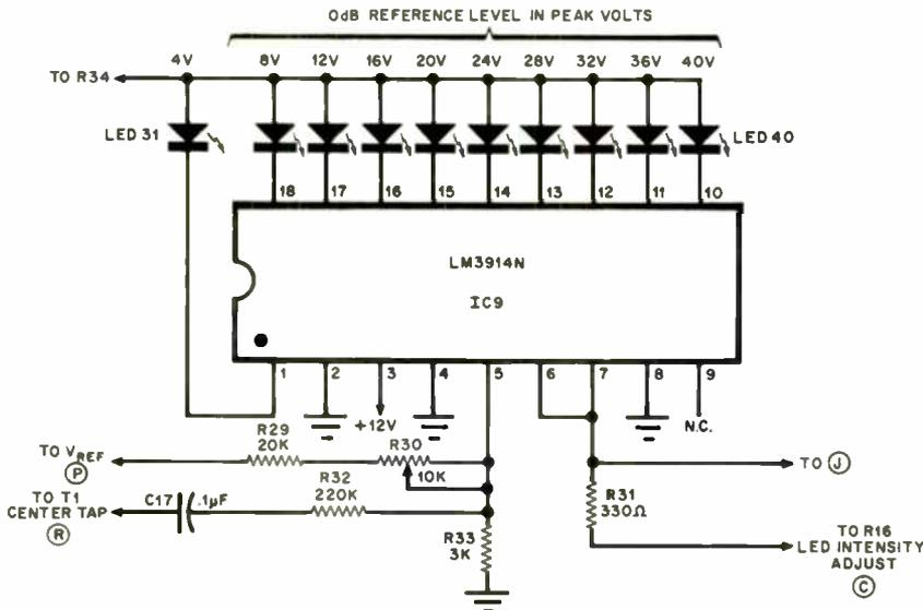
Fig. 4. Schematic diagram of the project's 0-dB Level Indicator.
