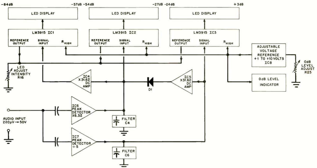
Fig. 2. Block diagram of one channel of the Wide-Range Audio Meter.
