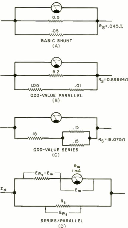
Fig. 2. Various configurations for using shunts with meters.
