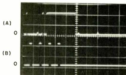
Fig. 7. Scope trace (A) shows switch bounce, while (B) shows four pulses initiated by switch closure. Sweep time is 50  $\mu$ s/div.
