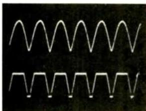
Fig. 7. Bottom waveform shows how a regulator "limits" peaks on rectified pulsating dc.
