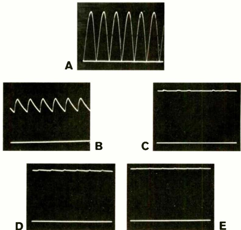
Fig. 5. How capacitors smooth waveform. Lower trace is zero volts. (A) is full-wave dc without filter; (B) has 150- $\mu\text{F}$  capacitor; (C) 2000  $\mu\text{F}$ ; (D) 5000  $\mu\text{F}$ ; (E) 18,000  $\mu\text{F}$ .
