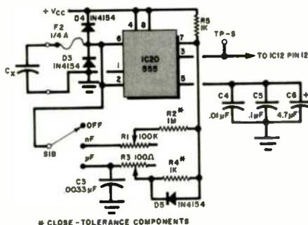
Fig. 2. Input stage has free-running 555 timer.
