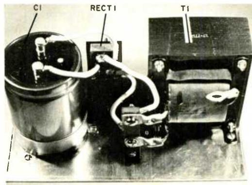
Fig. 1. Basic 8-volt, 15-ampere dc source. Note heavy wiring between elements.
