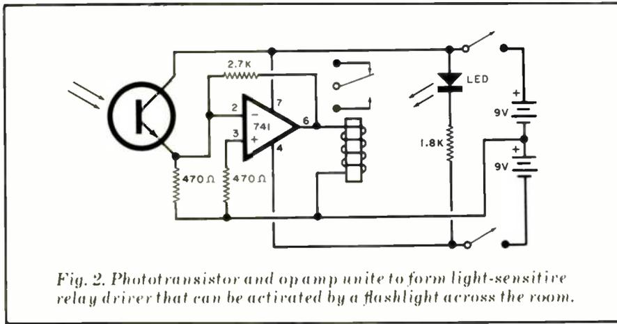
Fig. 2. Phototransistor and op amp unite to form light-sensitive relay driver that can be activated by a flashlight across the room.
