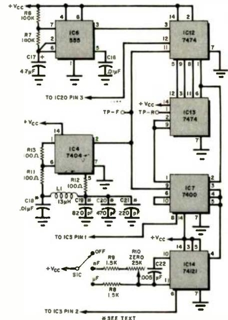
Fig. 3. Oscillator, sync., and reset circuits.
