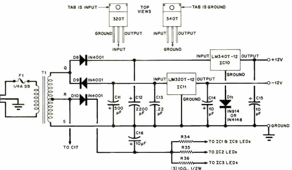
Fig. 5. Schematic diagram of the supply that satisfies the power requirements of a two-channel version of the Wide-Range Audio Meter.
