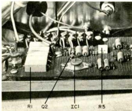
**Fig. 4. Typical regulated supply for 5 V at 10 A. Circuit includes a line over-voltage protector and current limiting regulator. Photo at top shows top of chassis. Underneath view is directly above.**
