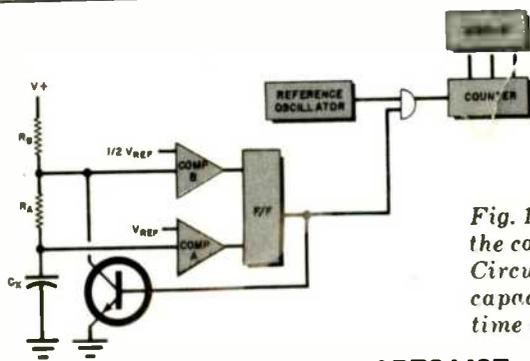
Fig. 1. Block diagram of the capacitance meter. Circuit determines unknown capacitance by measuring time it takes to discharge.
