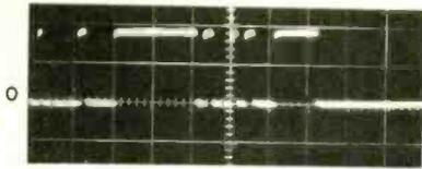
Fig. 1. Pulse train resulting from switch contact bounce. Sweep time is 50  $\mu$ s/div.
