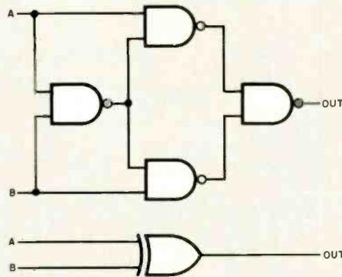
Fig. 5. The combinational circuit at top provides an Exclusive-OR, as shown in the middle. The truth table is below.
