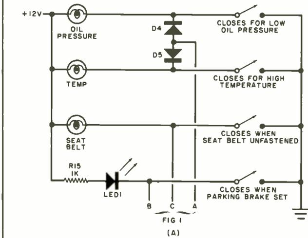
Fig. 2 Function sensing is shown at (A) while (B) shows how dc power is applied to the alarm circuit.
