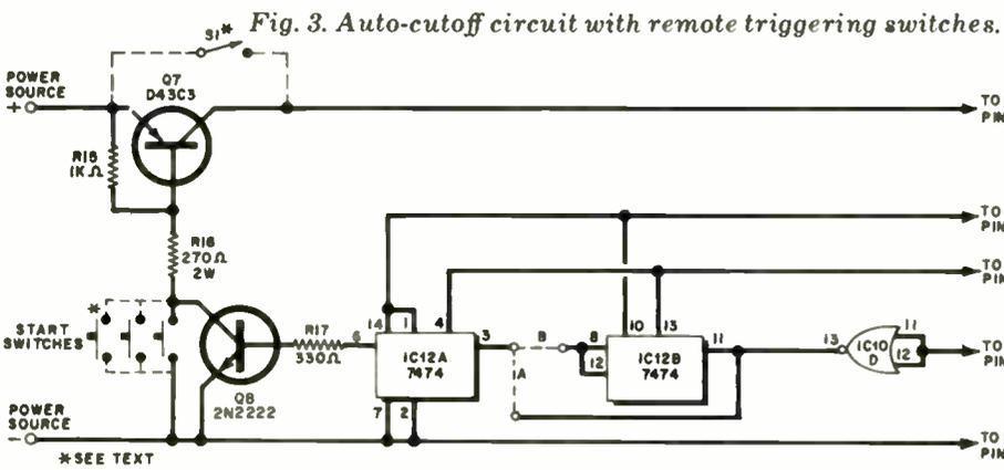
Fig. 3. Auto-cutoff circuit with remote triggering switches.
