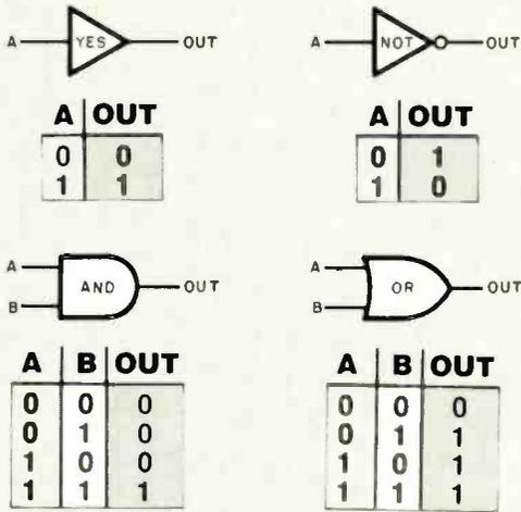
Fig. 1. The four basic logic gates: YES, NOT, AND, OR.
