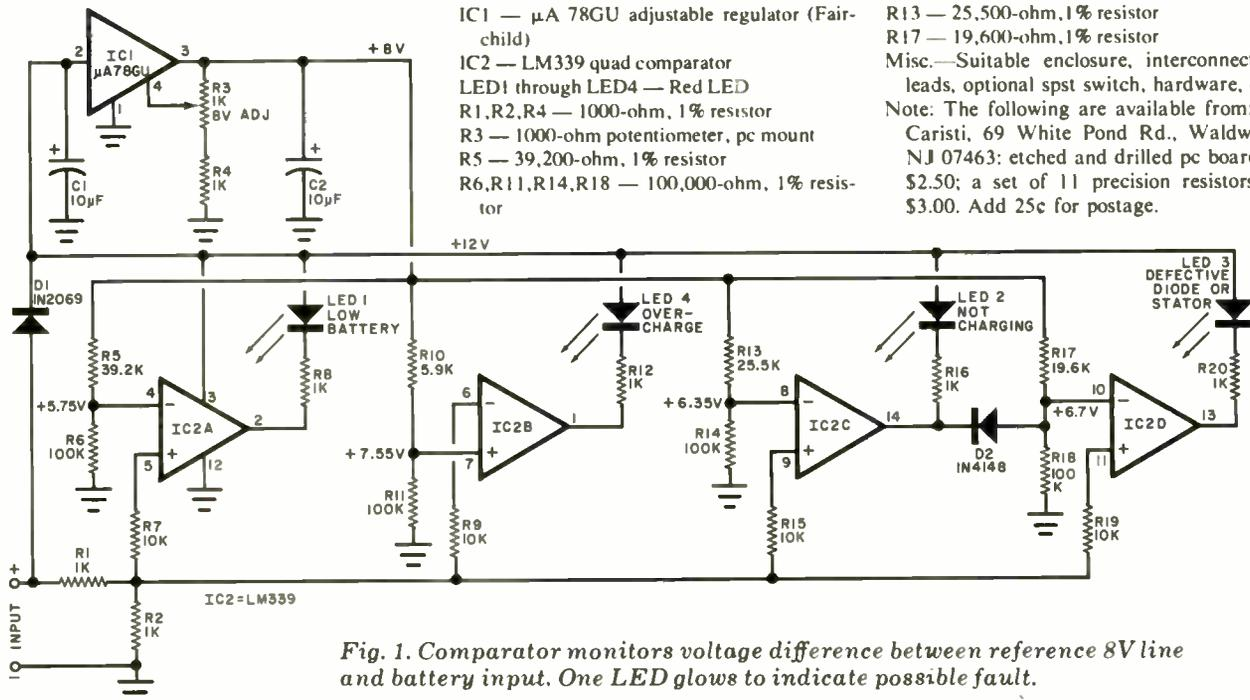
Fig. 1. Comparator monitors voltage difference between reference 8V line and battery input. One LED glows to indicate possible fault.
