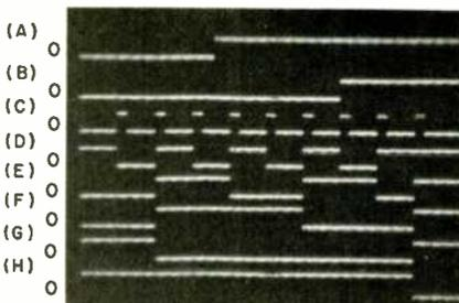
Fig. 8. Nine pulses generated by key switch closure (50 ms/div): (A) key closure; (B) sync; (C) outputs of 74123; (D) output QA; (E) output QB; (F) output QC; (G) output QD; all of IC3; and (H) latch input to IC1D.
