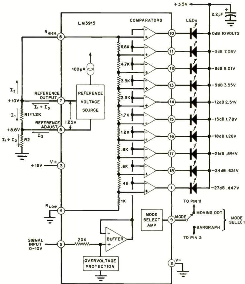
Fig. 1. Functional diagram of the LM3915 LED driver IC.
