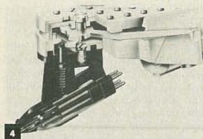
A closeup view of the Ortofon ULM cartridge mounted in the lightweight headshell of the Dual model 606 is shown in Fig. 4. While the headshell of the arm is permanently affixed to the arm itself, the cartridge can be easily removed and, if desired, other cartridges having standard 1/2-inch mounting centers can be
