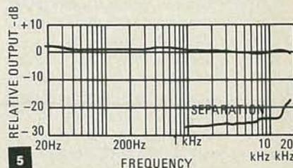
Frequency response of the ULM cartridge is plotted from 20 Hz to 20 kHz (the available frequencies on our test record) in Fig. 5. To obtain that response, we had to add about 200
