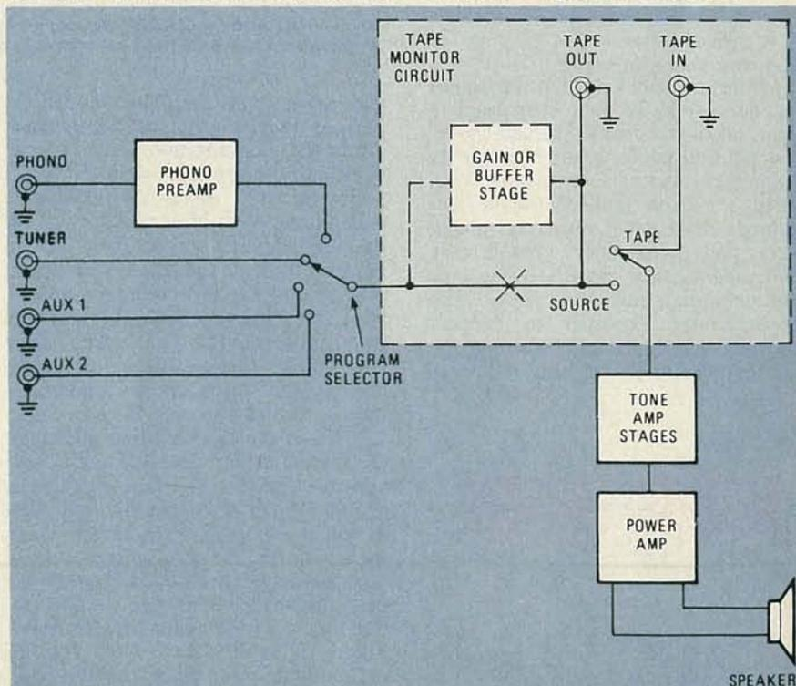
FIG. 1—TAPE MONITOR CIRCUIT is actually a point of access to the signal path within the preamplifier. Although originally used for connection to a tape deck, many signal processors and add-on accessories can be connected to the system at this point.
