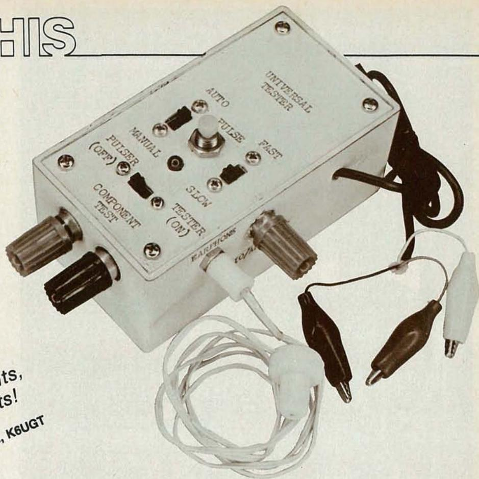
THE UNIVERSAL TESTER IS USED TO troubleshoot digital logic and counting circuits. It performs useful checks of resistors, capacitors, transistors, and most other electronic components. It can also be used to test audio and AM radio circuits.
