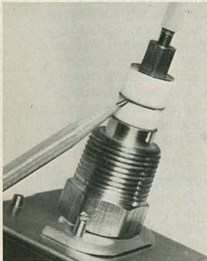
THE GUARD-RING midway down the insulator is connected to the electric line and to the input of the relay coil that holds the circuit closed. When the insulator is clean, it has no effect. If conductive contamination builds up on the insulator, it shunts current around the relay to cause it to drop out, stopping the burner.
