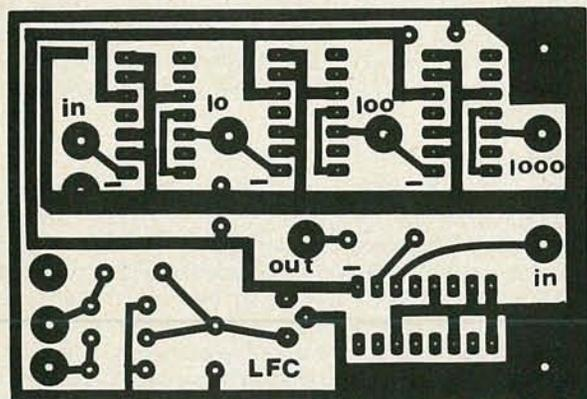
FIG. 3—FOIL PATTERN for the printed-circuit board. Circuit is so simple that using stripboard or perforated board and point-to-point wiring will be a cinch.
