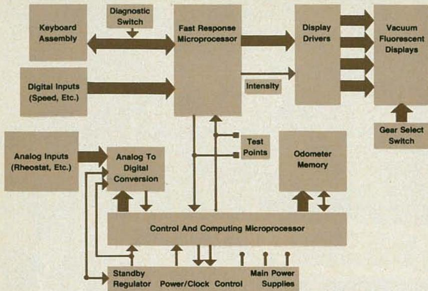
**INSTRUMENT CLUSTER** of 1981 Chrysler Imperial uses two microprocessors. The first interfaces primarily with the automobile; the second with the driver.
