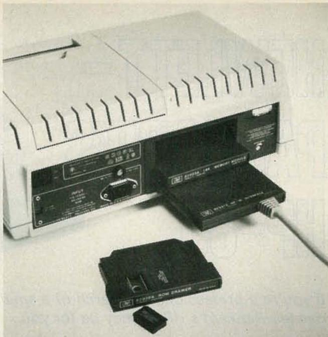
EXPANSION AND I/O modules plug into rear of *HP-85*.
