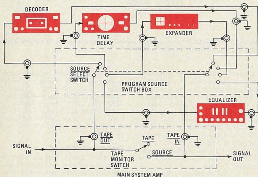
FIG. 8—SWITCH BOX allows you to select which of several devices will be placed in tape monitor loop. Setup shown allows only one device at a time to be used.
