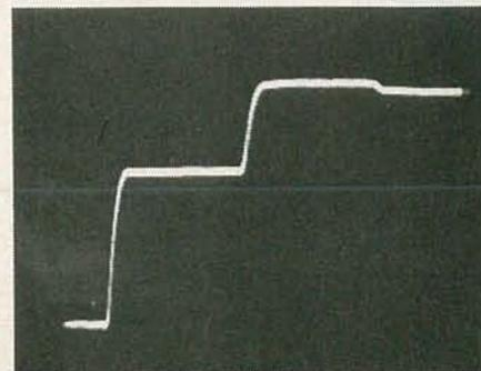
FIG. 5—OPEN-LOAD curve. In theory, incident and reflected pulses are equal.
