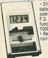
• 3 1/2 digits display • 200 hours 9V battery life • Auto zero; polarity; overrange indication • 100MV DC F.S. sensitivity • 19 ranges and functions • D.C. volt: 0.1 MV to 1000V • A.C. volt: 0.1 V to 600 V • Resistance: 0.1Ω to 20 MΩ • D.C. current: 0.01 A to 100 MA
