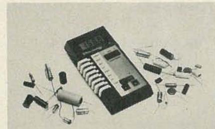
DIGITAL CAPACITANCE METERS come in a variety of sizes. This one, the Data Precision 938, fits in your pocket.
