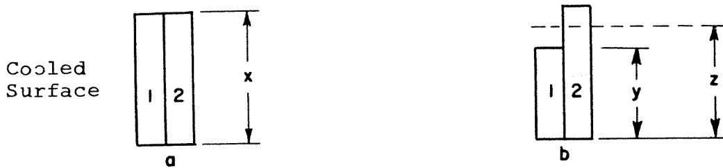
Fig. 6 Development of Temporary Stresses in Glass During Cooling Below the Strain Point.
