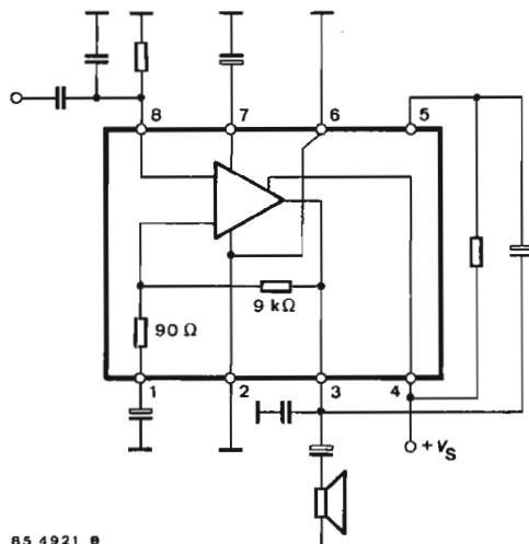
Fig. 1 Block diagramm and pin connections
