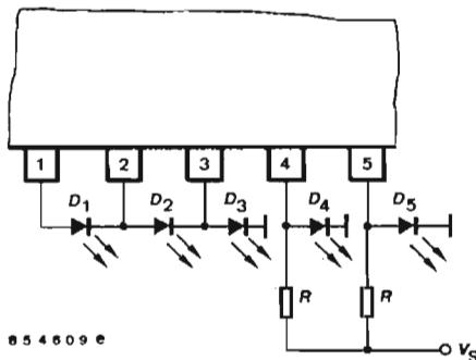
Fig. 4 3 LEDs in series
