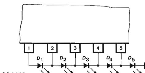
Fig. 2 Series circuit for 5 LEDs
