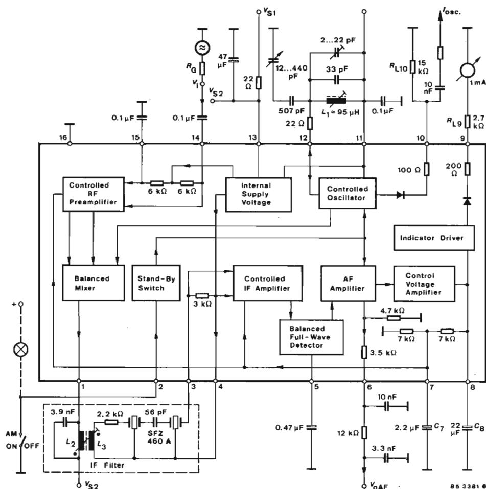
Fig. 2 Test circuit
