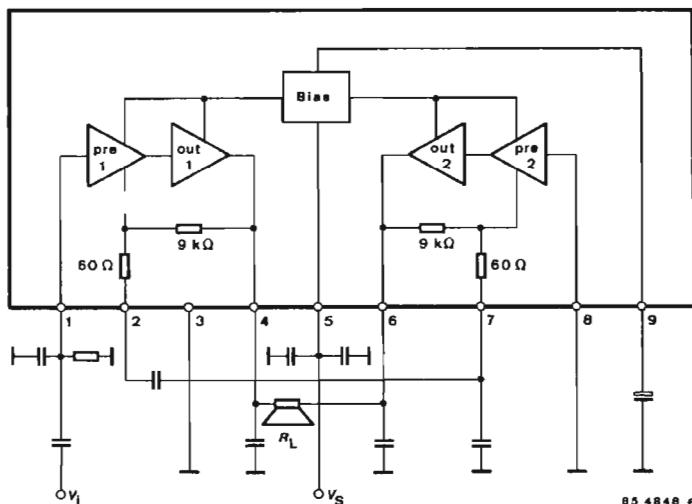
Fig.1 Block diagram and pin connections
