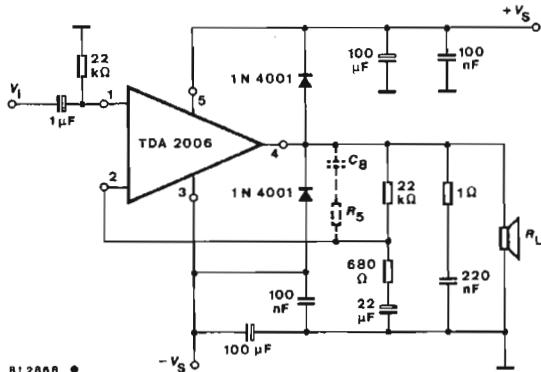
Fig. 18 AF amplifier with split power supply
