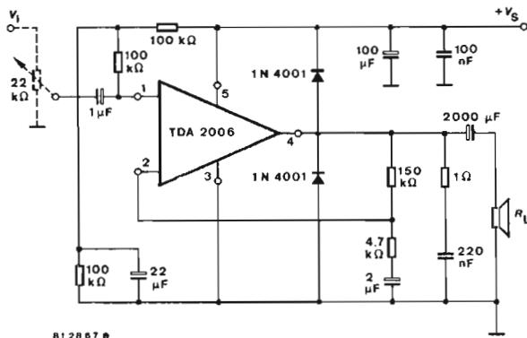
Fig.16 AF amplifier with single power supply
