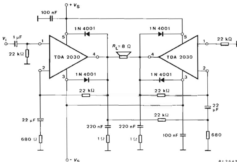
Fig.17 AF amplifier with split power supply
