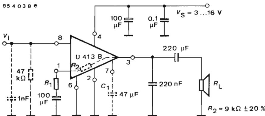
Fig. 2 Test circuit for:  $P_o$ ,  $P_{\text{tot}}$ ,  $d$ ,  $V_{no}$ ,  $B$ ,  $G_v$  and application note
