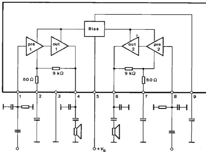
Fig.1 Block diagram and pin connections
