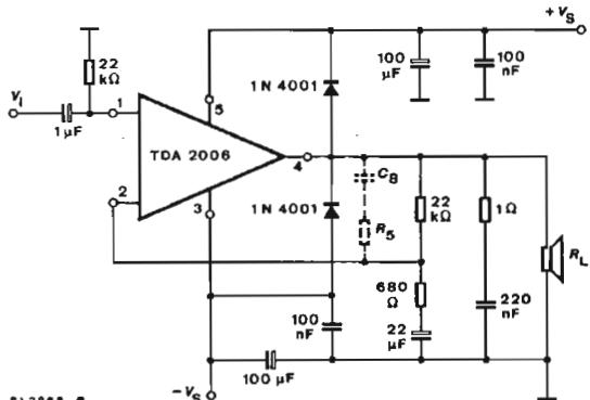
Fig. 3 Test circuit
