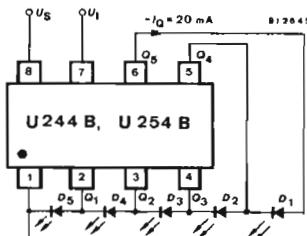
Fig. 2 Bar display with 5 LEDs
