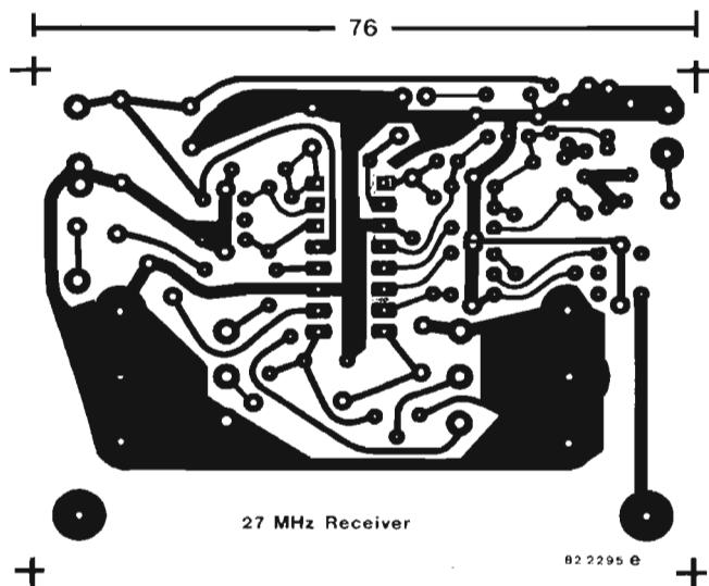
Fig. 13 Layout of circuit board (soldered side) for 27 MHz-receiver
