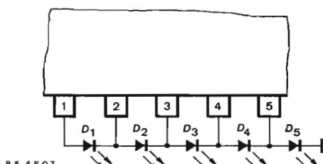
Fig. 2 Series circuit for 5 LEDs
