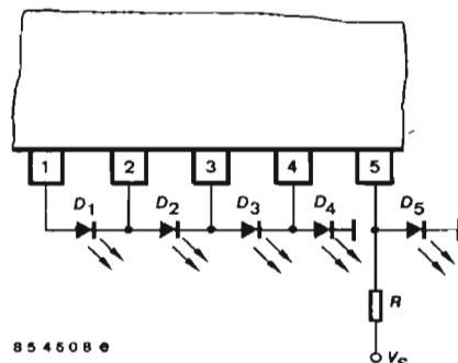
Fig. 3 4 LEDs in series
