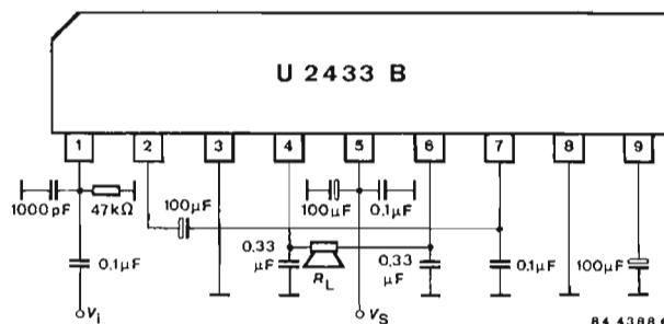
Fig. 2 Test circuit
