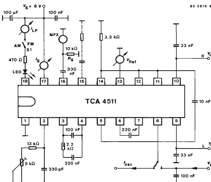
Fig. 2 Test circuit
