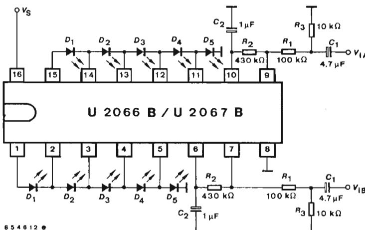
Fig. 7 Circuit with  $G_v = 4.3$
