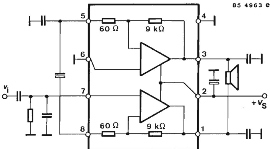
Fig.1 Block diagram and pin connections
