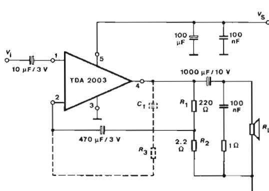
$$R_3 = 20 \cdot R_2; C_1 = \frac{1}{2\pi \cdot B \cdot R_1}$$
