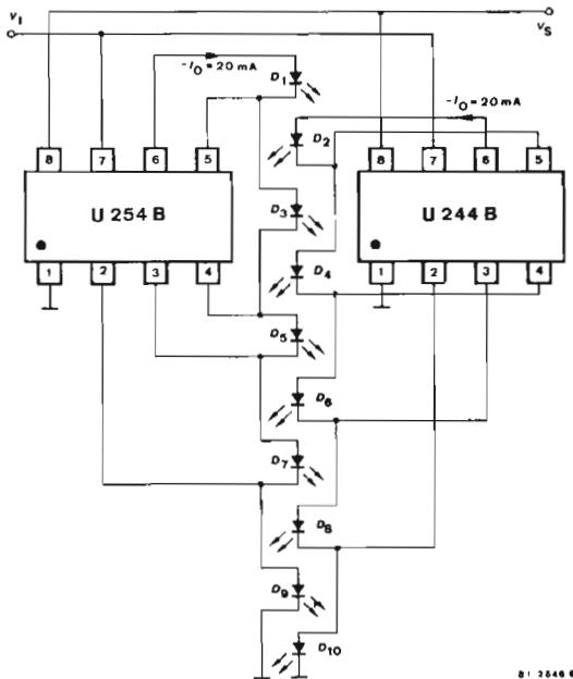
Fig. 3 Bar displays with 10 LEDs
