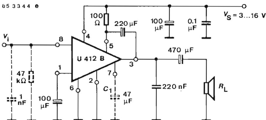
Fig. 2 Test circuit for:  $P_o$ ,  $P_{tot}$ ,  $d$ ,  $V_{no}$ ,  $B$ ,  $G_v$  and application note
