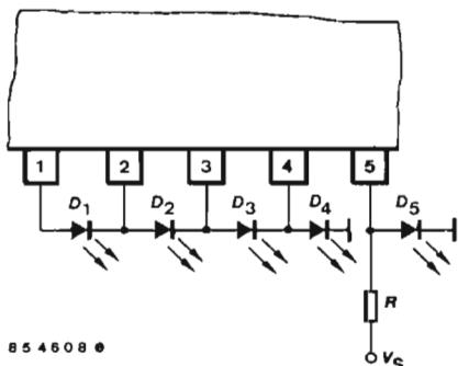
Fig. 3 4 LEDs in series
