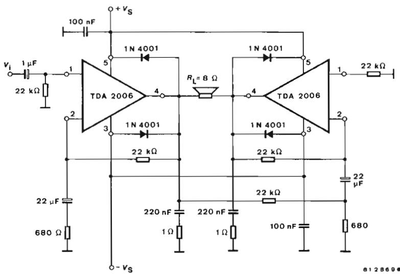
Fig.17 Bridge amplifier with split power supply
