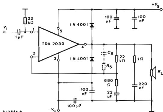
Fig. 18 Bridge amplifier with split power supply
