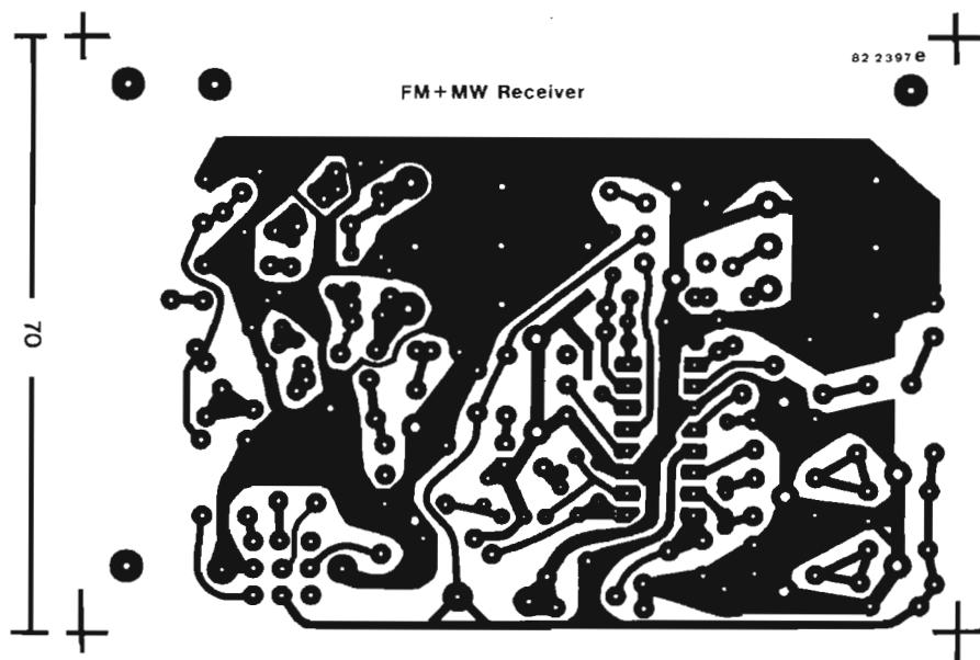
Fig. 10 Layout of circuit board (soldered side) of the FM-/AM-receiver
