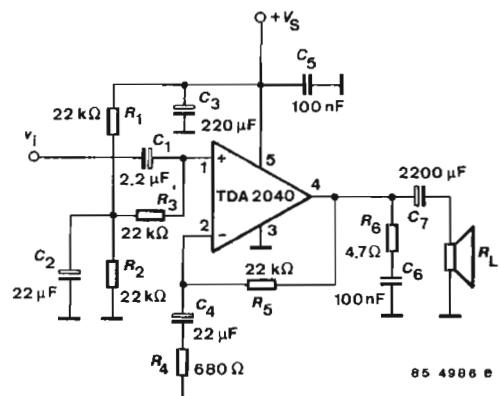
Fig. 4 Amplifier with single supply (\*)
