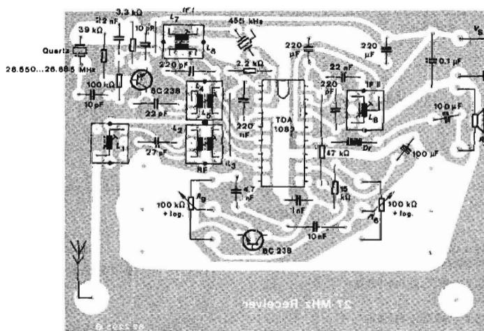
Fig. 14 Printed board with components for 27 MHz-receiver
