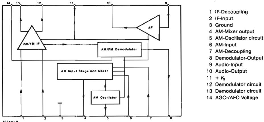
Fig. 1 Block diagram and pin connections
