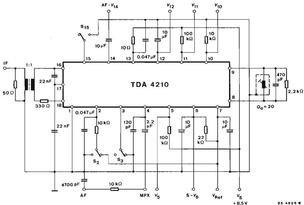
Fig. 2 Test circuit
