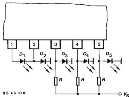
Fig. 5 2 LEDs in series
