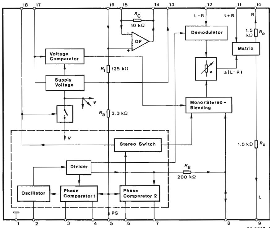
Fig.1 Block diagram and pin connections
