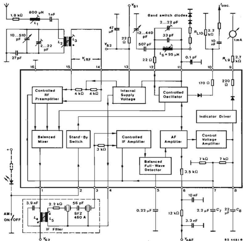
Fig. 1 Block diagram and application circuit
