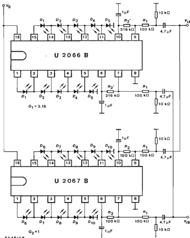
Fig. 8 Dual 10 LED control circuit
