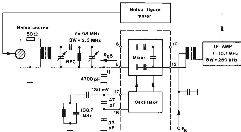
1) Mounted as close as possible between pin 6 and Ground
