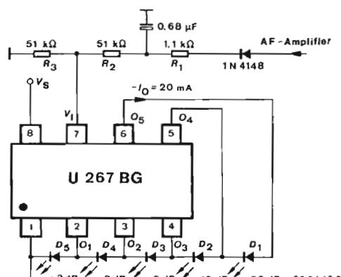
Fig. 5 Logarithmic AF recording level display with 5 LED's
