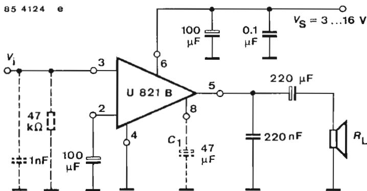
Fig. 2 Test circuit for:  $P_o$ ,  $P_{tot}$ ,  $d$ ,  $V_{no}$ ,  $B$ ,  $G_v$  and application note
