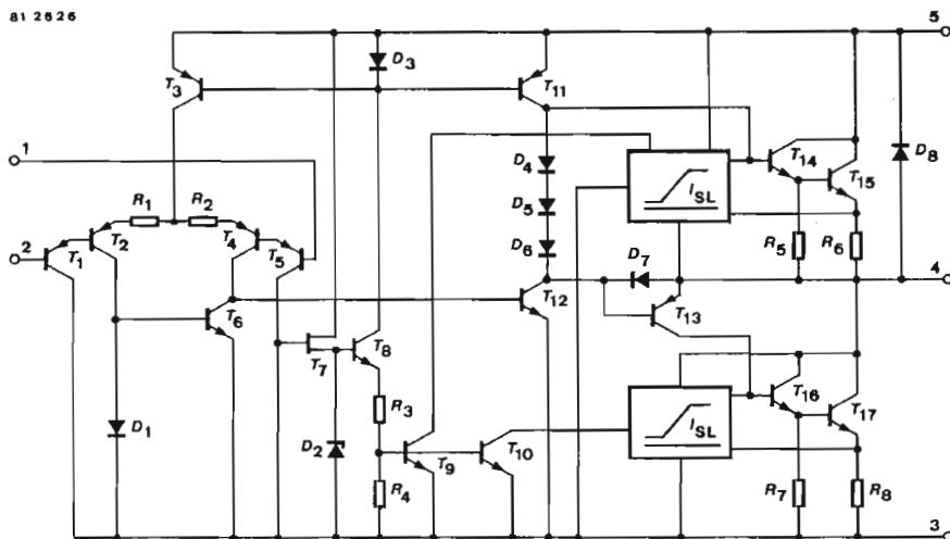
Fig. 1 Diagram and pin connections, Pin 3 connected with metallic surface
