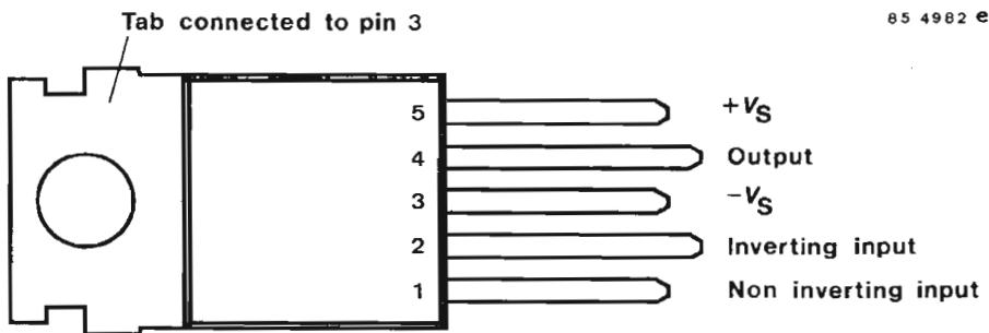
Fig. 1 Connection diagram (top view)
