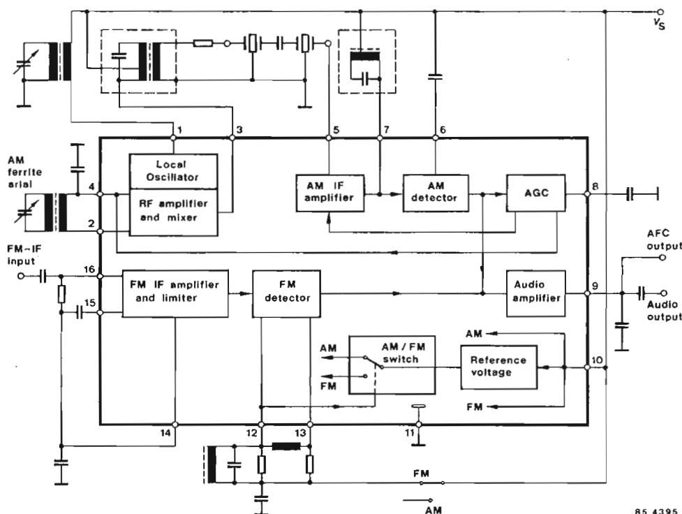
Fig.1 Block diagram and pin connections
