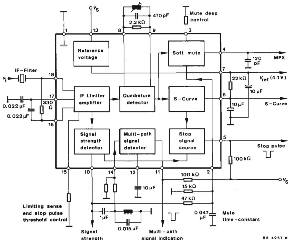
Fig. 1 Block diagram and application circuit
