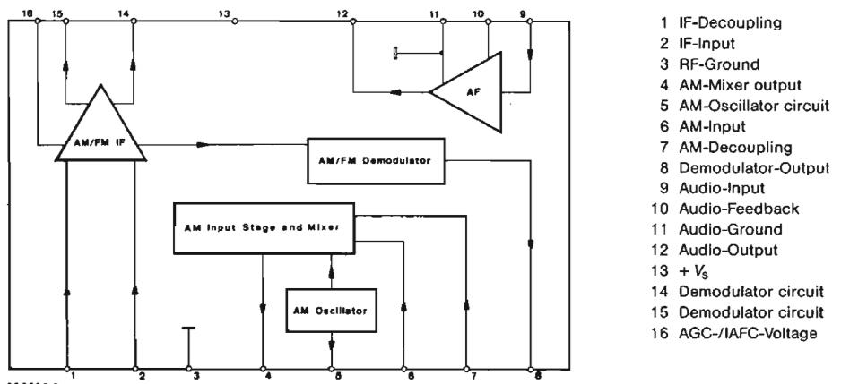
Fig. 1 Block diagram and pin connections
