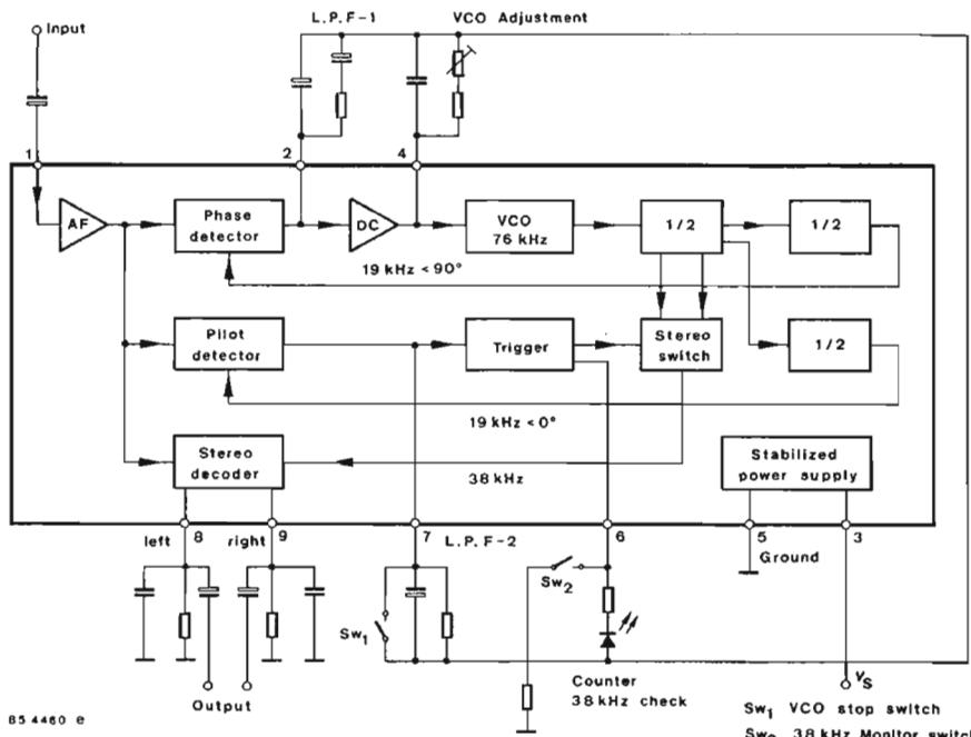
Fig.1 Block diagram and pin connections
