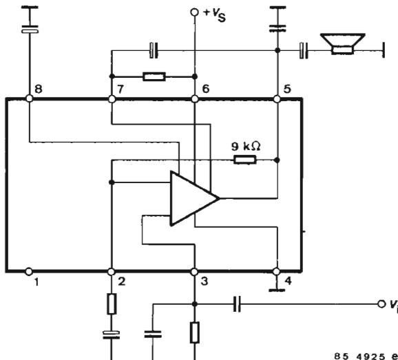
Fig. 1 Block diagram and pin connections
