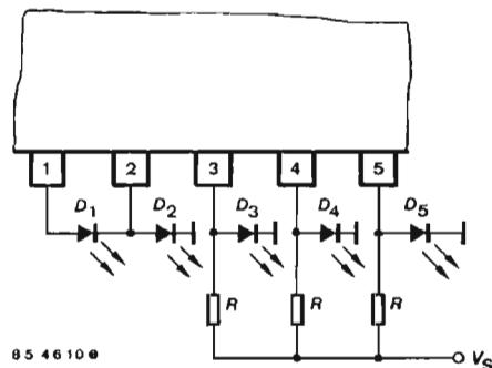
Fig. 5 2 LEDs in series
