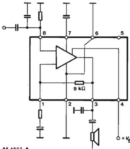
Fig. 1 Block diagramm and pin connections
