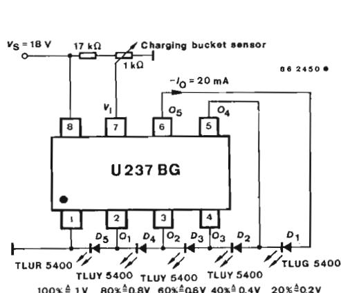
Fig. 4 Liquid level display with linear resistance pickup
