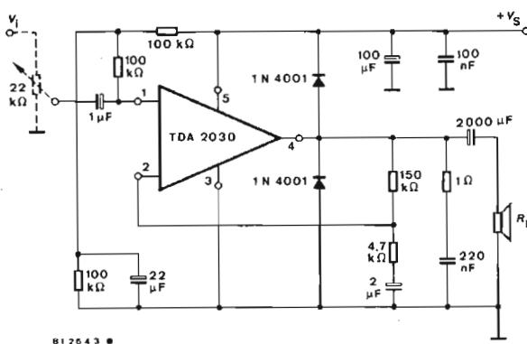
Fig.16 AF amplifier with single power supply
