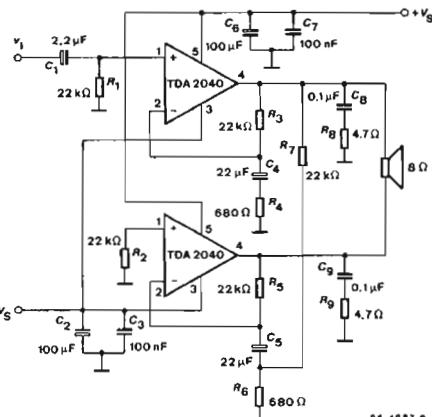
Fig. 5 30 W Bridge amplifier with split power supply
