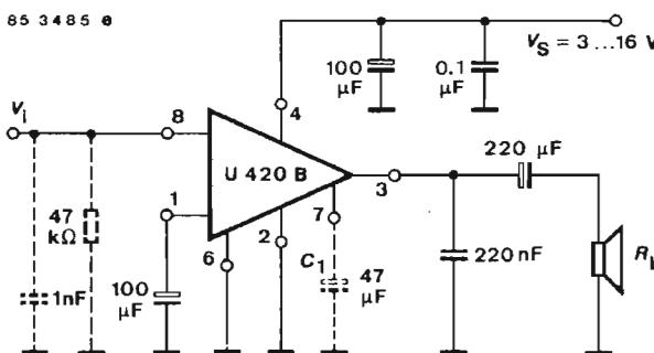
Fig. 2 Test circuit for:  $P_o$ ,  $P_{\text{tot}}$ ,  $d$ ,  $V_{\text{no}}$ ,  $B$ ,  $G_v$  and application note
