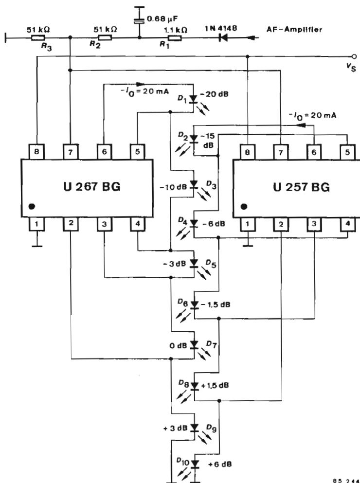
Fig. 6 Logarithmic AF recording level display with 10 LED's
