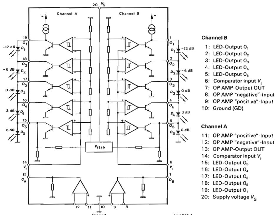
Fig. 1 Block diagram and
