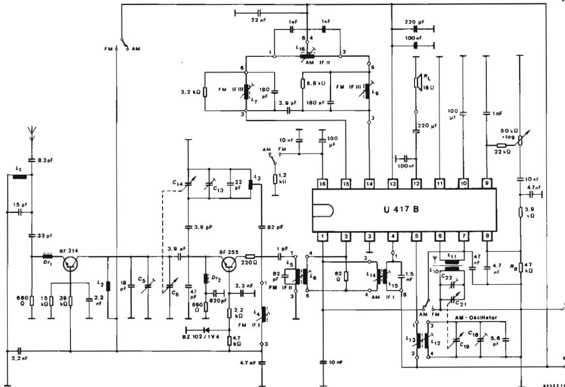
Fig. 2 FM-/AM-receiver circuit
