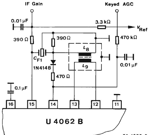
Circuit (section) from above diagram with keyed AGC
