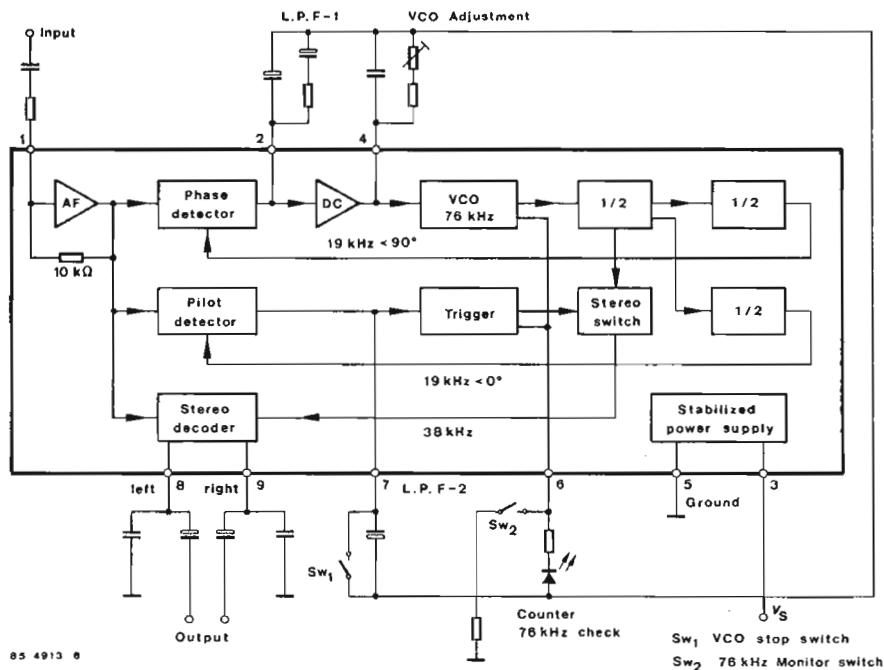
Fig.1 Block diagram and pin connections
