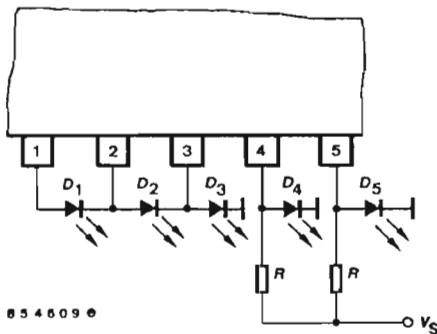
Fig. 4. 3 LEDs in series
