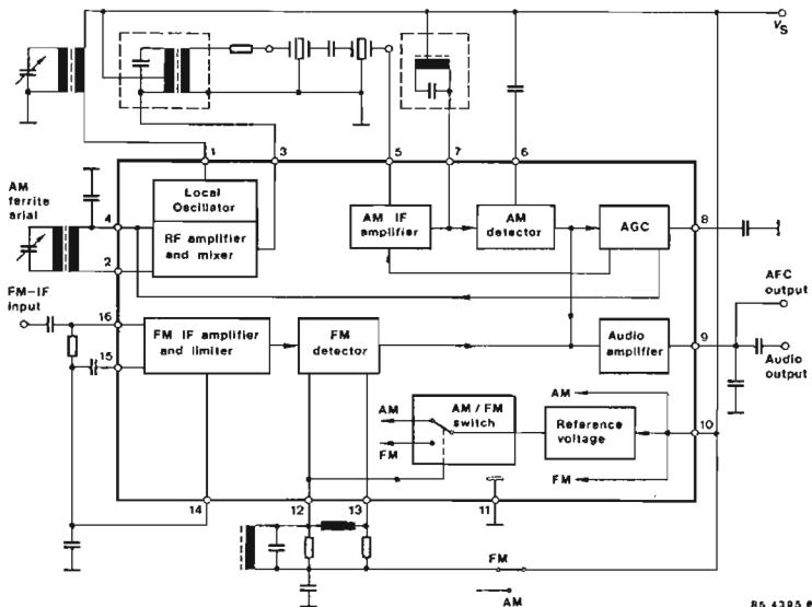
Fig.1 Block diagram and pin connections
