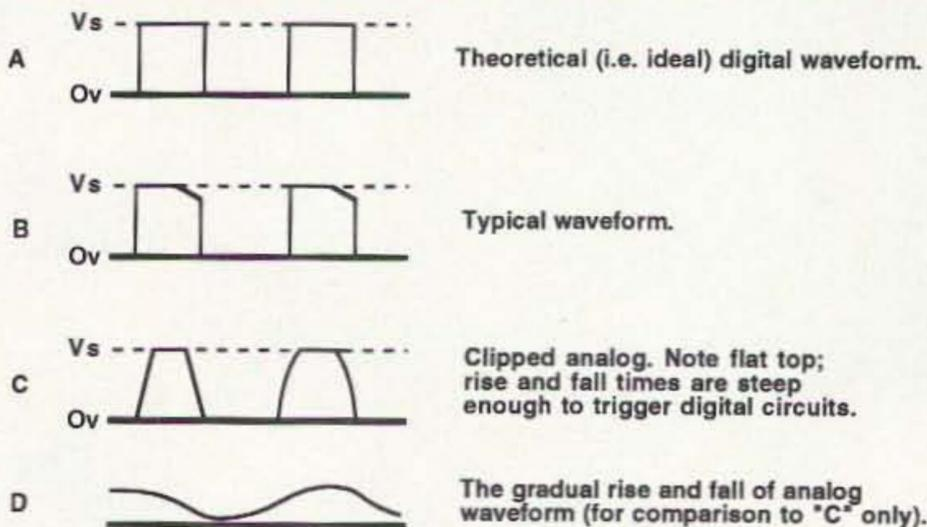
Figure 3. a) Theoretical (i.e. "ideal") digital waveform. b) Typical waveform. c) Clipped analog. Note flat top; also, rise and fall times ("up" and "down" ramps) are steep enough to properly trigger digital circuits. d) Note gradual rise and fall of analog waveform (for comparison only to diagram "c").
