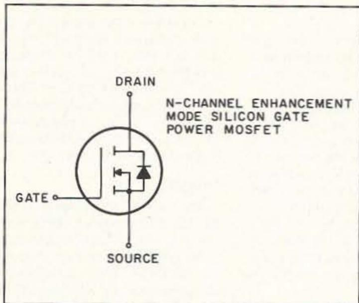
Figure 1. Schematic drawing for a power MOSFET.
