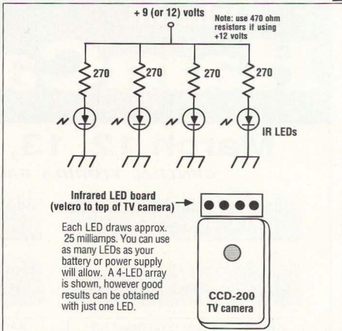
Figure 1. An array of high-output infrared LEDs mounted above the CCD-200 TV camera will provide enough illumination to light up a small room. Since the output is all in the infrared spectrum, the room will appear completely dark with the naked eye. For 9-volt operation use 270-ohm resistors; for 12 volts use 470 ohms.
