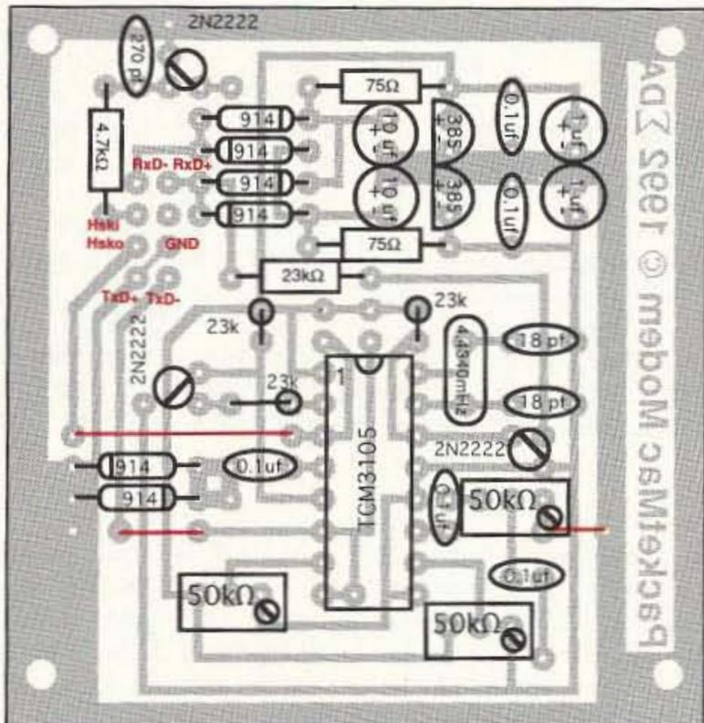
Figure 1. The corrected (and hopefully final) parts placement diagram of the PacketMac Modem showing the jumper wires as well as the new pad assignments (shown in red). Using these new pad assignments, just follow the wiring hookup chart in Figure 4 in the original article for the proper connections.
