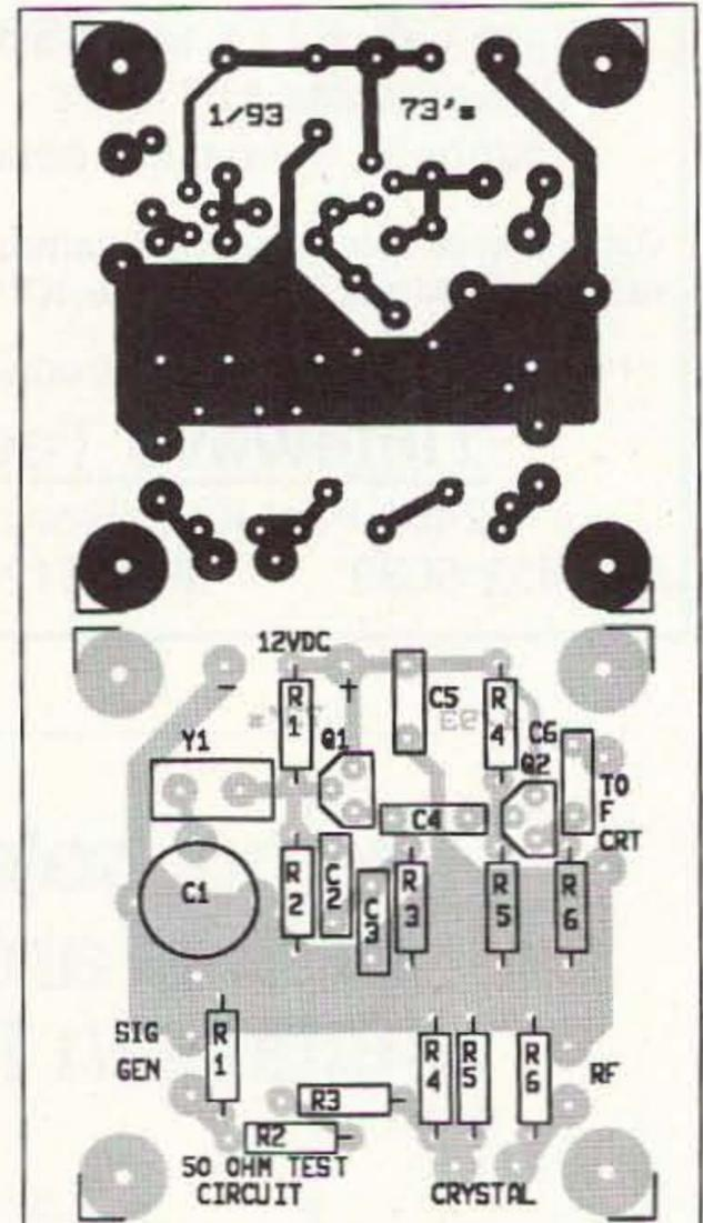
Figure 10. (a). PC board foil pattern for the oscillator circuit. (b). Parts placement. Note that the 50-ohm test circuit shown in Figure 3 is incorporated on this board.
