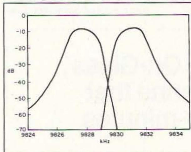
Figure 8. Calculated passbands with series resistance included.
