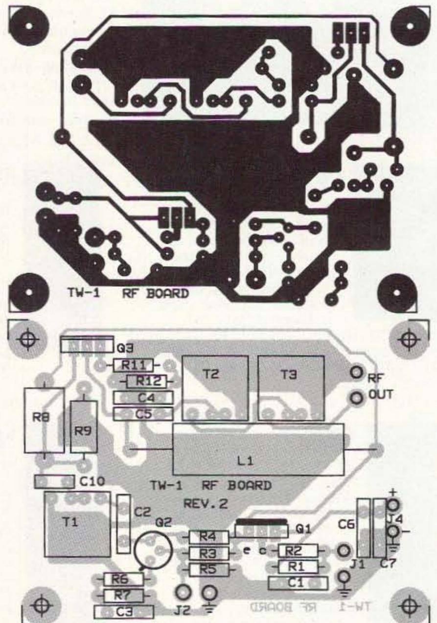
Figure 2 (a). PC board foil pattern of the power amplifier board. (b). Parts placement.
