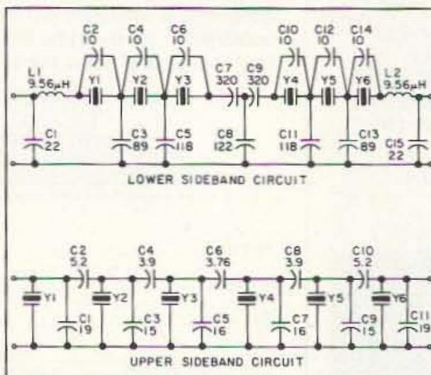
Figure 2. Filter schematics. All capacitors in pF.
