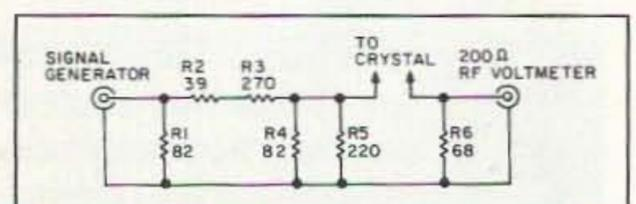
Figure 3. 50-ohm test circuit.
