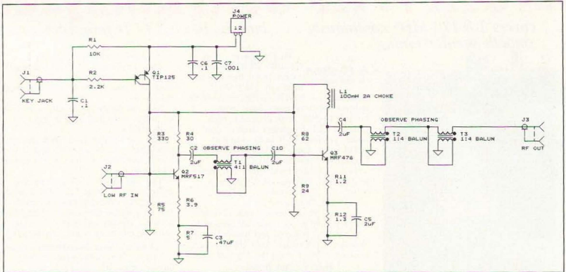
Figure 1. Schematic diagram of the power amplifier board.
