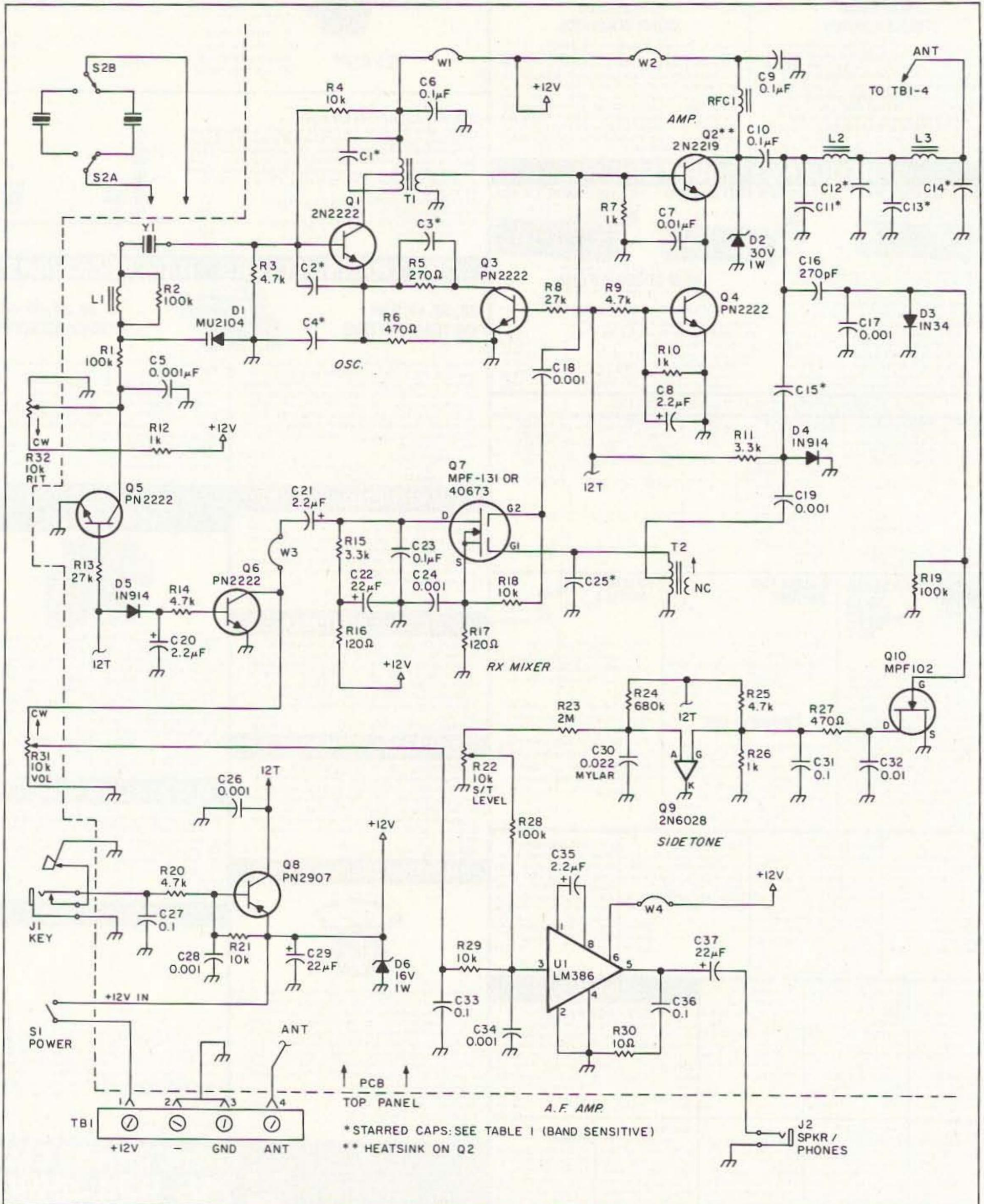
Figure 1. Schematic diagram of the SP-1 transceiver.
