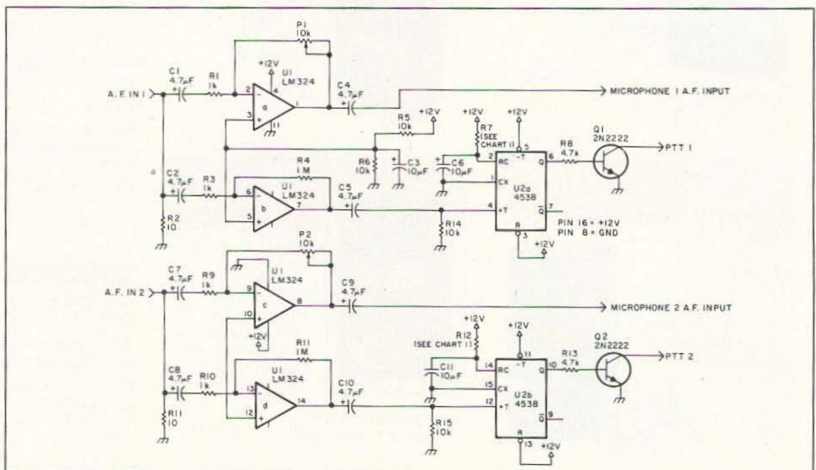
Figure 1. Tape deck to beacon transmitter interface circuit.
