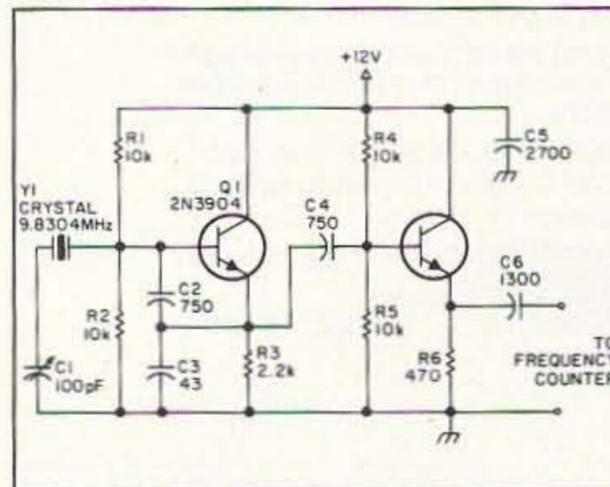
Figure 9. Oscillator circuit for use as a BFO or transmitter carrier.
