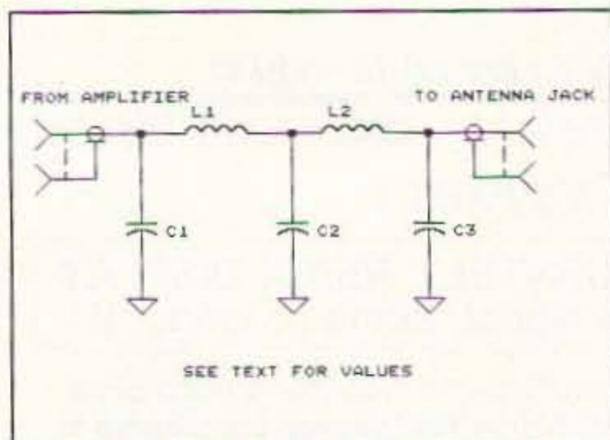
Figure 3. Schematic diagram of the optional output filter board.
