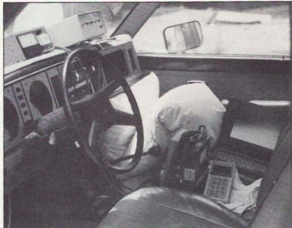
Photo C. WB8WFK's car is ready for the hunt. The analog fox-box and digital interface unit are on the dash. The computer (protected by pillows) has replaced a human in the passenger's seat. (Photo by WB8WFK.)
