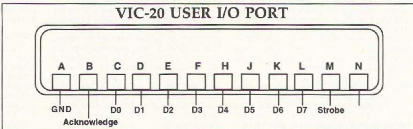
Figure 1. Corrected diagram (see last month's column) showing the Commodore VIC-20 user I/O port.
