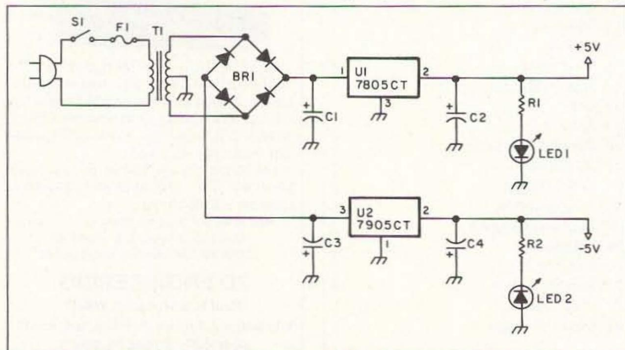
Figure 4. Schematic diagram of the +/- 5 volt power supply.
