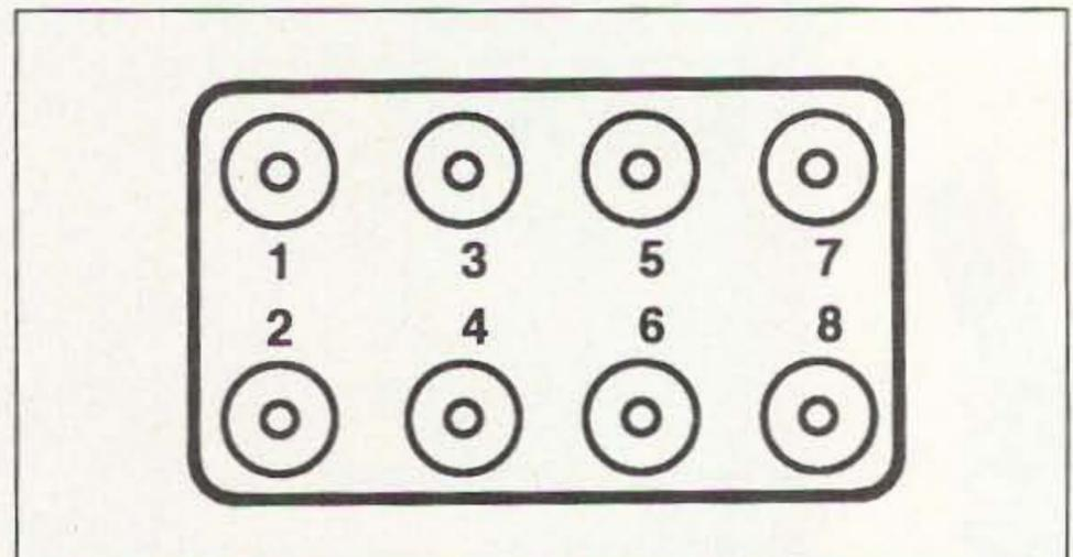
Figure 2. Pinouts for the Mini-Circuits SRA-series.
