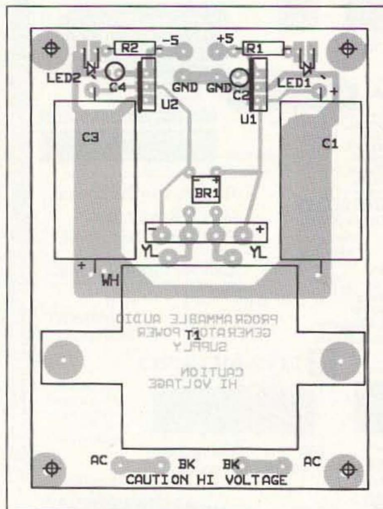
Figure 8. Parts placement for the power supply.
