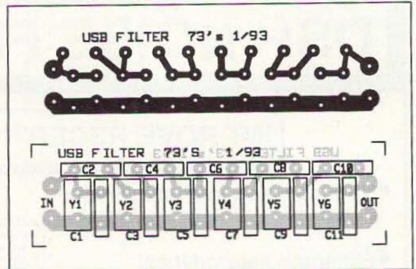
Figure 5. (a). PC board foil pattern for the upper sideband filter. (b). Parts placement diagram.
