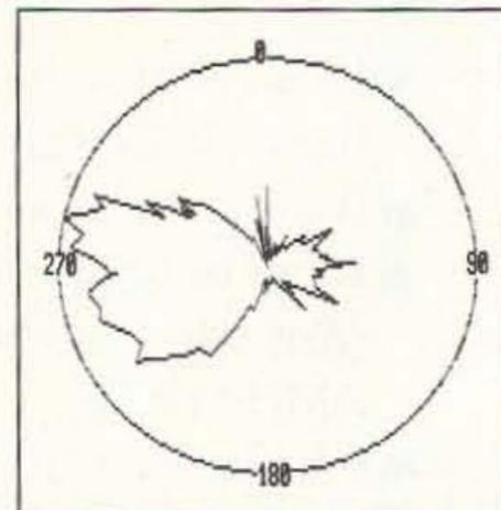
Figure 5. This plot was taken in a supermarket parking lot on an Albuquerque T-hunt. The spikes at zero degrees represent noise from power lines ahead of the vehicle. The hidden T is to the left and there is reflected signal from the right.
