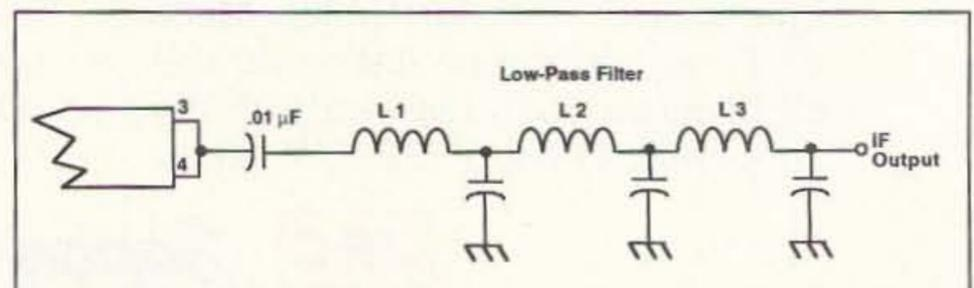
Figure 4. Low-pass filter output circuit.
