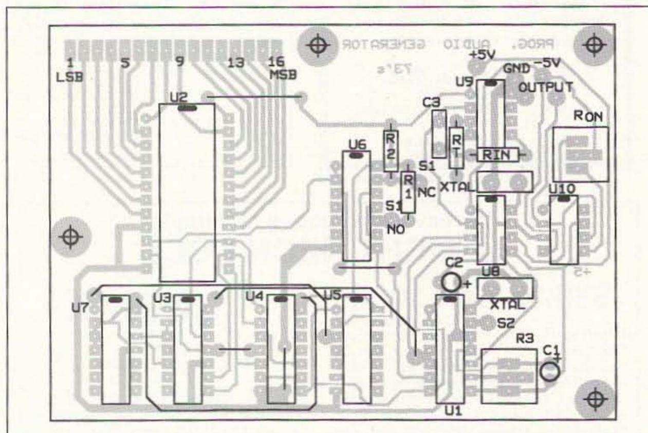
Figure 6. Parts placement for the Audio Generator.
