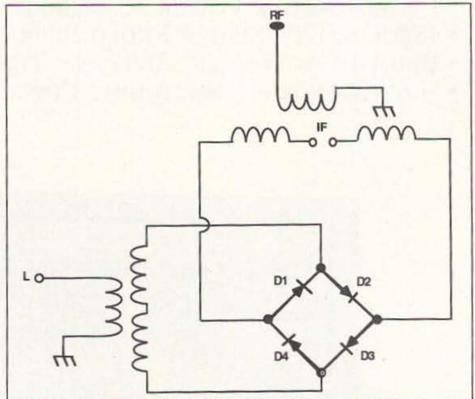
Figure 1. Circuit for a double-balanced mixer.
