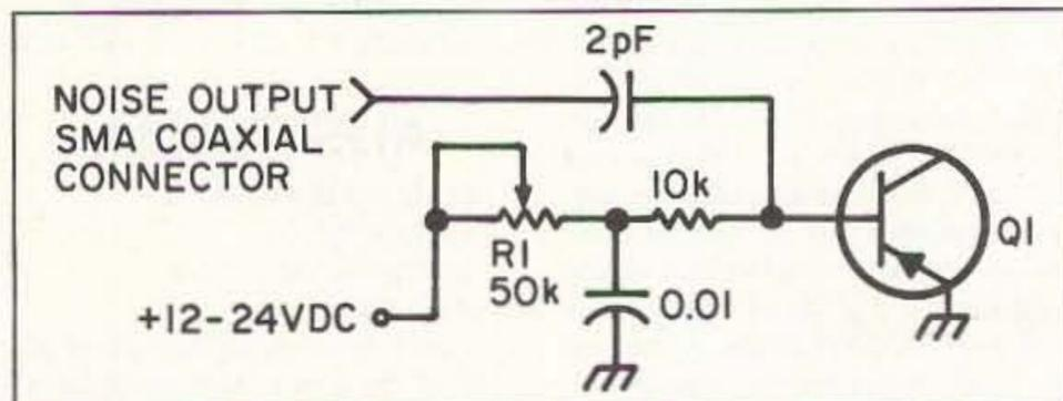
Figure 1. Noise head construction: transistor AT-42085 or any NPN device with high Ft. Set R1 for 1-2 mA current through the Q1 base emitter.
