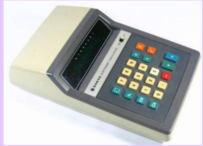
Some of these early calculators resembled portable transistor radios of the time – in particular because of the carry handle at the top which could be pushed back into the case or folded out to prop the calculator up at one angle. All had General Instruments' circuits within.
