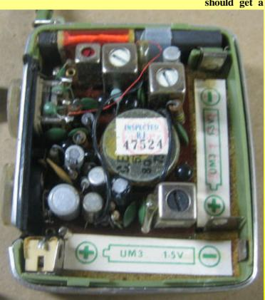
Use superglue if the break is clean and somewhere near the middle. There will be a slight reduction in performance with this sort of repair, but not enough to worry about. If the rod is broken into several pieces it should be replaced. The fine wires from the coils on the ferrite rod aerial can become broken, and the break is not always visible. If in doubt, check with multimeter.
