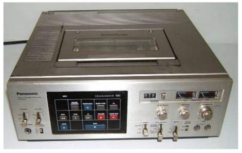
pre-programming of a recording event up to 24 hours in the future, required the pressing of the 'stop' button' before pressing either the fast-forward or rewind buttons, and made the screen go black when the pause button was pressed. The outside was usually silver or wood grain effect.
