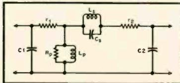
Fig. 1. Equivalent circuit of audio transformer.
