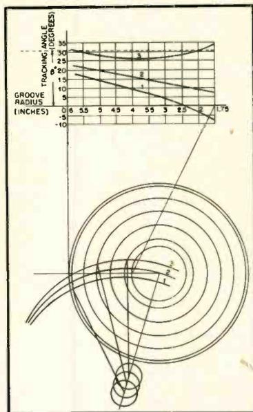
Fig. 4. Tracking angle variation of the same arm at different pivot mountings.<sup>3</sup>
