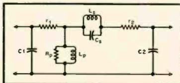
Fig. 1. Equivalent circuit of audio transformer.
