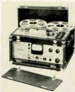
for either half-track or full-track recording, the 400-A can be operated at either 7½ or 15 ins./sec. as controlled by a speed selector switch. The Model 400-A differs from the earlier Model 400, which it surpasses, in the fact that all mechanical motions are operated by solenoids under push-button control. Starting interval is
