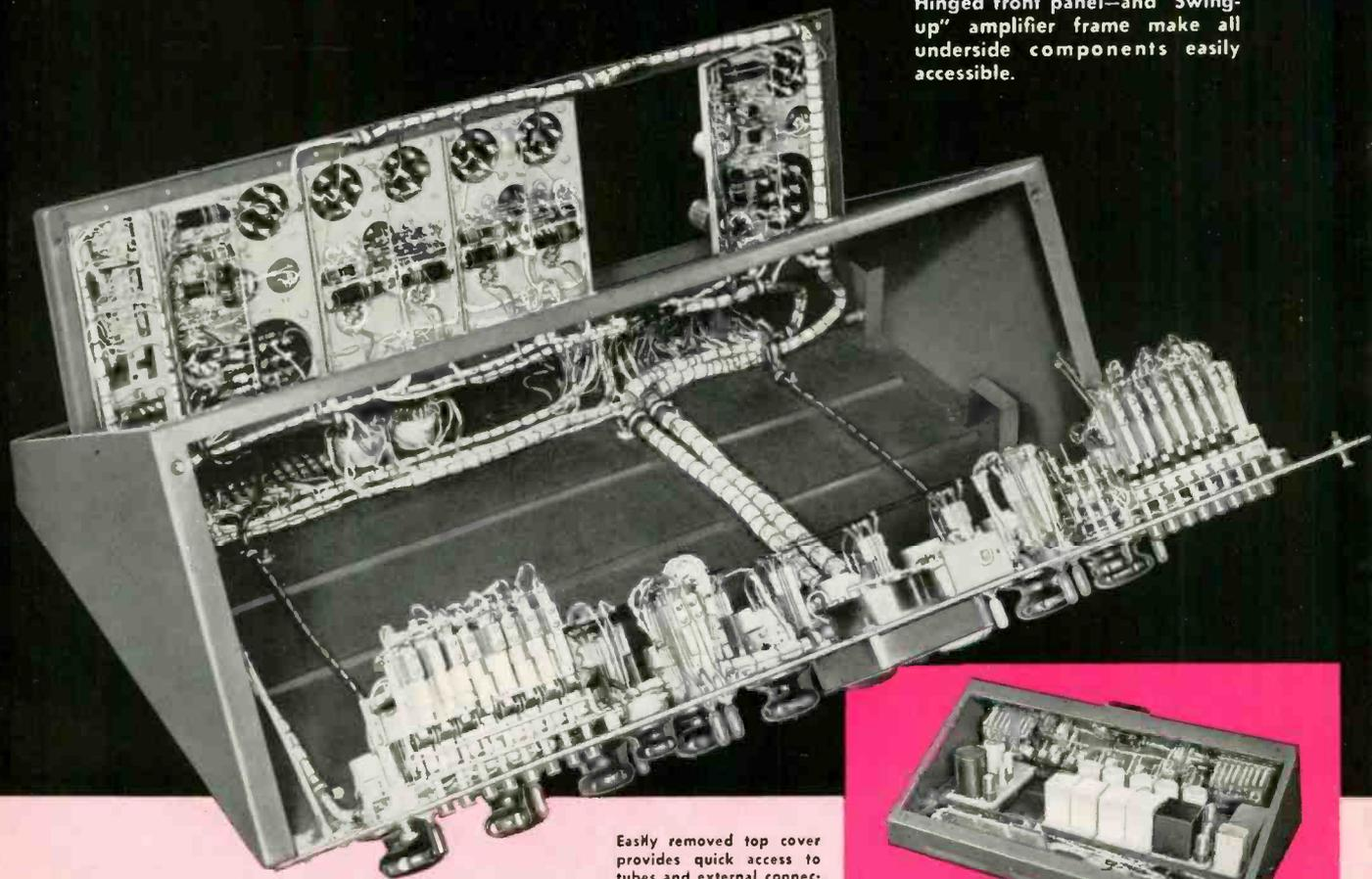
Hinged front panel—and "Swing-up" amplifier frame make all underside components easily accessible.
