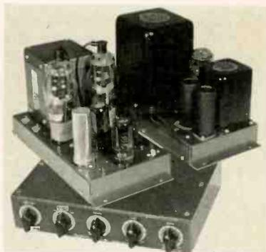
fier is flat within one db from 10 cps to 100 kc. Harmonic distortion is less than 0.5 per cent between 20 and 20,000 cps at five watt output. Intermodulation at five watts is 0.5 per cent using 60 and 3000 cps. The Heath Company, Benton Harbor 25, Mich.
