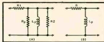
Fig. 2. Equivalent circuit for low-frequency cut-off, in a direct-coupled a.f. transformer. (A) Complete arrangement:  $R_1$  = primary source impedance;  $R_2$  = secondary load impedance. (B) Simplified equivalent of (A):  $R$  = parallel combination of  $R_1$ ,  $R_p$ , and  $R_2$ .
