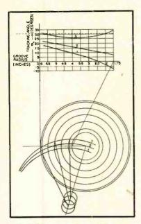
Fig. 4. Tracking angle variation of the same arm at different pivot mountings.<sup>3</sup>
