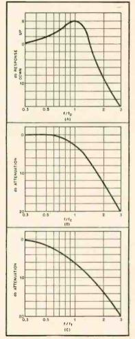
Fig. 10. Attenuation responses for high-frequency cut-off; (A) less-than-critical damping; (B) critical damping; and (C) more-thancritical damping.
