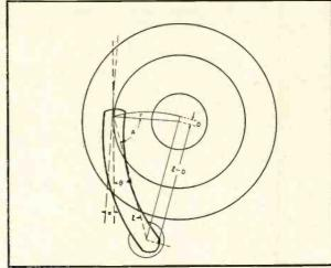
As would be expected from the tracking curves of Fig. 4 optimum mounting of the straight arm requires that the needle be underhung by an amount which places the point of perfect tracking at the inner grooves.
