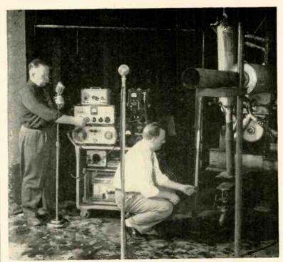
TESTING OF MUFFLERS at the Donaldson Co., St. Paul, Minn., is simplified with recording equipment tailored to the job by Donaldson engineers. Comparative performances recorded on tape can be played over and over again for analysis.
