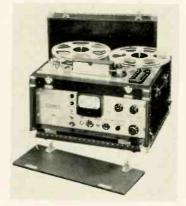
for either half-track or full-track recording, the 400-A can be operated at either 7½ or 15 ins./sec. as controlled by a speed selector switch. The Model 400-A differs from the earlier Model 400, which it supercedes, in the fact that all mechanical motions are operated by solenoids under push-button control. Starting interval is
