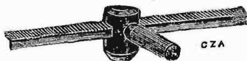
FIG. 17.—Slider fitted to Rack. By turning the knurled projection a smooth movement is assured.
