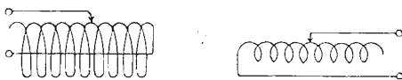
FIG. 44.—Coils of Aerial and Detector Circuit of a Loose-coupler, both tuned with Sliders.
