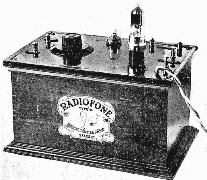
FIG. 70.—Variometer Tuned Receiver, with enclosed Crystal Detector and built in Single-valve Magnifier. Such a receiver will give far stronger signals than can be obtained with the best crystal alone.
