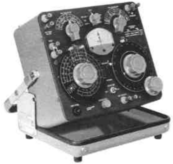
Two popular GR impedance bridges: the modern Type 1650-A and its predecessor, the Type 6.50-A of 1934.
