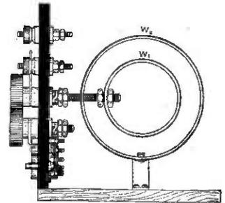
Fig. 11. Showing the construction of a tuner. The fixed coil  $W_2$  has two sets of tappings for rough and fine tuning respectively. The rotor  $W_1$  is connected in the secondary circuit.
