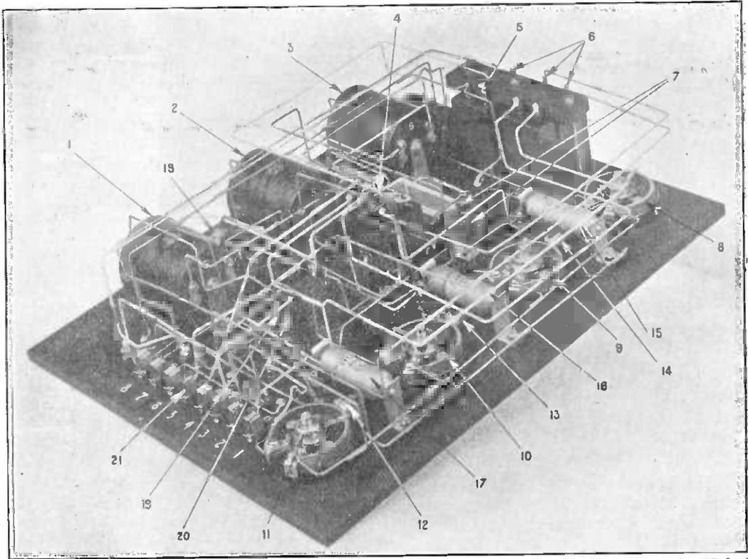
*General view: 1, 2 and 3. Transformers. 4. Switch. 5. H.T. Condenser. 6. Loud speaker and grid feed condenser. 7. Grid cells. 8, 9, 10 and 11. Filament resistances. 12 and 13. Grid leaks of L.F. valves. 14. Grid leak of detector valve. 15, 16 and 17. Anode resistances. 18. Transformer secondary shunt resistance. 19. Transformer primary condenser. 20. Grid condenser. 21. Connector clips.*
