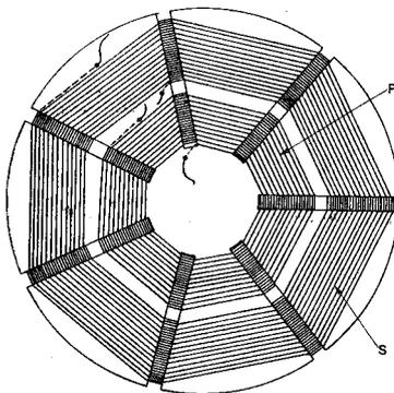
Fig. 21. A useful high-frequency transformer.
