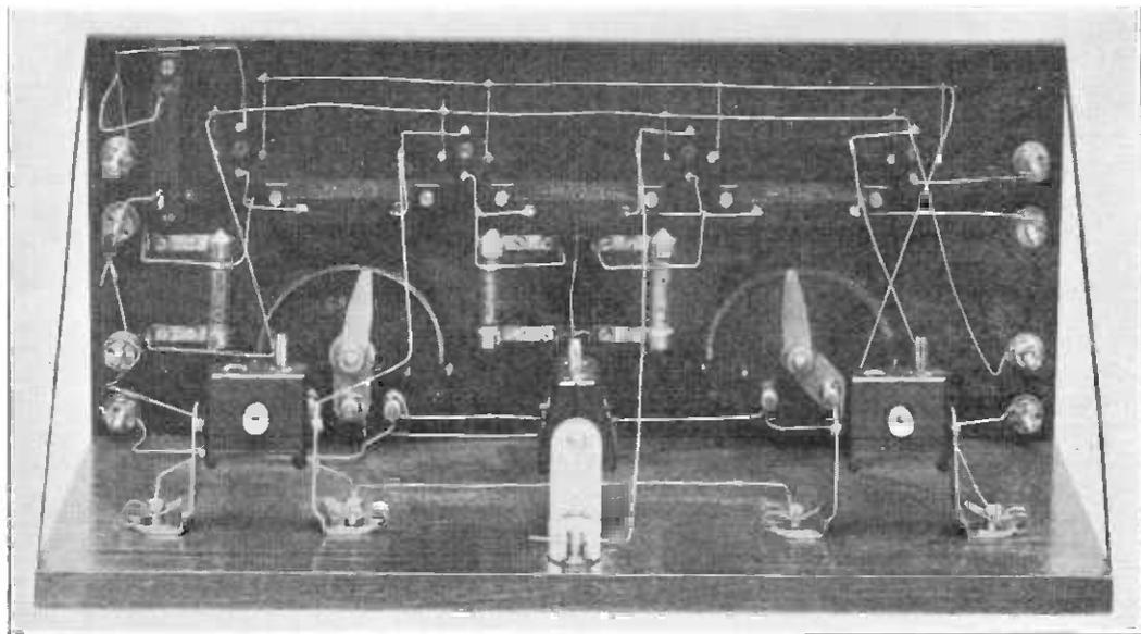
*Fig. 1. Four valve long wave amplifier with three high frequency circuits and detector.*
