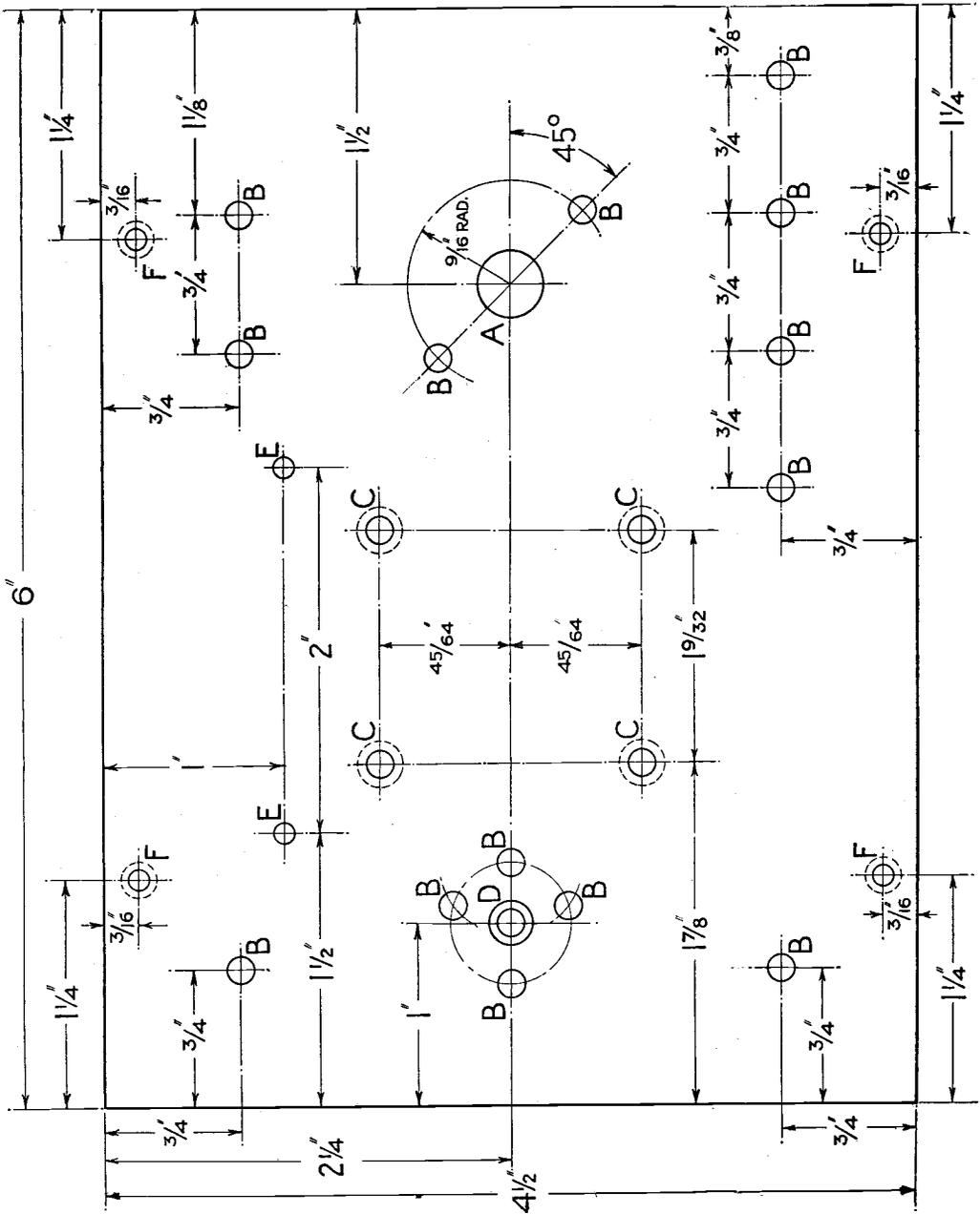
The location of the holes on the ebonite panels, and for the purpose it will be sufficiently accurate if the centres are pricked through on the panel. Size of holes: A, 3/8 in., B, 5/32 in., C, 5/32 in. and countersunk on top side. D, 5/32 and countersunk on underside; E, 1/8 in. blind holes 3/16 in. deep; F, 1/8 in. and countersunk on the top side for No. 4 wood screws.
