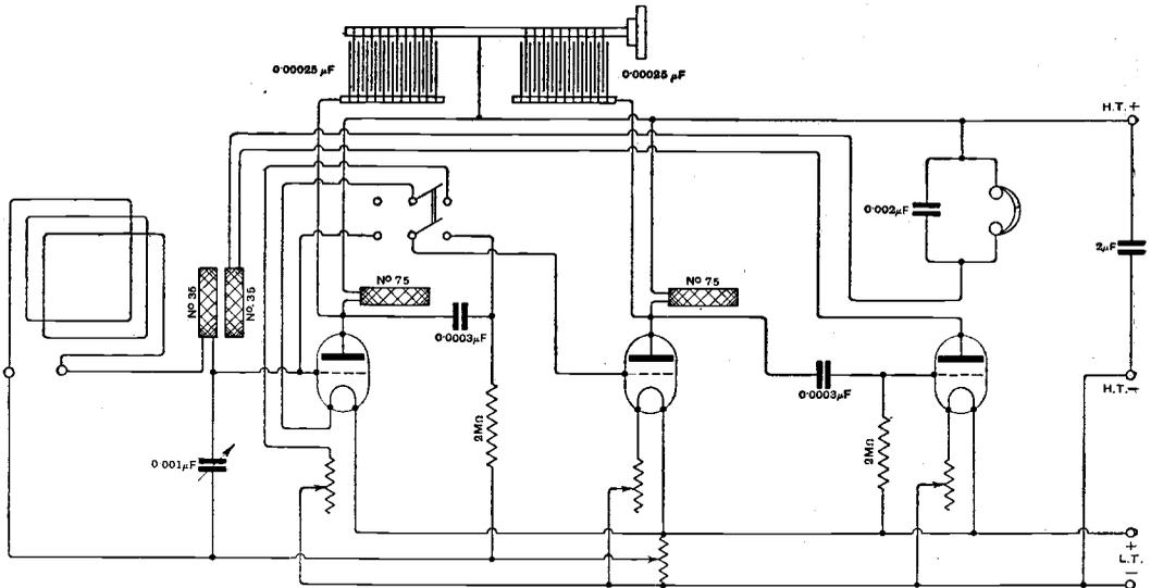
Fig. 1. "NITON" (Boscombe). Three-valve receiver (two H.F. and det.), with switch to cut out one stage of H.F., and employing a coupled variable condenser for tuning the H.F. circuits.
