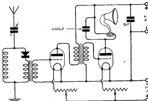
Fig. 1. "R.A.J." (Torquay). A crystal receiver with two note magnifiers.
