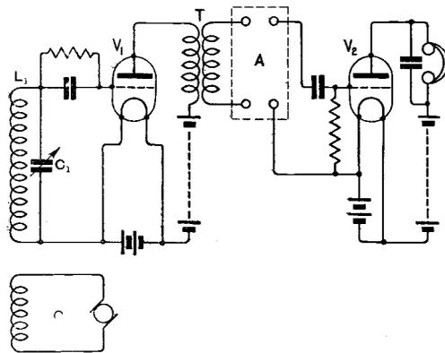
Fig. 1. Circuit principle of the Supersonic Heterodyne Receiver.
