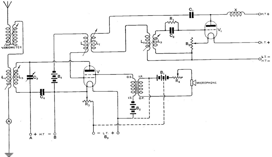
Fig. 5. Circuit of the complete transmitter.
