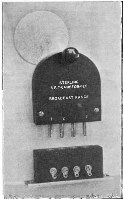
Fig. 24. A plug-in transformer with mounting. The inductance of the coils, and therefore their natural frequency, is varied by changing the position of the metal plate.
