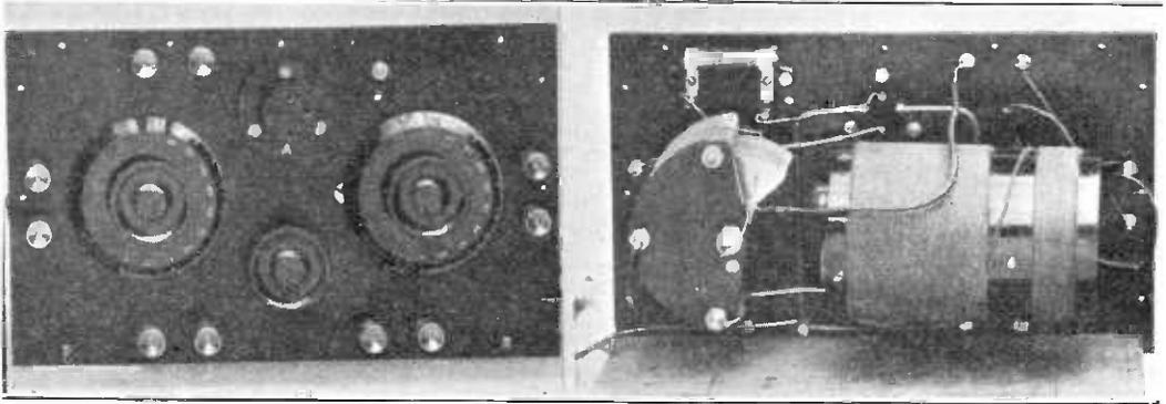
Fig. 1. Front and rear view of the rectifier unit.
