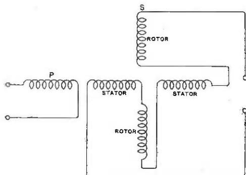
Fig. 20. Connections of another sort of vario-transformer.
