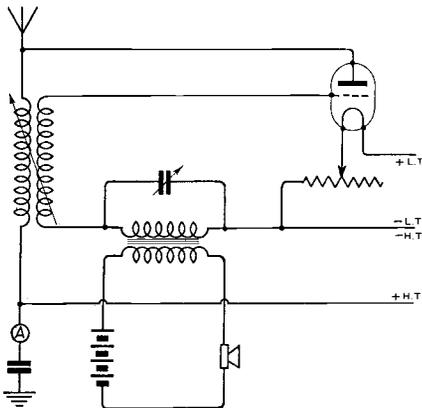
Fig. 1. A grid control valve transmitter.
