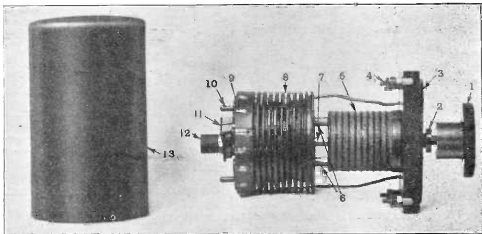
Fig. 14. A tapped reactance unit with a coupling coil for providing reaction effects. (Lissen, Ltd.)
