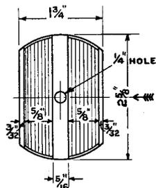
Fig. 3. Reaction coil.
