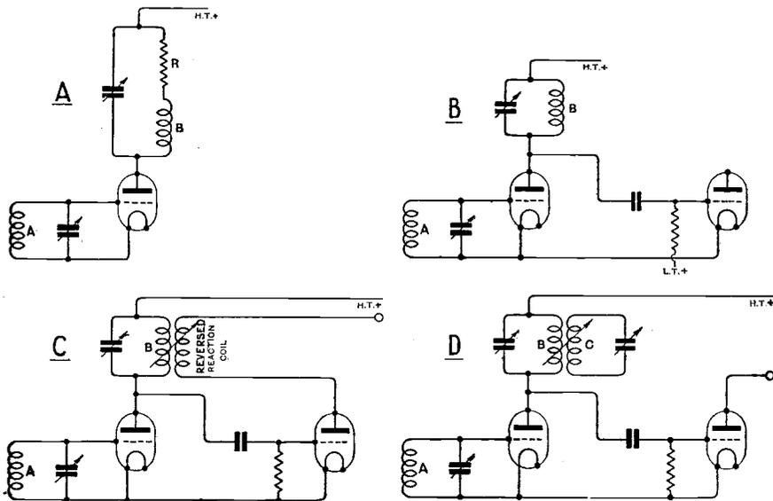
Fig. 2. Four methods for reducing the tendency of sharply tuned circuits connected with valves generating oscillations.
