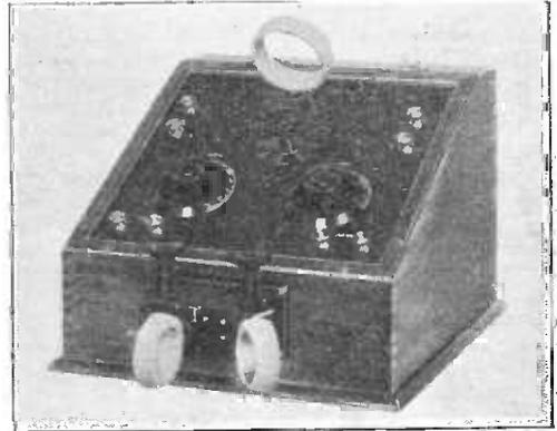
*The constructor's two-valve receiver assembled.
