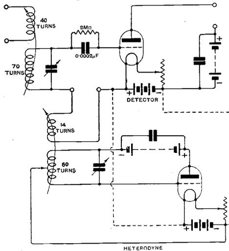
Fig 2. Detecting and oscillator circuits for frequency changing.
