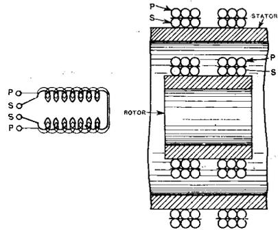
Fig. 28. A vario-transformer, consisting of a variometer with two sets of windings.
