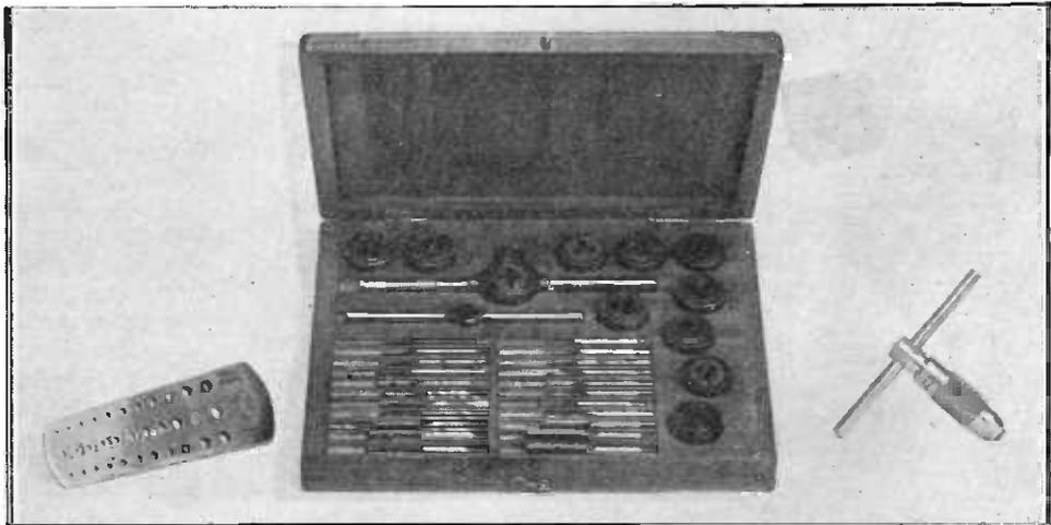
Fig. 2. BA. Tapping gauge, set of BA. stocks and dies, and tee tap holder.
