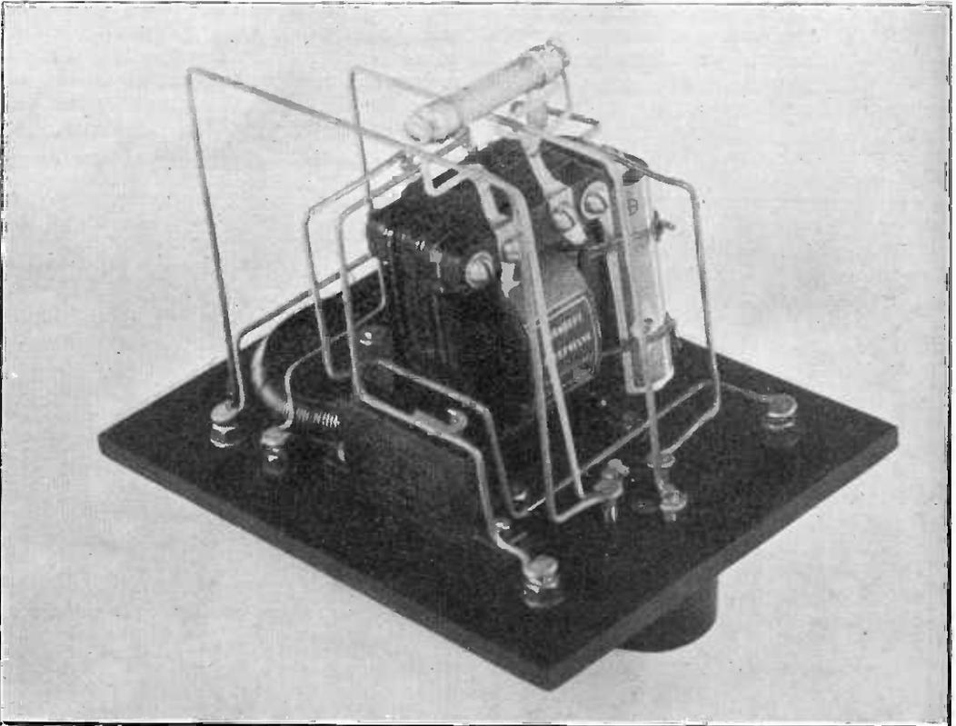
*View of the underside. The method of wiring is clearly shown. The tinned ends of the high resistance (grid-leak type) can be easily soldered to loops to avoid the fixing of brackets on to the panel, but care must be taken not to overheat the resistance.*
