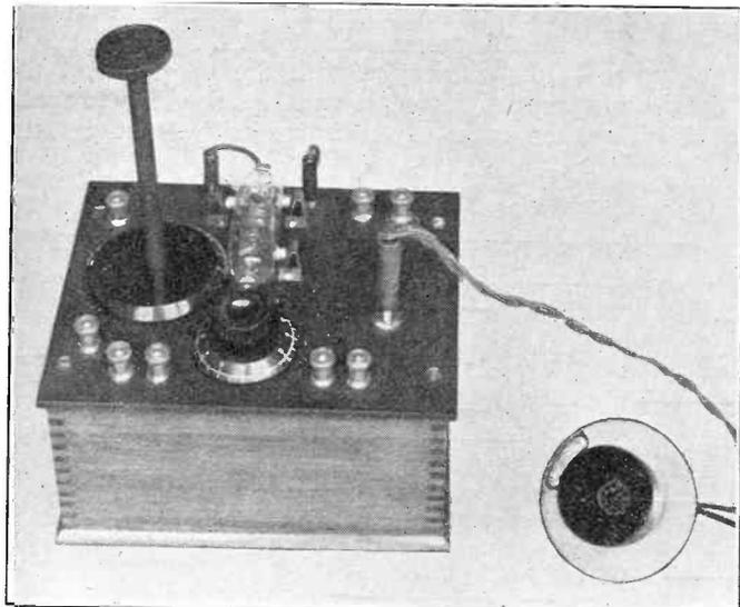
Fig. 3. Complete modulating unit for attachment to existing valve oscillator.
