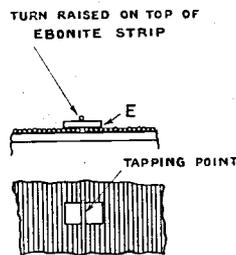
Fig. 2. Method of making tappings.
