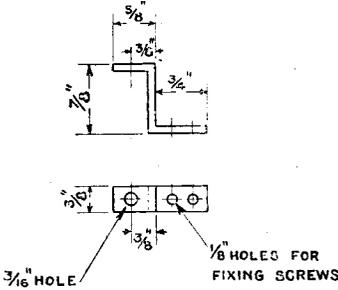
Fig. 5. Bracket for tuning coil.
