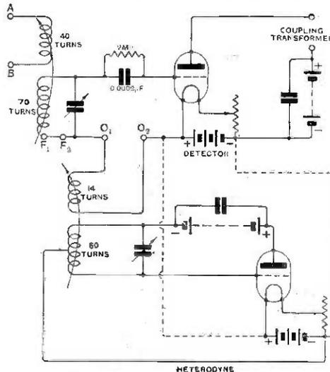
Fig. 2. Circuit connections of the oscillator and detector units.
