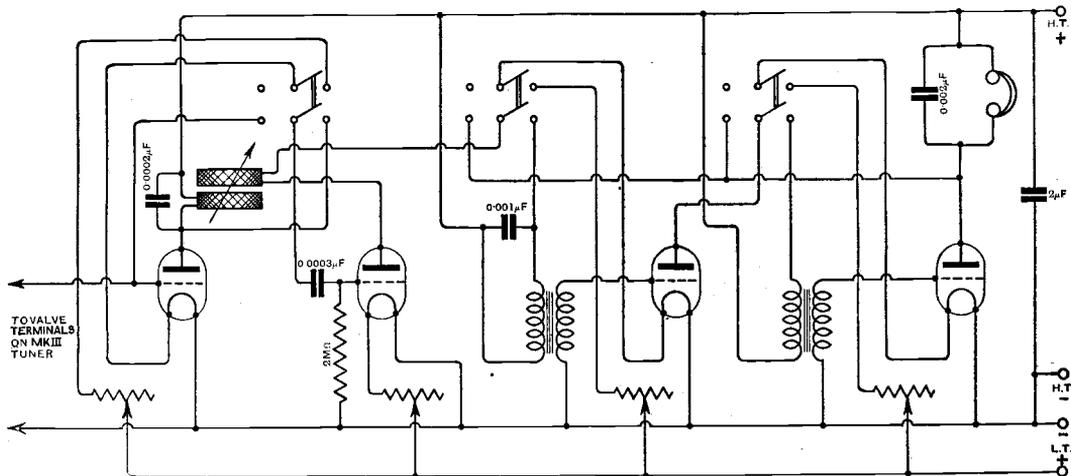
Fig. 2. "E.B." (Leeds). The first valve operates as a high-frequency amplifier, the second as rectifier, and the last two as note magnifiers. The switches are connected so that the number of valves in circuit may be easily varied.
