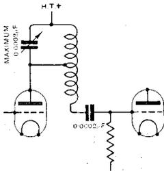
Fig. 1. Simple method for obtaining a potential step-up in a H.F. circuit.
