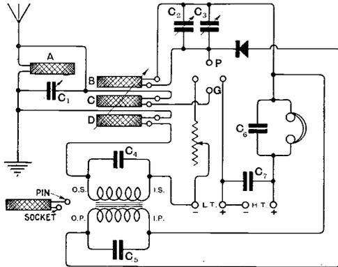
Fig. 2. Simplified practical wiring diagram. The references B,C should be read as C,B to correspond with Fig 1.
