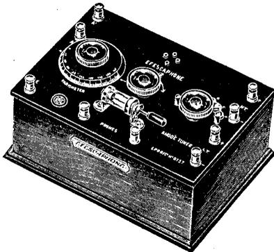
*The Efescaphone crystal and valve set, making use of dual amplification.*
