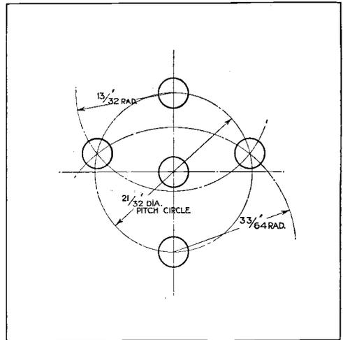
An enlarged drawing giving the exact setting out of the positions of the valve pins.
