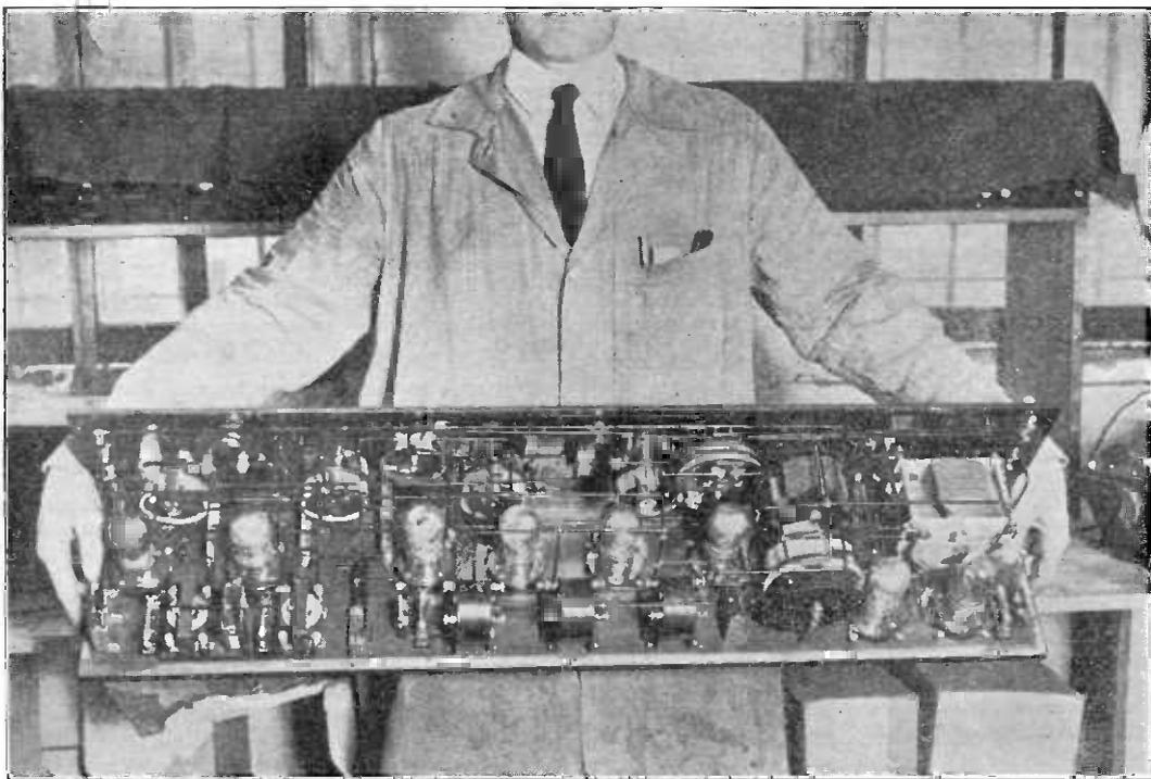
The photograph shows the interior of a well-built eight-valve super-heterodyne receiver. The first valve is the detector, the next the oscillator, then follow three H.F. stages, detector, and two note magnifiers.
