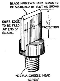
Construction of a connector.
