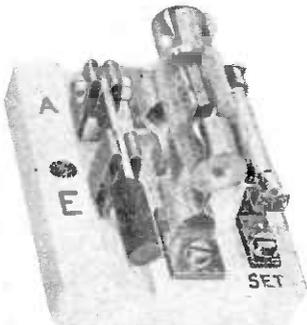
*Aerial protection device of Messrs. Siemens.*
