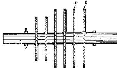
Fig. 22. When a number of basket coils are employed in a transformer, they should be spaced to reduce self-capacity.
