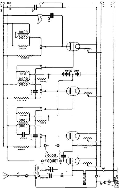
Circuit in which L.F. amplification can be obtained either with resistances or transformers.
