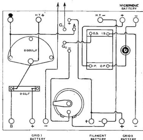
Fig. 4. Practical wiring on underside of the modulating panel.
