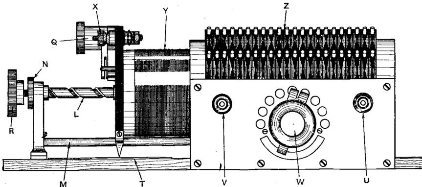
Fig. 8. Another type of long wavelength loose coupler with multilayer windings. The primary winding is Z, which is tapped by switch W, and connection is made with terminals V, U. The secondary winding is Y, which is tapped by switch Q; the connecting terminals are X. The secondary coil is moved by turning knob R and rod L. N is a lock nut, and slides along bars M. The pointer moves over the scale T.
