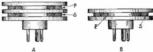
Fig. 23. Two well-known types of plug-in high-frequency transformers.
