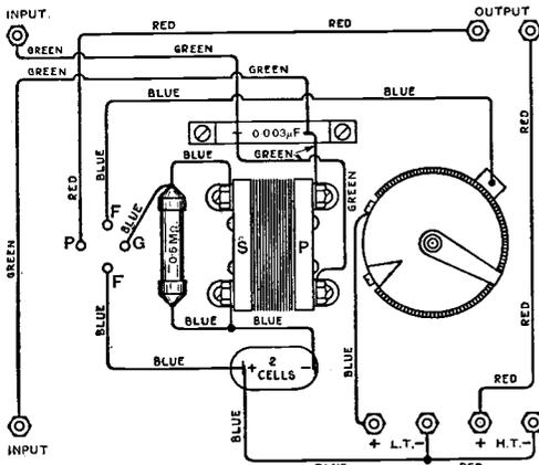
*Practical wiring diagram showing the actual points between which leads are connected. If the leads are enamelled in various colours, the tracing of the circuit is simplified.*
