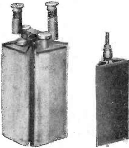
*Compressed plates of Fuller block secondary cell.*
