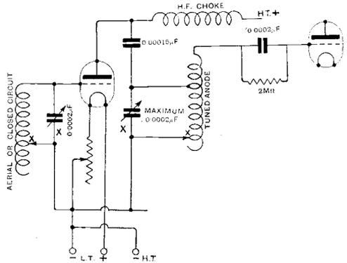
Fig. 2. An interesting H.F. amplifying arrangement. By reason of the small condenser in the plate lead it is possible to secure a higher potential across the anode coil than is normally possible. The H.F. feed choke must be well designed and of low self capacity to avoid excessive leakage.
