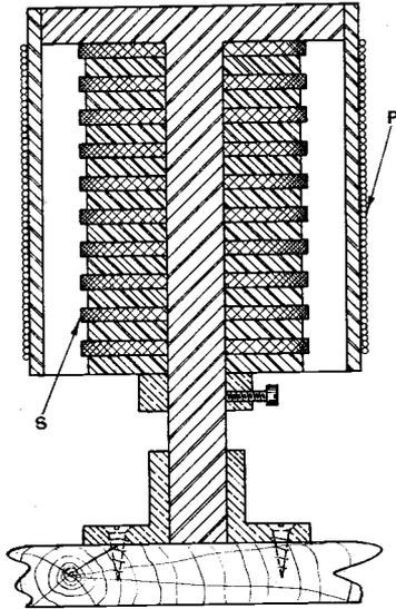
Fig. 27. A transformer with one winding in the form of a cylindrical coil, and the other consisting of a number of basket coils.
