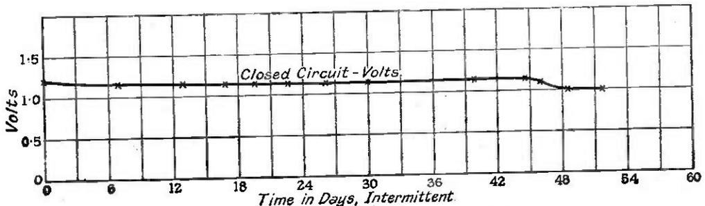
Fig. 1. Curve showing average voltage during discharge.
