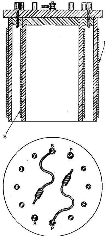
Fig. 26. A tapped transformer with the windings wound on tubes of different diameters.
