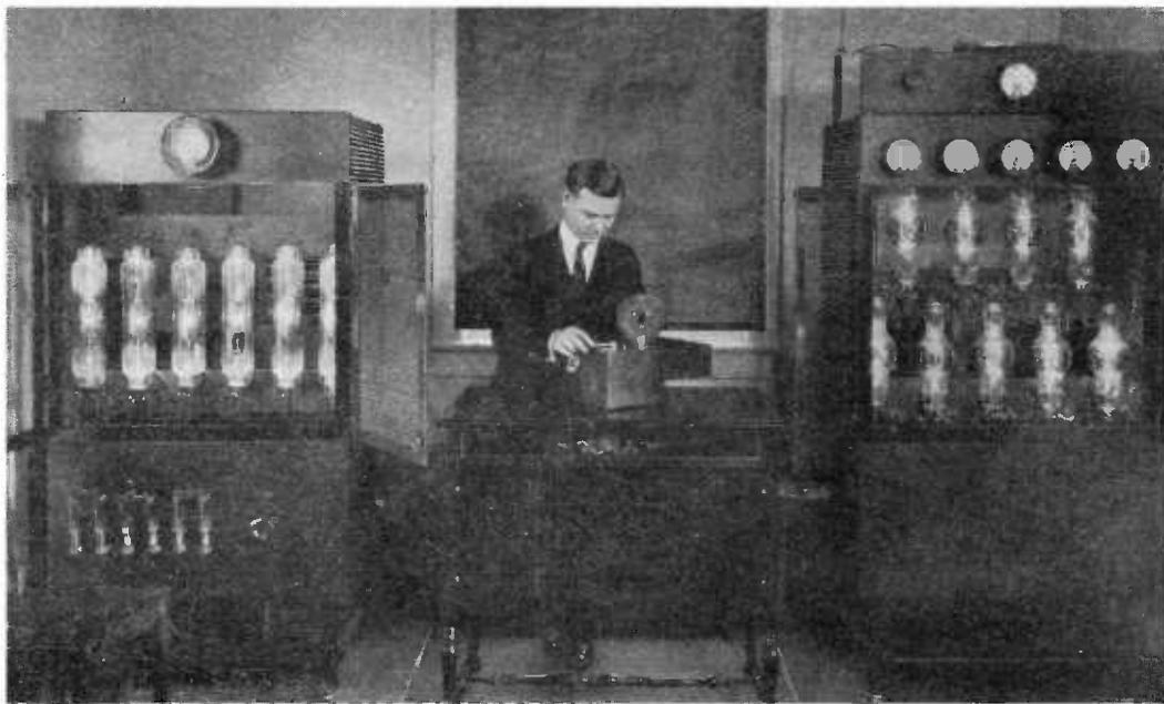
A corner of the transmitting room of station WJZ. The power panel is shown at the left. The six rectifier valves supply the 2,200 volts of direct current for the modulator and oscillator valves of the transmitter panel to the right. Five 250-watt modulator, and 4 oscillator valves of same rating are used in the transmitting circuit. The operator is shown checking the wavelength, which is 360 metres.
