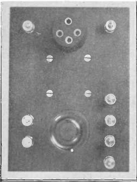
View of the top of the panel. The terminals can be identified by carefully enamelled lettering, or the panel can be put out for engraving before assembling.
