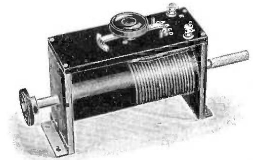
Fig. 18. A coupling unit, suitable for low-power, short-wavelength transmitters. (H. W. Sullivan, Ltd.)
