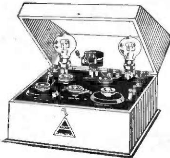
*Two-valve receiver by Messrs Radiax, Ltd.*
