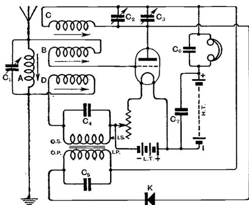
Fig. 1. Theoretical diagram of the dual amplification circuit described.
