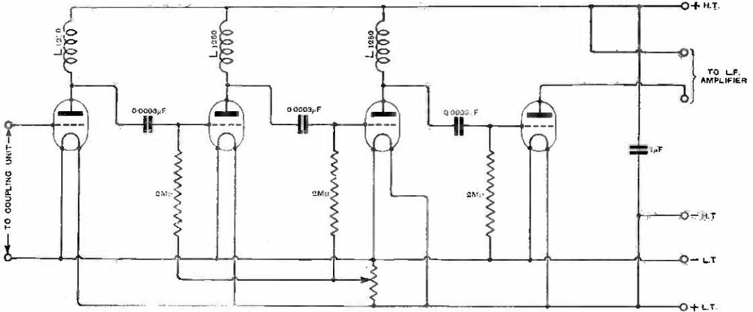
Fig. 2. Circuit of H.F. amplifier for use after the frequency change is effected by the detector and oscillator.
