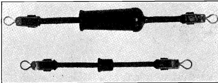
They are constructed of rubber and cotton, with end clips of duralumin. The cup in
