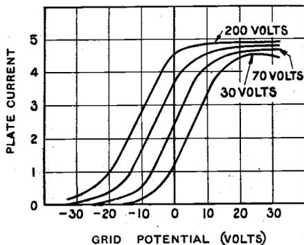
Fig. 1. A "family" of characteristic curves for various plate voltages and constant filament current.
