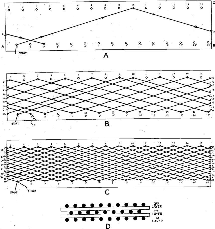
Fig. 4. Method of winding a duolateral coil. A shows a single turn. Notice the end 1 lies two pegs ahead of the commencement of the turn. B gives the appearance of a complete layer plus one turn of the second, and C shows two complete layers. Notice the beginning of the second layer lies over the spaces of the first, while the third layer lies directly over the first. D is a section which shows the position of the wires in the coil.
