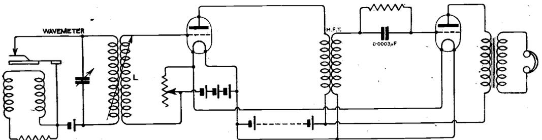
Fig. 1. The wavemeter on the left induces oscillations of the desired wavelength into the inductance "L" and high frequency amplifying circuit, affording a simple method for testing the efficiency of the H.F. transformer.
