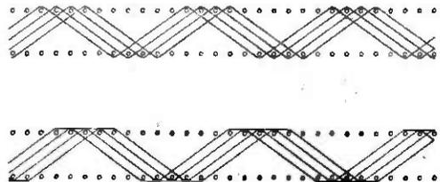
The upper figure shows the usual method of winding, while the lower figure is a suggested improvement for producing flat sides.
