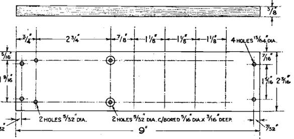
Details of the wooden panel on which the resistances and condensers are mounted.
