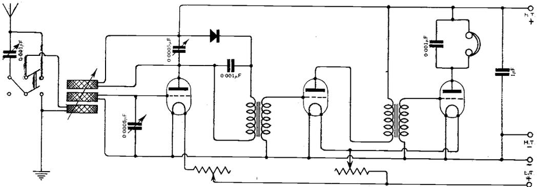
Fig. 2. **"J.N.S." (Sheffield)**. A simple receiver arranged as follows: H.F. amplifier, crystal rectifier, and two note magnifiers.
