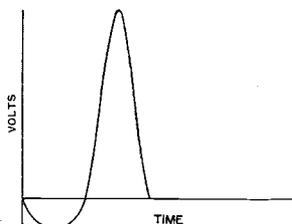
Voltage curve of T.V.T. secondary.
