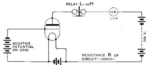
Fig. 2. When a negative potential is applied to the grid, the circuit resistance is high, and the time constant lower.
