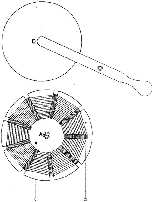
Fig. 16. A very simple method of varying the inductance of coil A is to arrange a metal plate B, so that its position with respect to the coil may be varied.
