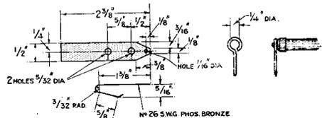
Dimensions of connector springs. The method of making connection to the grid leaks is also shown, and care must be taken not to overheat the leaks as they are wax filled.
