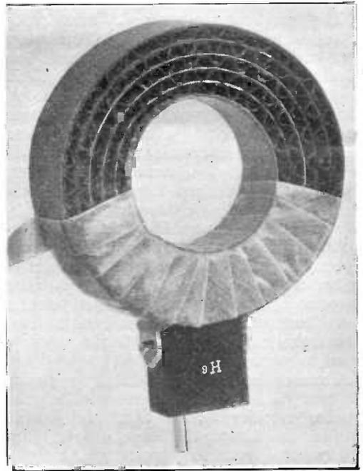
Fig. 2. This is another form of plug-in coil. The layers are spaced with corrugated separators.
