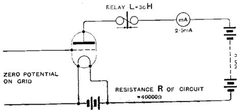
Fig. 1. The relay is shown here connected in the anode circuit of the last valve.
