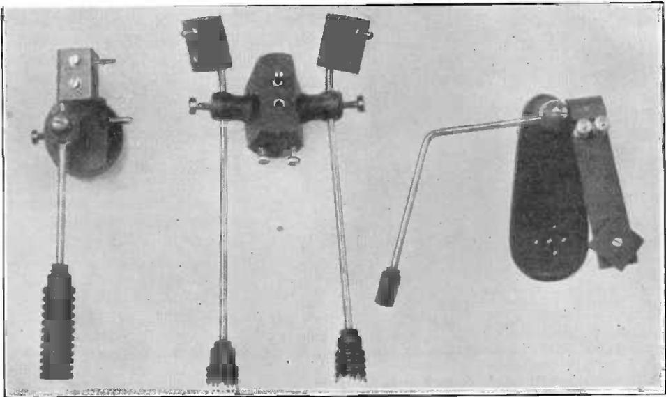
place of a single aerial circuit plug-in coil, for reacting on to the tuned anode or H.F. transformer
