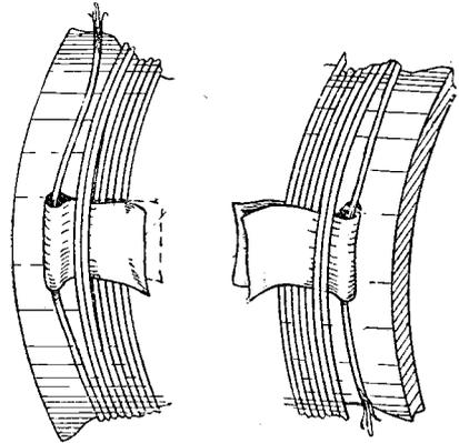
Method of securing the ends of the winding by means of tapes.
