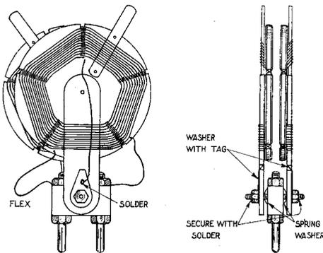
coils are held by the spring washers and nuts shown in the figure.
