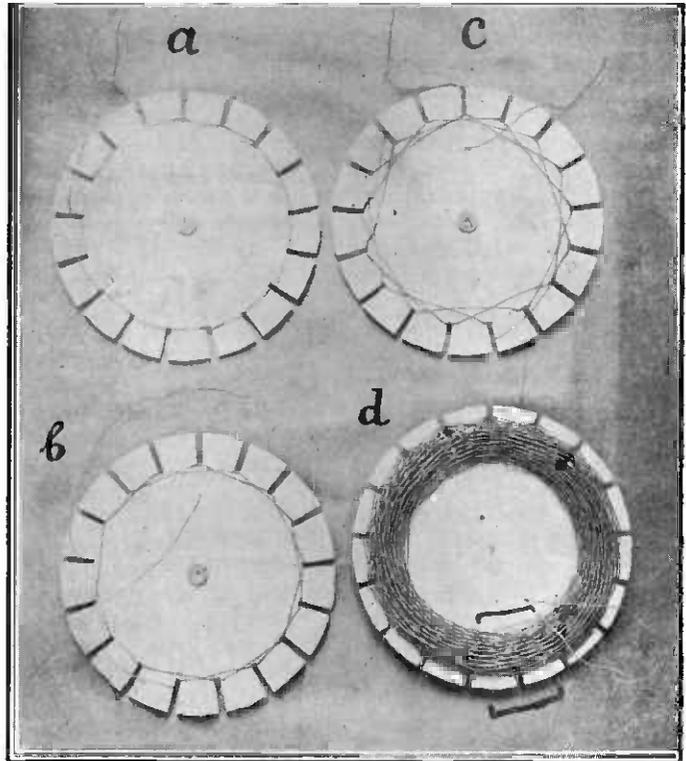
Fig. 3. Basket coils wound with different pitches, a having the pitch  $(1 + 1)$ , b —  $(2 + 2)$ , c —  $(3 + 3)$ , d —  $(4 + 4)$ .
