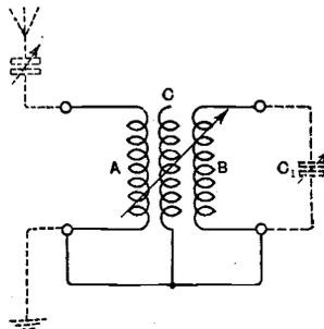
Fig. 2B. The third winding C, which is wound as shown in Fig. 2A, is connected on one side with coil B and earth.
