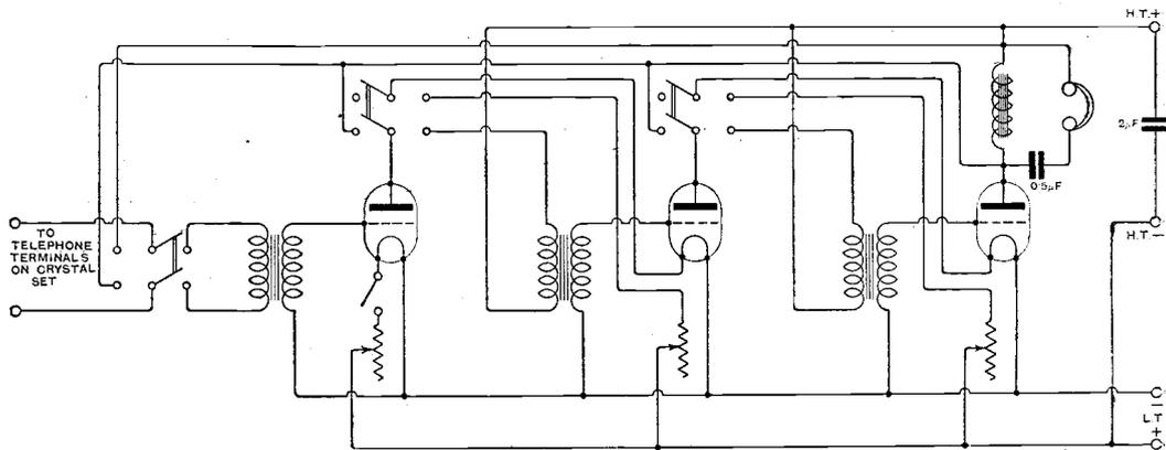
Fig. 3. “A.F.B.” (Crumpsall). A three-valve note magnifier suitable for connecting to a crystal receiver.
