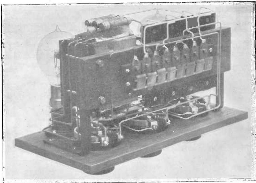
*Another view showing the mounting of the components. A special feature in the design is that connection is picked up with the stems of the terminals by means of a strip of contact springs, permitting of the withdrawal of the instrument from the case without the entanglement of flexible leads, and at the same time disconnecting battery and other leads.*
