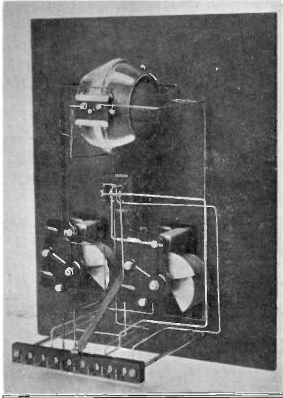
Back view of the tuning panel. The specially shaped condensers and vernier adjustments can be seen. The strip of contacts carries the connection to the back panel.
