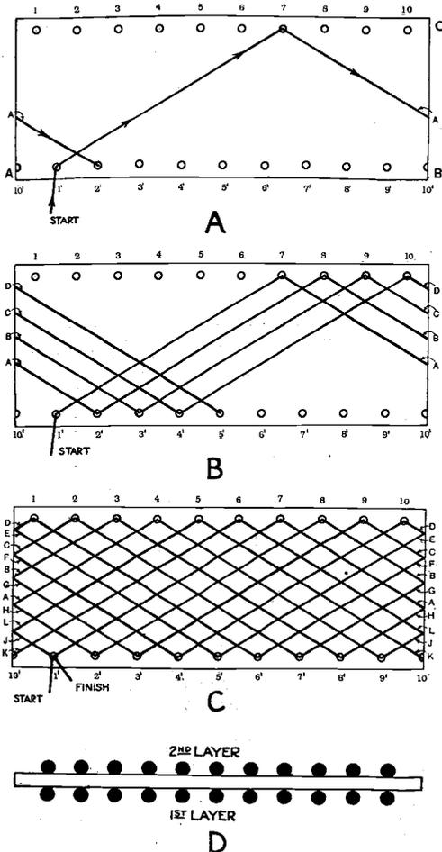
Fig. 3. Method of winding a simple honeycomb coil. A shows a single turn; B several turns; and C a complete layer. Follow out the winding with the aid of the figures and letters to learn the formation. D is a section, showing two layers. The turns in adjacent layers lie above each other, but separated by the wire thickness.
