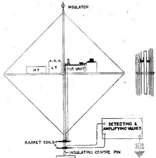
the signals to the detecting circuit is through coupled inductances concentrically arranged about the spindle of the frame, thus avoiding flexible leads or rubbing contacts. J. F. S.
