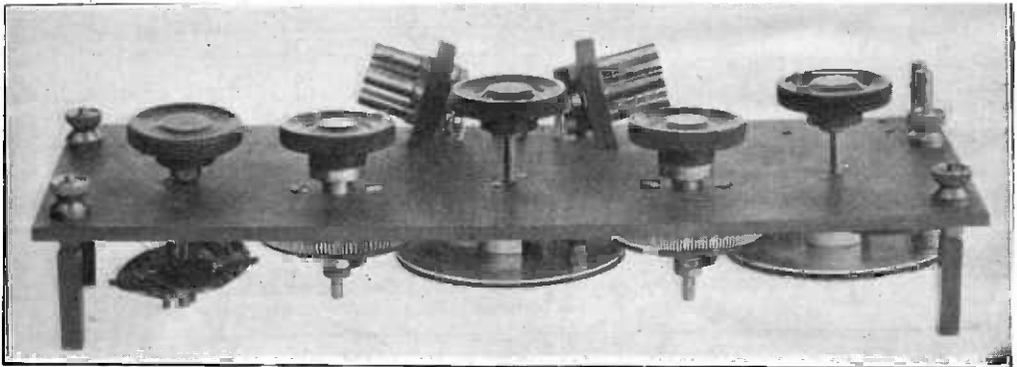
*Complete two-valve receiver of particularly simple construction.*
