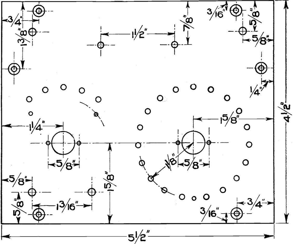
*Drawing, exactly full size, showing the setting out of the positions for the holes. Departures from the dimensions given may be necessary to suit the particular components used.*
