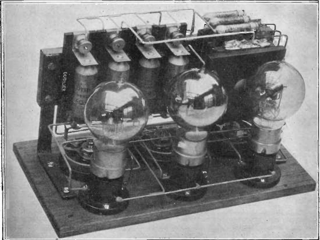
*The interior of the Resistance Coupled Low Frequency Amplifier. The instrument is lifted from the containing case and inverted. It should be noted that the use of ebonite mounting panels is avoided, wood being employed and perfect insulation maintained. Filament brightness can be observed through the gratings in one side of the case.*
