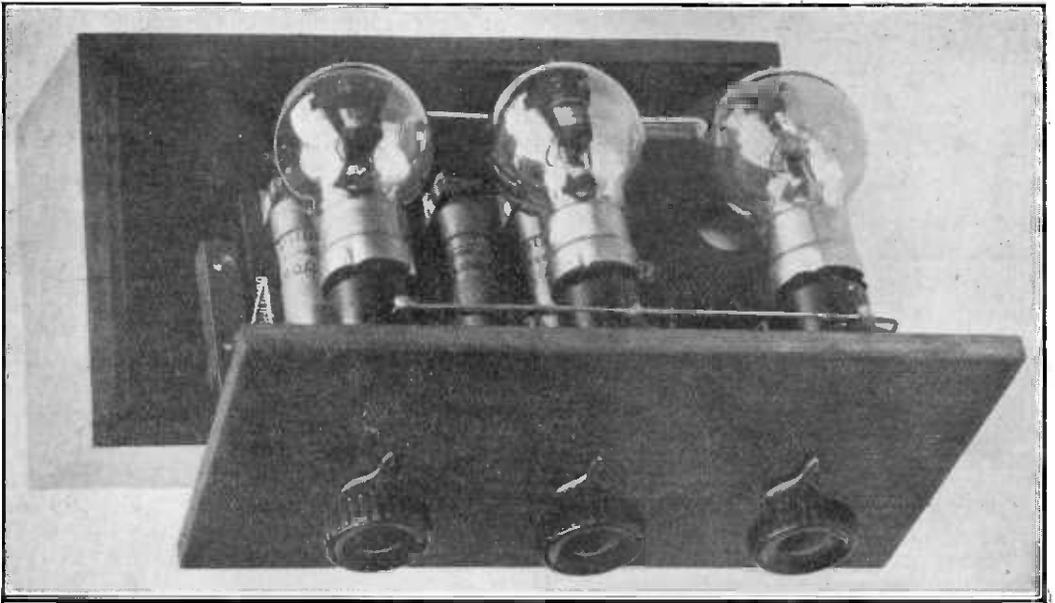
*The complete resistance coupled amplifier raised from the box container.*
