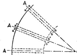
Fig. 2. When the former has been marked out with the aid of the pattern, the slots are cut as at ab-a'b', etc.
