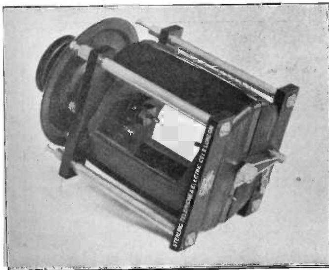
Fig. 8. Another variometer of type 2C. The ends of the windings are brought to terminals, and may be easily joined in series or parallel. Notice the method of making contact with the rotor through the wires which are held against the moving contact with a spring. (Sterling Telephone & Electric Co., Ltd.)
