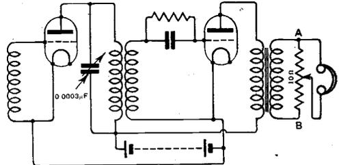
Fig. 3. Tuned H.F. amplifying circuit with an arrangement in the telephone leads for comparing signal strength.
