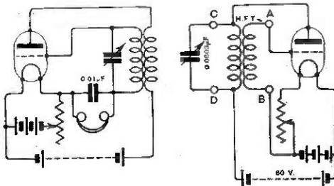
Fig. 4. Heterodyne wavemeter and transformer testing circuit.
