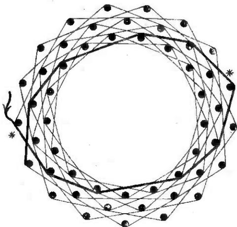
Fig. 10. Example of one of the many possible systems of winding lace coils. One turn is shown for the sake of clearness with a thick line.
