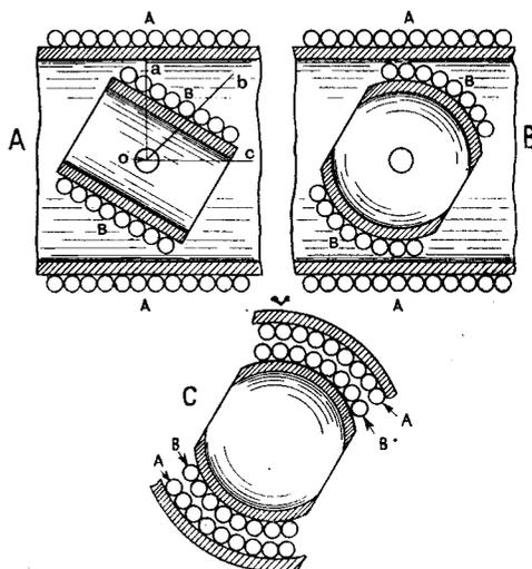
Fig. 2. The shape of some ordinary variometers. A. The fixed winding A is wound on a cylinder and the moving winding is wound on a smaller cylinder B. B. Here the rotor consists of a winding upon a ball. C. This is the best method of all. The rotor and stator windings B and A are wound on portions of spheres, so that they are quite close together.
