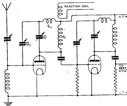
Fig. 4. A valve circuit diagram illustrating the method of neutralising valve capacity.
