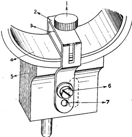
(c) Here the plug 5 has screwed to it at 6 a metal strap 2, which carries a screw 1. By turning the screw, the metal strip 3 is held tightly against the coil 4. The hole 7 is provided so that the arrangement may be fitted to larger coils.
