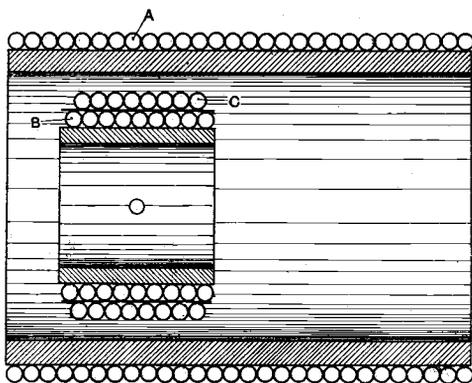
Fig. 2A. Capacity coupling may be neutralised by providing a third winding C, which is wound over the secondary winding B. A sheet of paper or empire cloth separates them.
