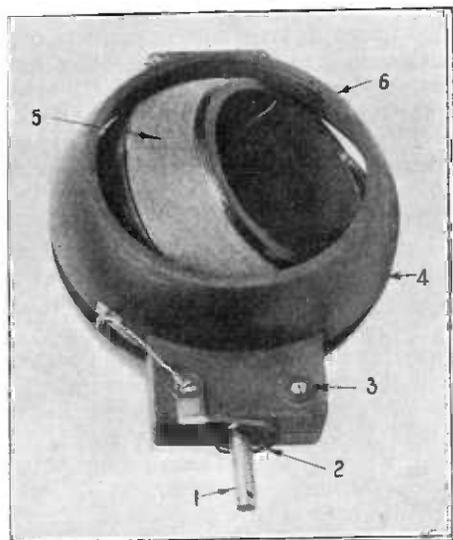
Fig. 7. This variometer is represented in Fig. 2C. Here, 1 is the spindle carrying the rotor 5. The spring 2 makes connection between the rotor and stator 4. Notice the rotor winding 6 is on the inner surface of the stator former. The other end of the coil is connected at 3. (Igranic Electric Co., Ltd.)
