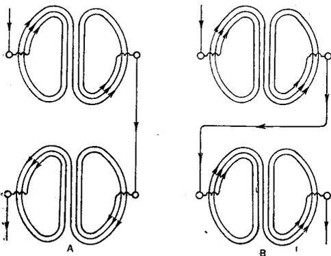
Fig. 13. Here the coils are in series. The inductance is low at A and high at B.
