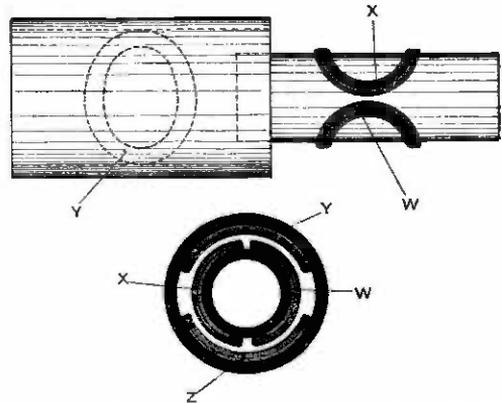
Fig. 15. The arrangement of the coils in a cylindrical type variometer. The smaller cylinder carrying the windings X and W is mounted so that it may be rotated inside of the larger cylinder.
