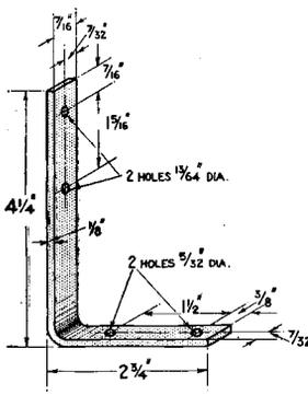
Iron bracket for supporting condenser and resistance rack.
