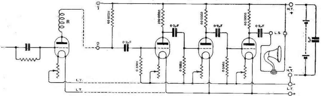
*Circuit of the three-valve resistance coupled low frequency amplifier.*
