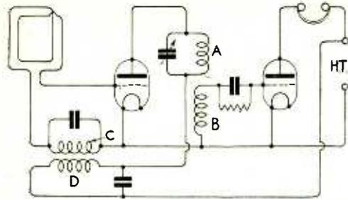
Fig. 5. Another circuit arrangement by which super-regenerative effects may be obtained.
