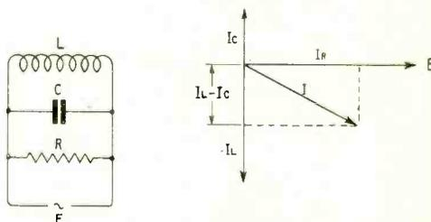
Fig. 66. Inductance capacity and resistance of  $R$  ohms in parallel. The vector relationship is shown. The current  $I$  is the total current from the supply.
