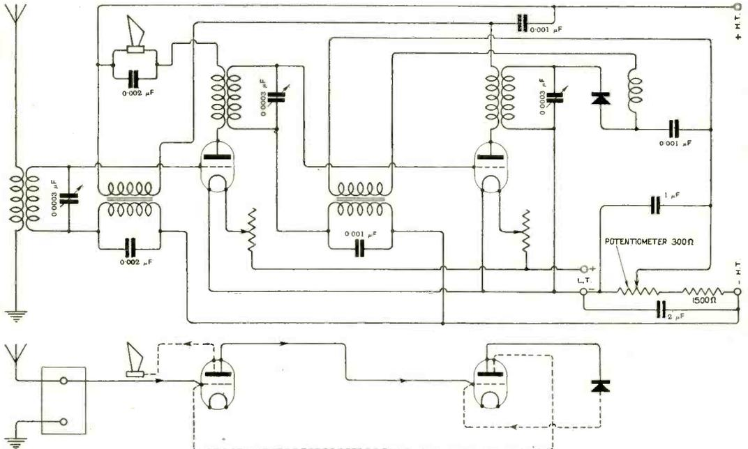
Fig. 1. The figure gives the theoretical connections of the new double magnification receiver. It will be observed that a number of new features are included for the first time. The lower figure shows schematically the circuit arrangement.
