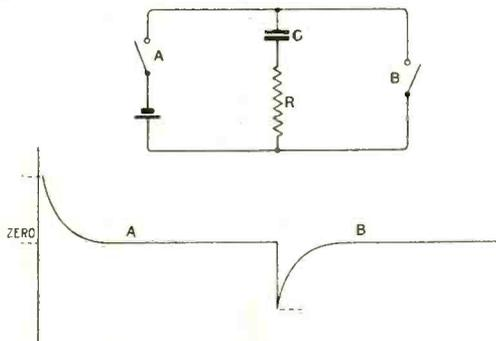
Fig. 58. Curves illustrating the charging and discharging of a condenser in a circuit as shown.
