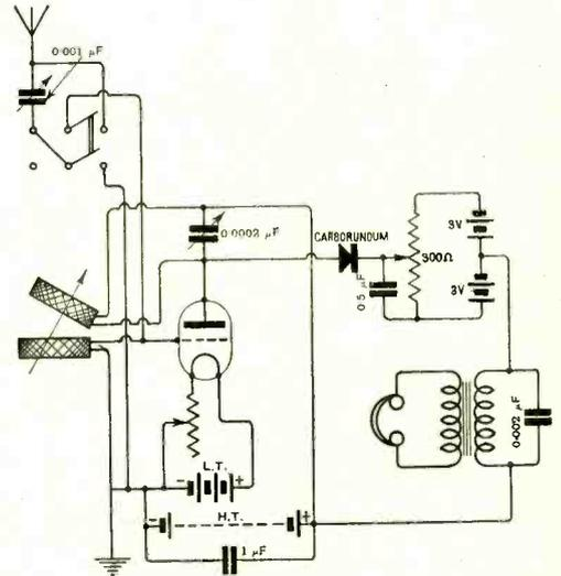
Fig. 1. "J.M." (Manchester). Diagram of a receiver with the valve operating as a high-frequency amplifier and the crystal as rectifier.
