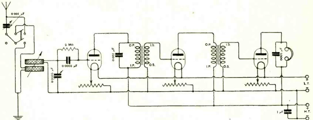
Fig. 2. "Nutty" (Sheffield). Here we have a three-valve receiver—the first valve operates as a rectifier, and the others as note magnifiers.
