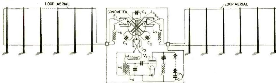
Fig. 8. The Weagant receiving system for eliminating interference.
