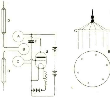
Fig. 2. Circuit of transmitter and arrangement of aerial.
