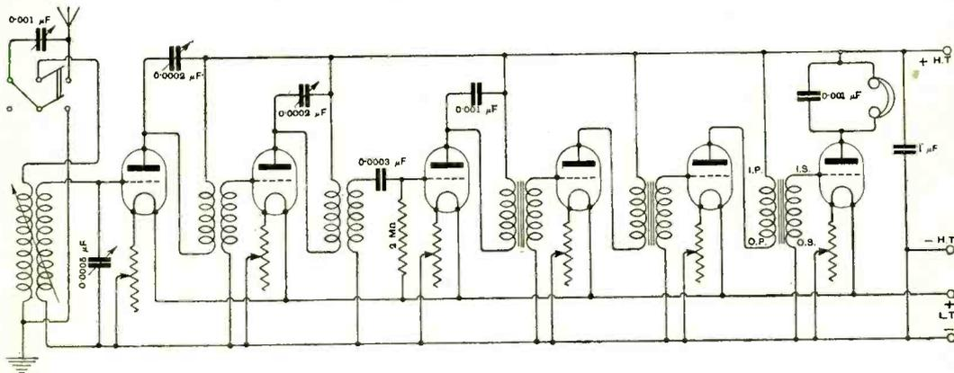
Fig. 1. "RADIO" (Mon.). The diagram gives the connections of a six-valve receiver with two H.F., rectifier and three L.F. valves. Tuned transformers are employed to couple the H.F. valves. No reaction is provided, and the circuit is suitable for the reception of broadcast transmissions.
