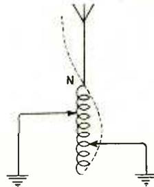
Fig. 4. Potential nodes in aerial system.
