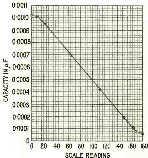
Fig. 2. Calibration curve of standard condenser, arranged so that differences of readings can be read off direct for the determination of values of condensers connected across the terminals of the standard.
