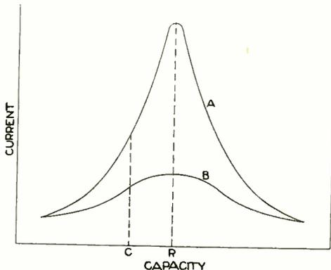
Fig. 64. The curves below show the current which flows in a series circuit when (A) the value of resistance is small, and (B) when the resistance has a higher value. The frequency of the applied pressure remains fixed and the capacity is varied.
