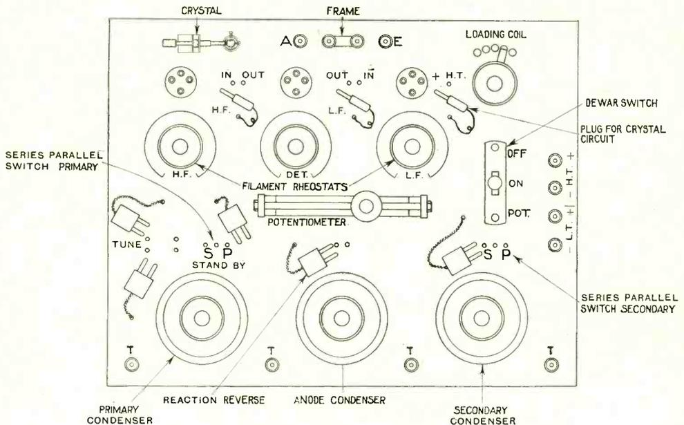
Fig. 3. Lay-out of the components on the face of the panel
