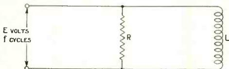
Fig. 52. Circuit consisting of resistance and inductance in parallel.
