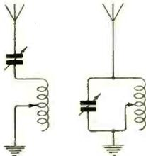
Fig. 1. A simple aerial tuning circuit. For broadcast wavelength work, the condenser may have a capacity of 0.0005 mfd. The coil may be 4 ins. in diameter and 4 ins. long wound with No. 20 D.C.C. with 12 or 14 taps, the more the better.
