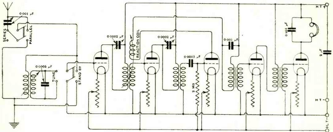
Fig. 2. "H.J.W.B." (Woolwich). A receiver wired according to this diagram is satisfactory for broadcast reception. The first and second valves are coupled with H.F. transformers. The third valve is the rectifier, and the last two are note magnifiers.
