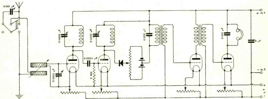
Fig. 1. "QUERY" (Sussex). Diagram of connections for 2 H.F. valves crystal detector and 2 L.F. valves.
