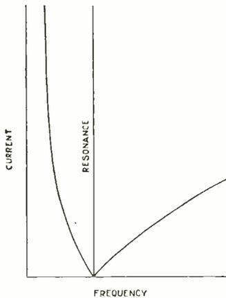
The curve shows the variation in current taken from the supply when the applied frequency is varied. At resonance the current is negligible, that is the circuit has a high impedance. To the left of the resonance point a larger portion of current flows through the inductance; to the right the condenser carries a larger current.
