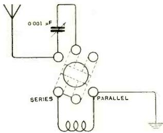
Fig. 7. "A.N.P." (Bristol). Method of connecting a switch to join the aerial condenser in series or parallel.
