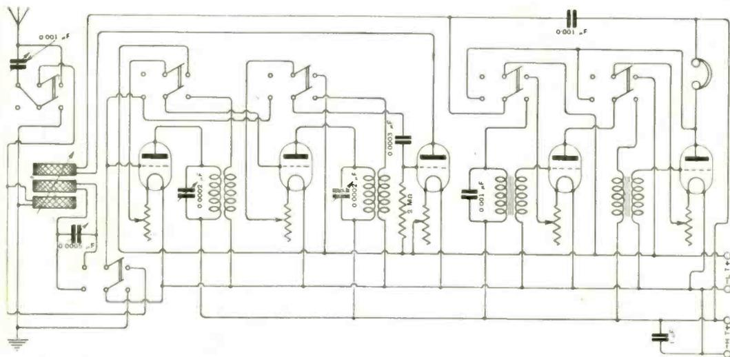
Fig. 1. "H.P.N." (London, W.14). Diagram of a five valve receiver with two H.F., detector and two L.F. stages. Switches are provided to control the number of valves in circuit.
