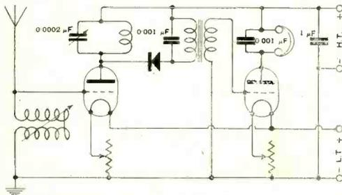
Fig. 6. "SIRKIT" (Lancs.). The first valve operates as a H.F. amplifier, the crystal rectifies and the second valve is a note magnifier.
