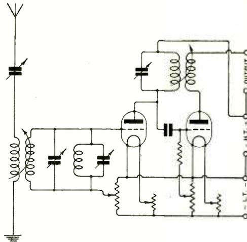
Fig. 13. Another circuit with rejector.
