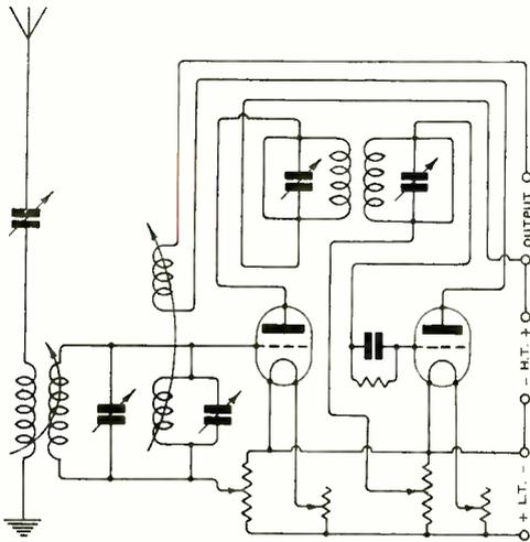
Fig. 12. Receiver with absorption circuit coupled to the reaction inductance for reducing interference.
