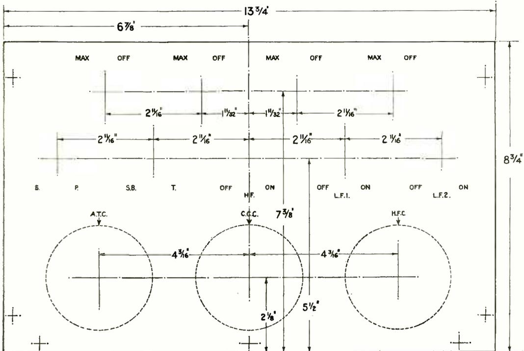
Panel lay-out for supporting the resistances, switches and condensers of a four-valve receiver. Suitable engraving is also indicated. The cross lines represent the centres of the holes for the spindles, the top row being for resistances, the second for the switches and at the bottom the variable condensers.
