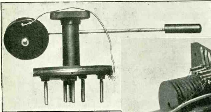
Fig. 1. Plug-in unit consisting of H.F. transformer and reaction coil. (Wellington Electrical and Radio Engineering Works, Ltd.)
