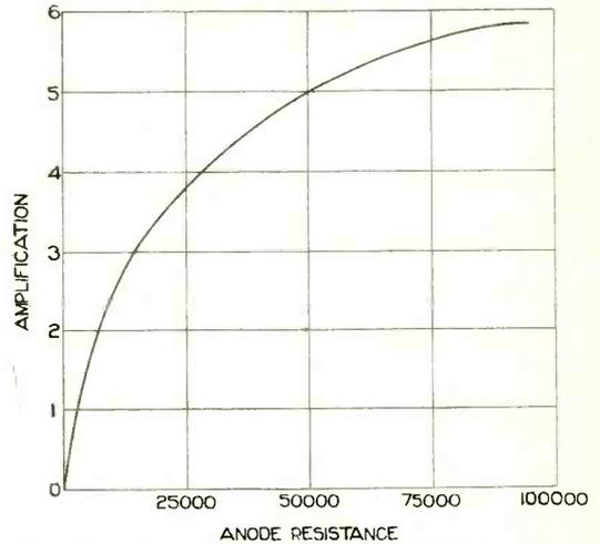
Fig. 57. Curve showing the amplification which may be expected when various anode resistances have various effective values.
