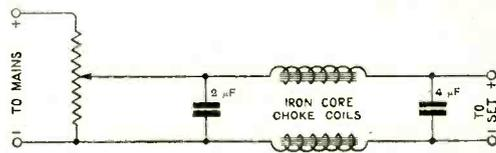
Fig. 4. "J.T.S." (Glasgow). Method of taking H.T. supply for valves from the direct current mains.
