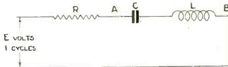
Fig. 59. Series circuit with resistance capacity and inductance.
