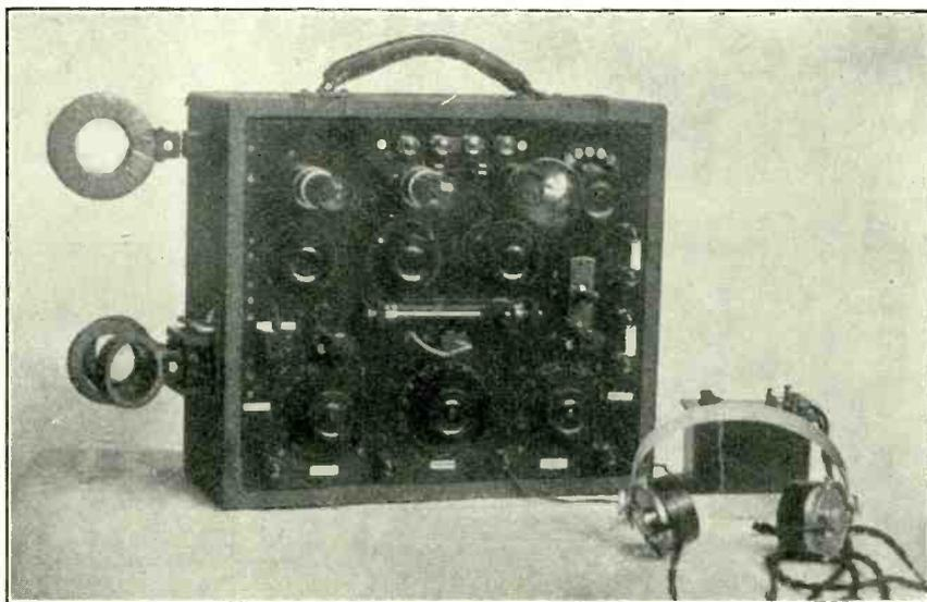
Fig. 1. Portable three-valve receiver, in which provision is made for a number of circuit arrangements.
