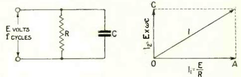
Fig. 55. Circuit consisting of resistance and capacity in parallel.
