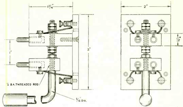
Fig. 4. Constructional details of the two-coil holder.
