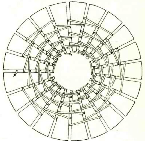
The accompanying sketch illustrates a novel method of winding a basket coil. As usual, an odd number of pegs or slots is used, but the wire is passed round two pegs at a time. The result is a basket coil of duolateral formation which possibly still further reduces the self-capacity.
