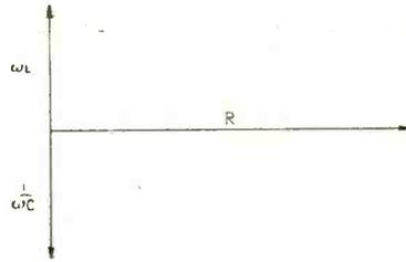
Fig. 62. When  $\omega L$  is equal to  $\frac{1}{\omega C}$ , only resistance is effective in the circuit so far as the total current which flows is concerned. We have then electrical resonance.
