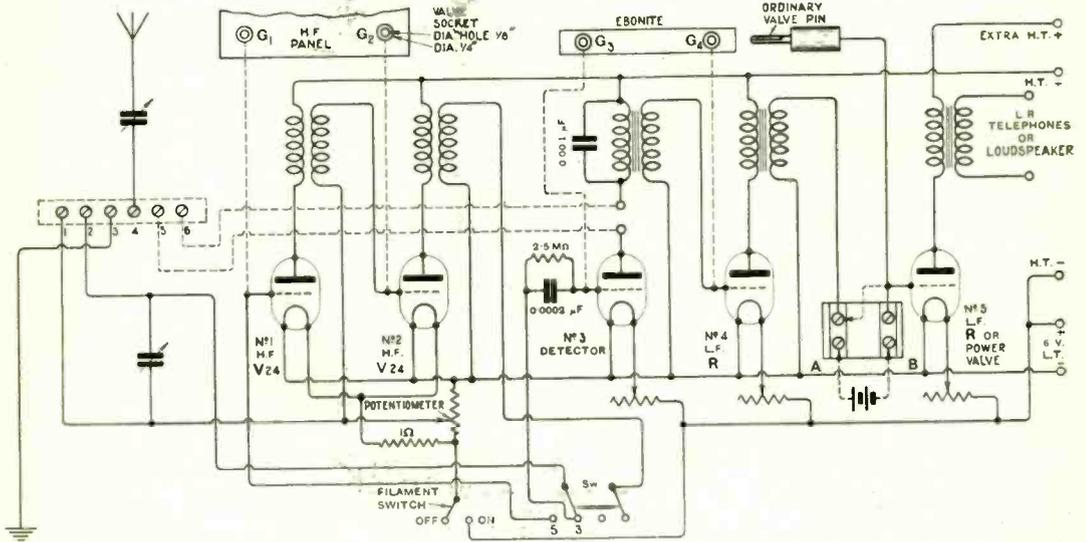
Fig. 1. Circuit diagram of the Receiver, which should be carefully studied in order that the principles may be thoroughly understood, before commencing to adjust and tune-in.
