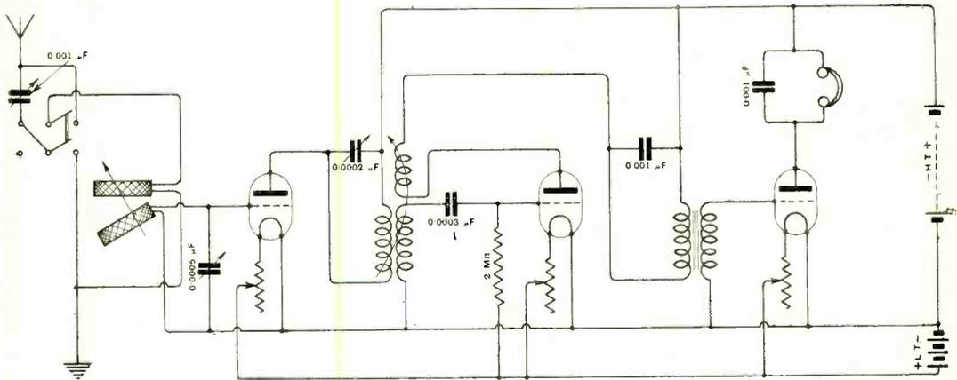
Fig. 3. "C.J.E." (London, W.C.1.) Connections of a three-valve receiver for broadcast reception—H.F., detector and L.F. The reaction coil is coupled with the H.F. transformer.
