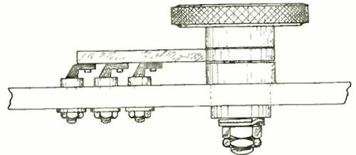
Fig. 2. Details of the switch arm.
