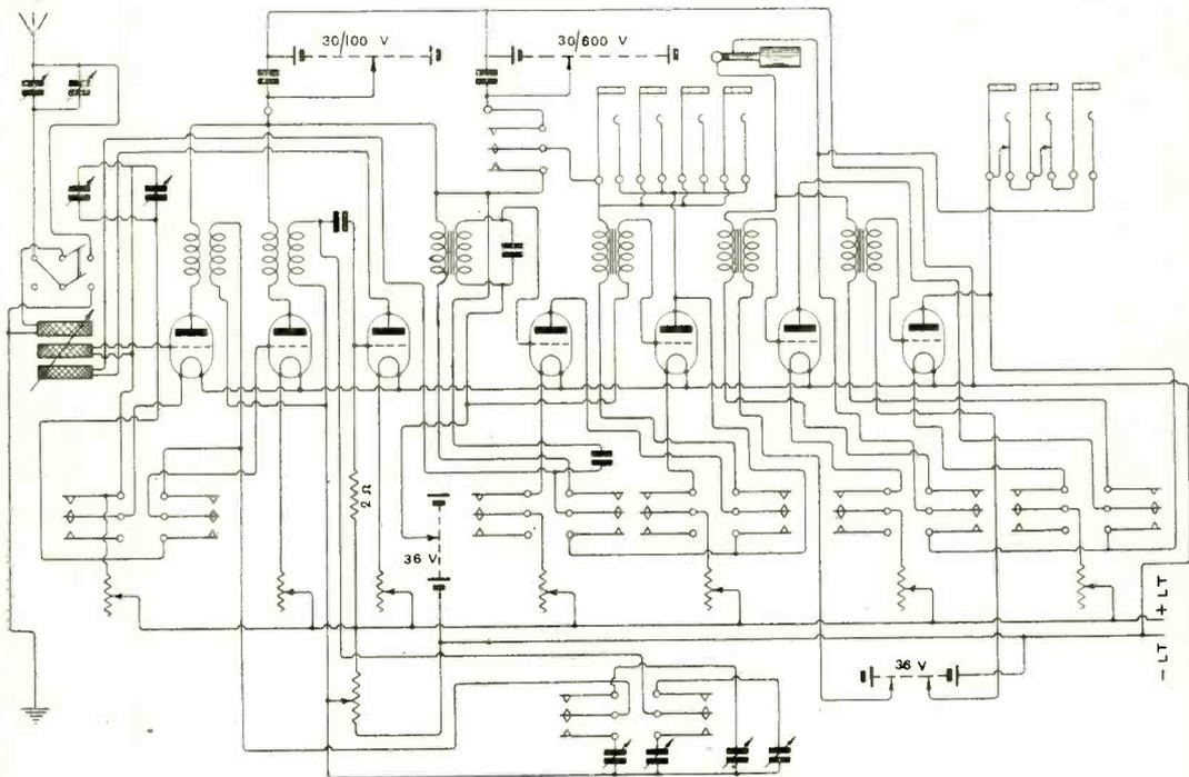
Fig. 4. Circuit of the seven-valve receiver.
