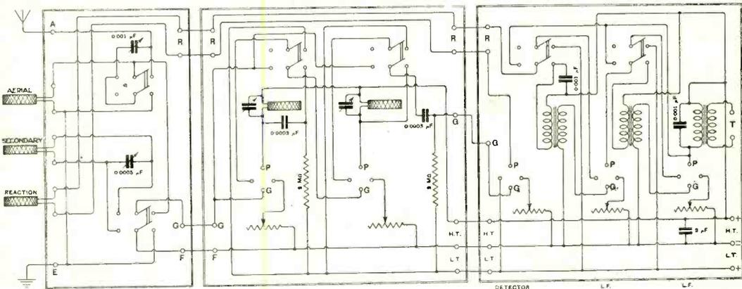
Fig. 1. "M.D." (Edinburgh). The figure gives the connection of three units. (1) Tuner with series-parallel and tune stand-by switches. (2) H.F. panel with two valves coupled with tuned anode coil and grid condensers and leaks, with switches to disconnect them when required. (3) Detector and two L.F. connected valves, with switches to cut out the note magnifiers when required.
