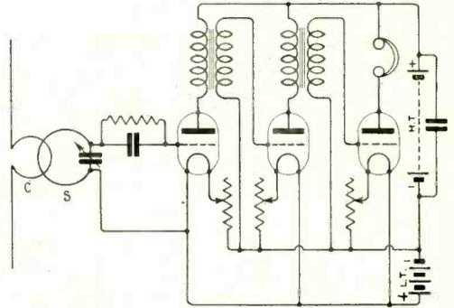
Fig. 8. Circuit of short wave receiver.
