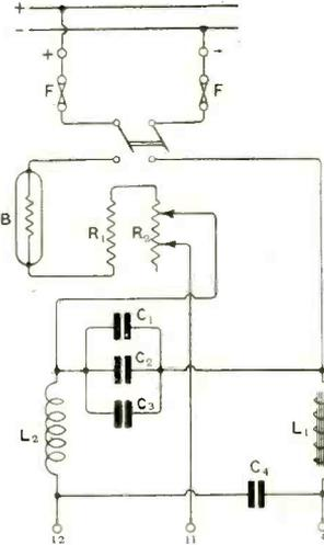
Fig. 12. Circuit arrangement for deriving H.T. and L.T. from D.C. mains.
