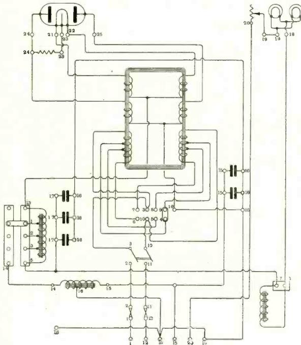
Fig. 16. Circuit of rectifier for supplying filament heating and smooth plate current from A.C. mains.
