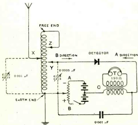
Fig. 15. *Experimental Crystal Receiving Circuit.*
