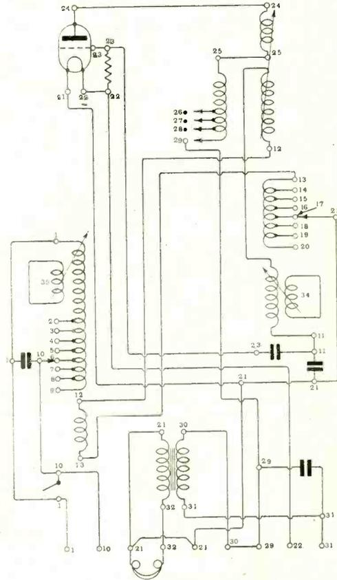
Fig. 4. Circuit of the tuner unit.
