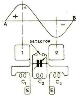
Fig. 7. Principle of the Weagant arrangement.
