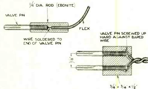
Fig. 5. A simple method of making single and two ended plug connectors.
