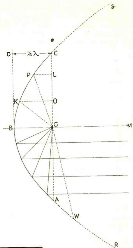
Fig. 5. The transmitter is located at the principal focus, which is arranged to be one quarter of the wavelength employed.
