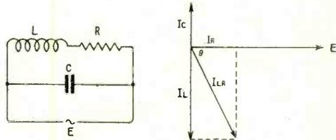
*Fig. 67.* A coil with inductance  $L$  henries and resistance  $R$  ohms in parallel with a condenser. The vector diagram shows the phases of the currents. The current  $I_{LR}$  is the current which flows through the resistance and inductance in series. The current from the mains is obtained by the method of Fig. 66.
