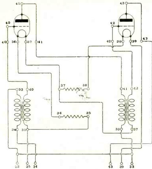
Fig. 10. Circuit of the 2-valve L.F. amplifier unit.
