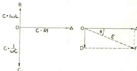
Fig. 60. Vector diagram showing phase relationship in a circuit such as Fig. 59.
