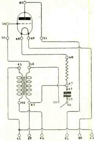
Fig. 7. Circuit of single valve amplifier unit.
