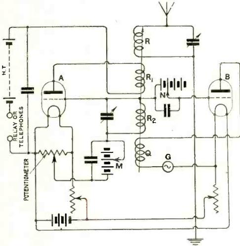
An abbreviated diagram of Capt. Bolitho's circuit.
