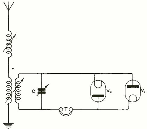
Fig. 6. Balanced valve circuit.
