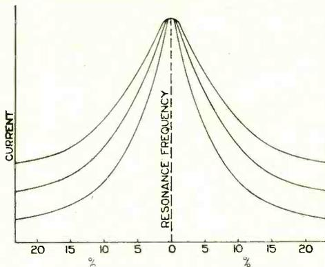
The figure illustrates a number of resonance curves showing how the selectivity of a circuit is improved with a high ratio of inductance to capacity. The upper curve corresponds with a low ratio of  $L$  to  $C$ , and the lower curve with a high ratio of  $L$  to  $C$ . It will be noticed, that for a given % change in the frequency, the amplitude of the current is reduced most in the lower curve—which corresponds with the circuit having the largest ratio of  $L$  to  $C$ .
