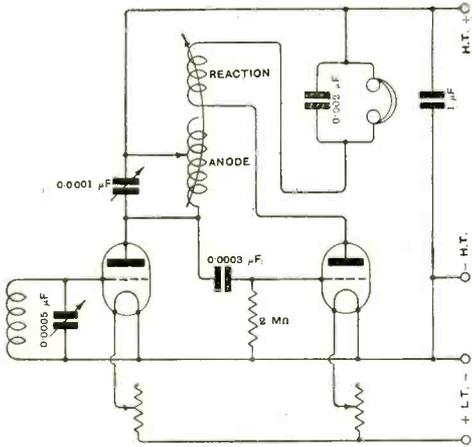
Fig. 4. Method of connecting a receiver using the tuned anode H.F. amplification with reaction coupled to the anode reactance.
