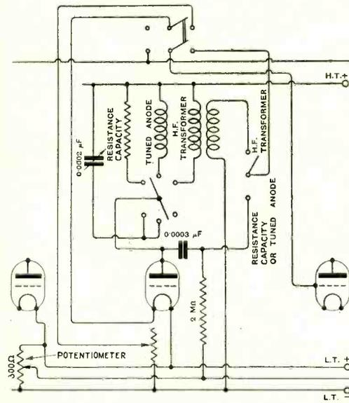
Fig. 5. "A. K." (Charlton). Method of connecting a switch so that the resistance-capacity, tuned anode, or transformer method of coupling may be used.
