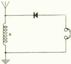
Fig. 2. A simple receiving circuit, which does not permit of selective tuning.
