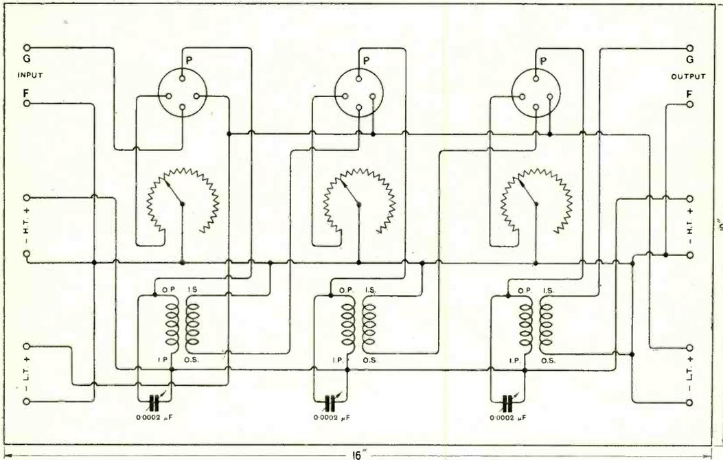
Fig. 5. "P.R.B." (Godalming). Panel with three H.F. valves.
