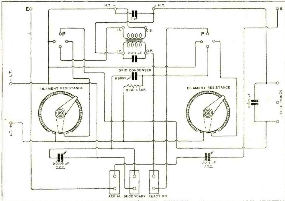
Fig. 3. "W. H." (Sutton). Wiring diagram of a two-valve receiver. The first valve operates as a rectifier and the second as a note magnifier.
