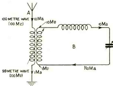
Fig. 10. Distribution of current and potential in receiving oscillatory circuits.
