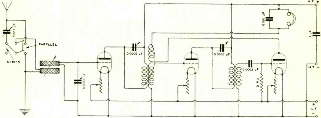
Fig. 3. "AERIAL" (Rugby). Diagram of a three-valve receiver suitable for the reception of broadcast transmissions. There are two H.F. transformer coupled valves and a rectifier. The reaction coil is coupled with the first H.F. transformer.
