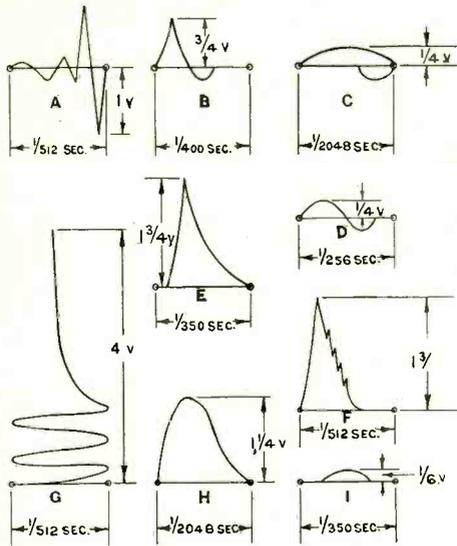
Fig. 2. Curves representing the wave shape of atmospherics.
