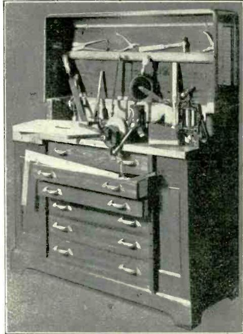
*A fully equipped work cabinet. When not in use the back rack of this cabinet is arranged to close down over the table.*
