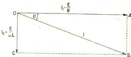
Fig. 53. Vector construction to find the total current  $I$  amperes due to the combined currents  $I_1$  amperes through the resistance and  $I_2$  amperes through the inductance.
