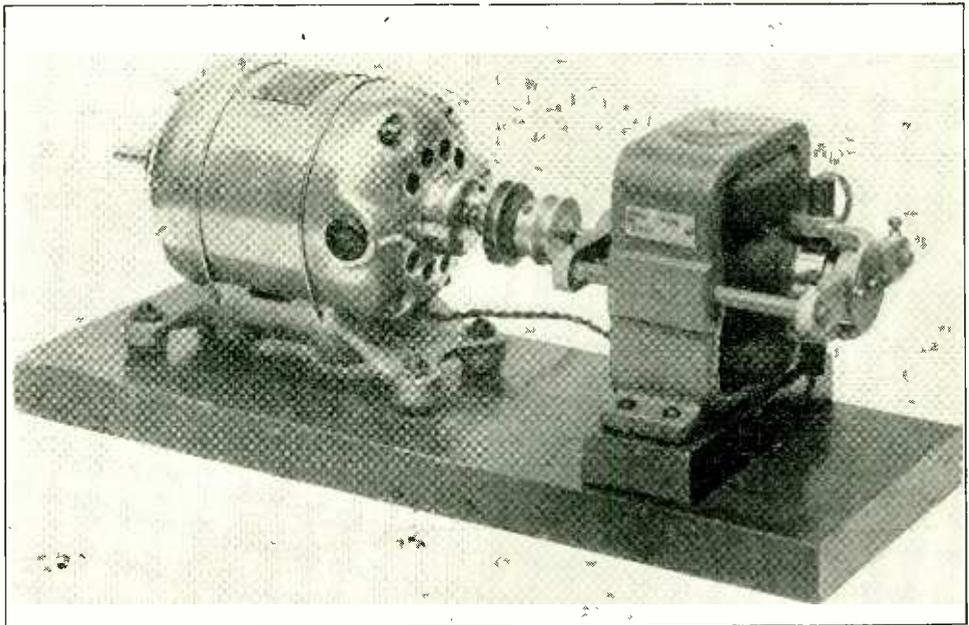
An efficient charging outfit made by Messrs. Serjeant & Rose of Bath Road, Hounslow, for small accumulators such as are used with receiving sets on A.C. or D.C. supply. The substantial motor on the left is driven from the house mains, and the dynamo on the right delivers charging current. It is fitted with ball race bearings and designed for long runs.
