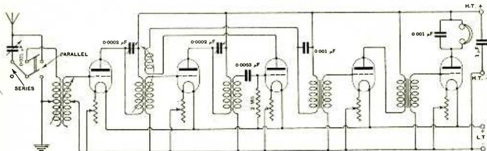
Fig. 5. "H.H." (Leyton, E.10). A five-valve receiver suitable for the reception of broadcast transmissions with two H.F. (transformer coupled), rectifier, and two stages of note magnification.
