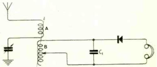
Fig. 3. Selective circuit, not liable to give rise to interference by jamming from stations operating on nearly similar wavelengths.
