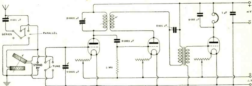
Fig. 6. "K.H." (S. Devon). This is a diagram of a three-valve Broadcast receiver using one H.F., rectifier, and one L.F. valves. All values are given. The reaction coil is coupled with the tuned arc coil.
