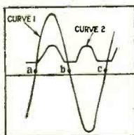
Fig. 1. Curve 1 represents the current amplitude of the A.C. supply and curve 2 the pulsating current delivered by the Rectifier during a corresponding interval of time.
