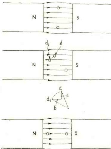
Fig. 35. When the loop is vertical, the pressure induced is zero, as represented at point 0, Fig. 36. As the loop rotates a few lines are cut at first, until when the loop reaches the horizontal position a maximum number of lines are cut, and the voltage induced at this instant is a maximum as shown at 90°, Fig. 36.
