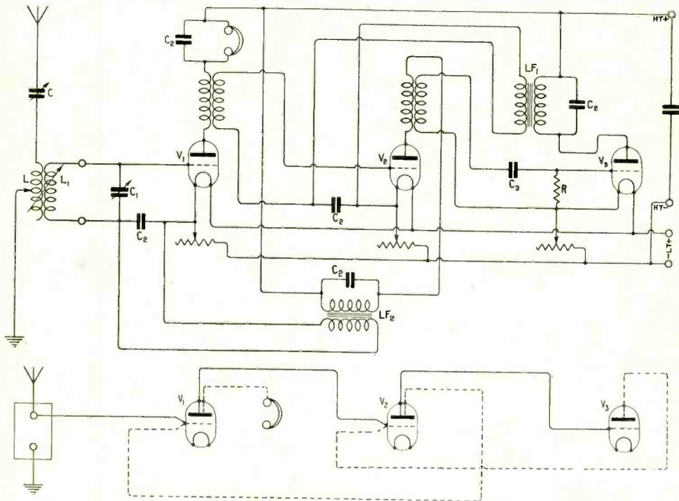
Fig. 10. New Double Magnification Circuit.
