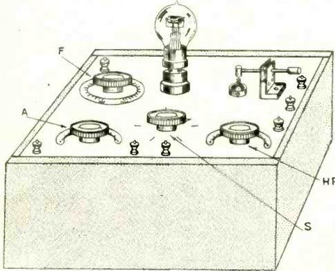
Fig. 1. The simple tuner provided with a barrel switch for five different circuit arrangements, without loss of efficiency.
