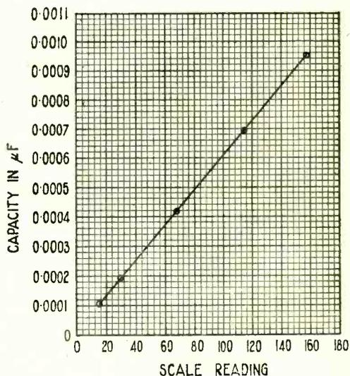
Fig. 2. Preliminary calibration curve of variable condenser, reproduced from Fig. 3 of last article.
