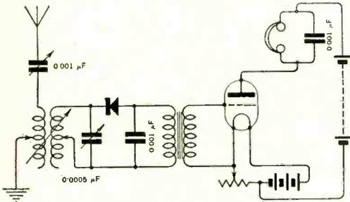
Fig. 1. "L.G.C." (Bucks). Loose coupled tuner with crystal detector and note magnifier.
