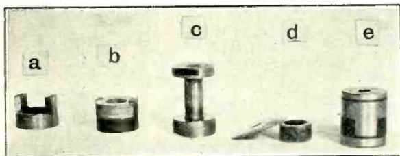
Fig. 2. The components of the interrupting commutators.
