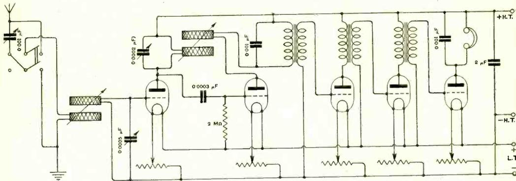
Fig. 1. **"J. D." (Surrey)**. A five-valve receiver with one H.F., rectifier, and three L.F. connected valves. Suitable for the reception of signals of any wavelength.
