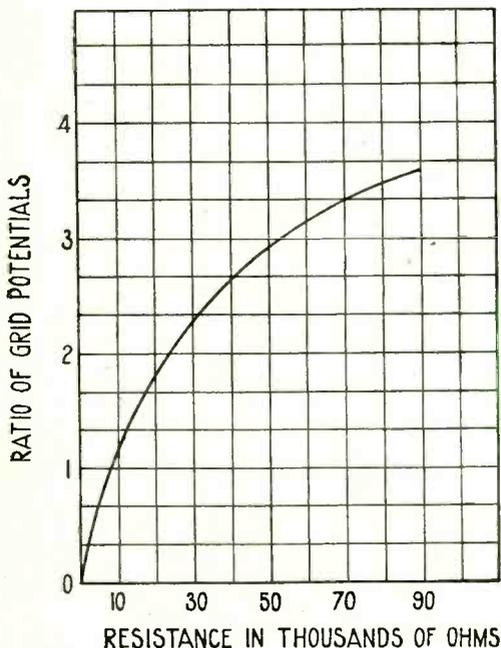
Fig. 4. The curve shows how the ratio of grid potentials between two successive resistance coupled valves, varies with increase in the value of the valve coupling resistance.
