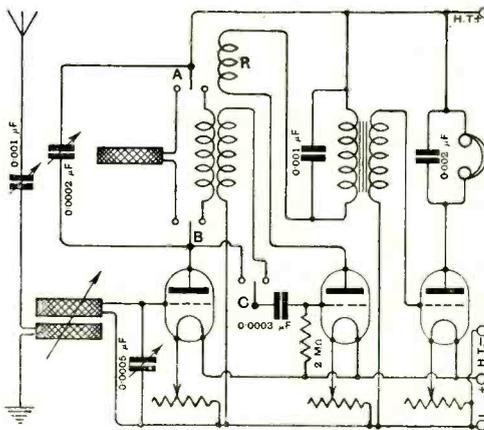
Fig. 3. "R.W." (Nottingham). Method of interchanging transformer and tuned anode by means of switches.
