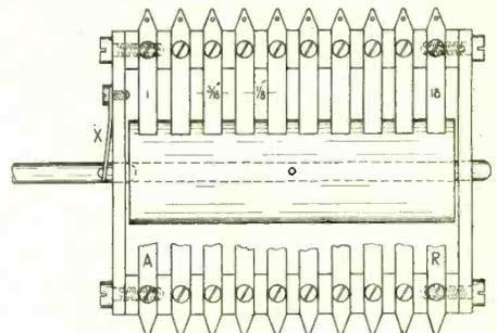
Fig. 12. The fitting up of the contacts.
