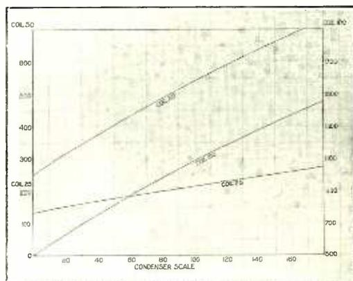
Fig. 9. Curves such as may be obtained for showing the wavelengths produced by various condenser settings with "25," "50" and "100" inductance coils.
