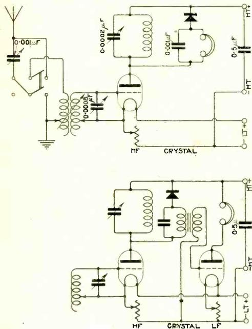
Fig. 8. “E.H.” (W 10). The upper figure gives the connections of a valve with a tuned anode circuit across which is a crystal rectifier. The lower diagram shows the upper diagram with a note magnifier added.
