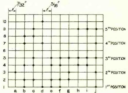
Fig. 10. Positions for inserting pegs in the revolving drum.
