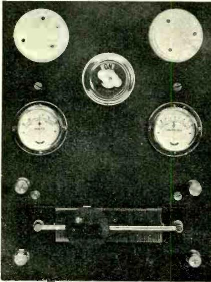
Fig. 4. Switchboard for use with the rectifier. A resistance is provided in order to regulate the charging rate to suit the voltage of the battery. The meters have scales with centre zero to indicate charge and discharge.
