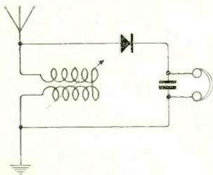
Fig. 3. Position 1. Simple Crystal Receiver.
