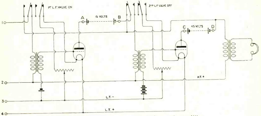
Double pole switches are arranged for cutting out the amplifiers.
