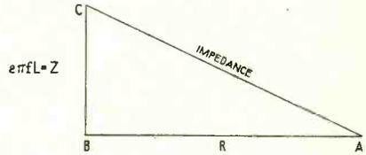
Fig. 51. The impedance of a series circuit containing resistance and inductance is given by  $\sqrt{R^2 + Z^2}$  as seen from the figure.
