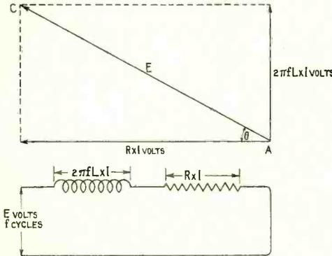
Fig. 50. When a coil and resistance are joined in series there is a pressure drop across the coil equal to  $2\pi fLI$  volts, and another pressure drop across the resistance equal to  $R I$  volts. The two pressure drops must be added vectorially, as shown in the upper figure, to give the pressure across the coil and resistance.
