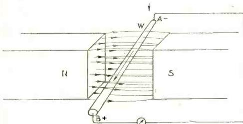
Fig. 32. This figure shows the direction of a current flowing along a wire which is moving through the magnetic field in the direction shown.
