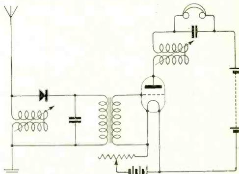
Fig. 6. Position 4. Crystal detector and note magnifier.
