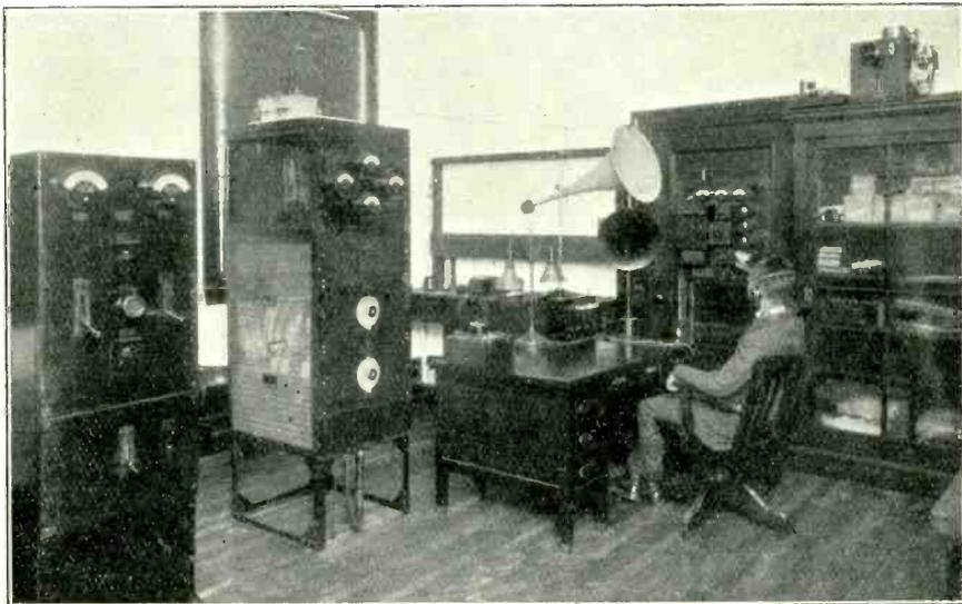
General view of the operating room of the American Station **WHAZ** at the Rensselaer Polytechnic Institute, Troy, N.Y. The equipment was installed for the purpose of collecting data on fading, interference, etc., in long distance short wave communication, and tests have been made for the U.S. Department of Commerce. Musical selections and addresses by prominent men are broadcast every Monday evening at 8.15 Eastern Standard Time (U.S.).
