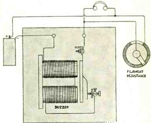
Fig. 2.—Producing a buzzer note in the telephones.
