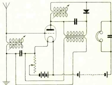
Fig. 7. Position 5. H.F. amplifier, crystal detector and note magnifier. A double magnification circuit. The diagrams show at a glance the circuits obtained.
