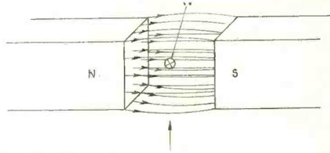
Fig. 33. When the wire moves across the magnetic field in the direction of the arrow, the current flows down the wire away from the observer—represented by the cross on the wire.
