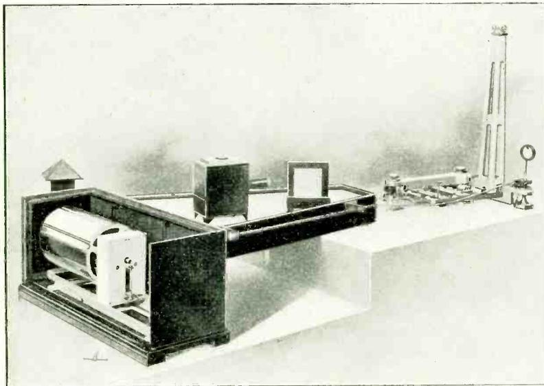
This photograph shows the details of the clock (right of cylinder) and revolving drum. The drum is covered with sensitised photographic paper and the record made by a point of light.
