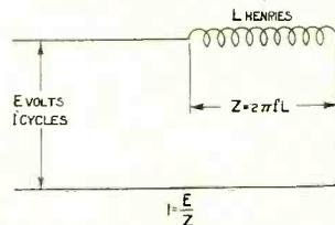
Fig. 47. The current flowing through a coil is given by the pressure divided by the reactance, the reactance being equal to 2πfL where f is the frequency and L the inductance in henries.
