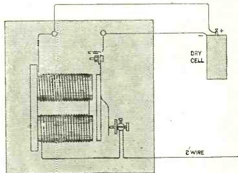
Fig. 6. Should the wiring up of the buzzer be as shown in this figure then the wire must be attached to the contact screw instead of the bracket which supports the armature
