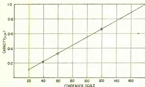
Fig. 12. A simple graph may be used, plotted from points obtained from several determinations, for giving approximate values over the full condenser scale.
