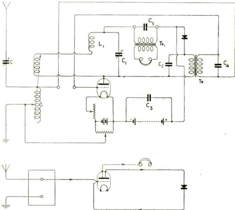
Fig. 3. Single-Valve Double Magnification.
