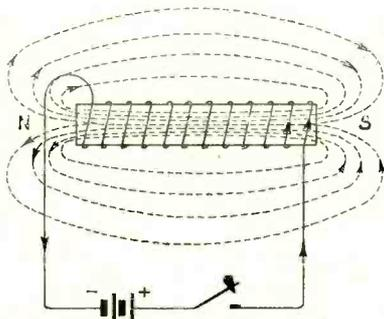
Fig. 26. When a wire is wound in the form of a coil and a battery is connected, a magnetic field is created as shown by the dotted lines. The field has its greatest density along the centre of the coil.
