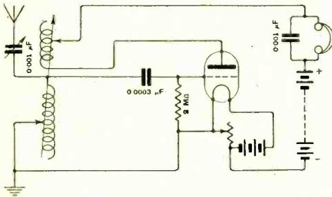
Fig. 6. "W.H.T." (S.E.5). Diagram of a single valve receiver—not recommended for the reception of Broadcast transmissions.
