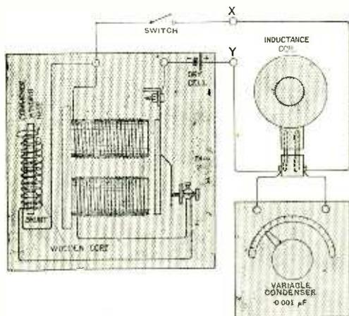
Fig. 8. The shunted buzzer, inductance coil, and variable condenser, connected together to form a buzzer wavemeter.
