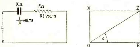
Fig. 42. Circuit containing capacity and resistance in series. The right-hand diagram shows the phase relationship.
