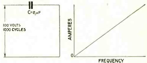
Fig. 41. When the quantities have the values given in the left-hand figure, the current which flows is 1.11 amperes. The condenser current increases with frequency as shown by the curve.
