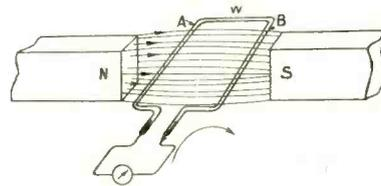
Fig. 34. When a loop is rotated in a magnetic field, the voltages induced in each half of the loop have such a direction that they add together.
