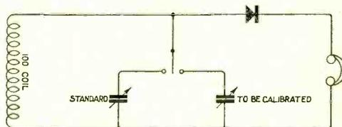
Fig. 11. The circuit arrangement by which a variable condenser of unknown capacity may be compared with a standard.
