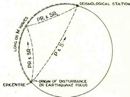
Fig. 1. Diagram showing wave motion through the earth.
