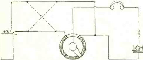
Fig. 4. Illustrating the operation of a crystal detector.
