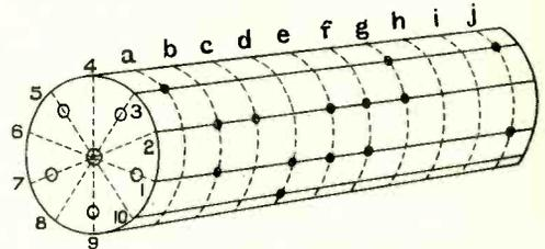
Fig. 11. Method of dividing the drum.
