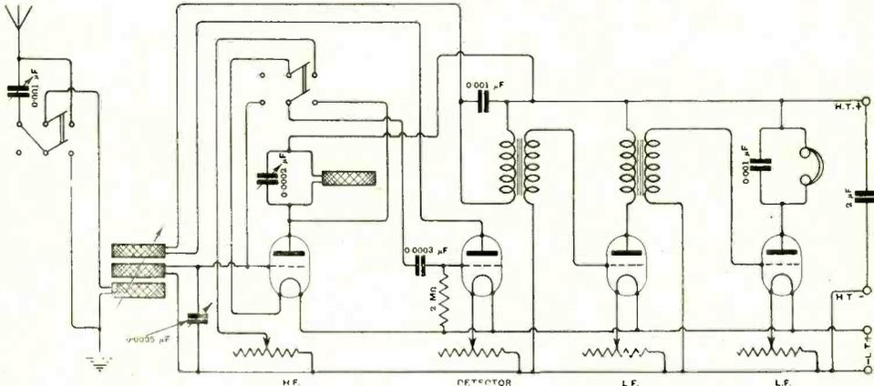
Fig. 4. "Sparks" (Cheshire). Here is a four-valve receiver with one high frequency connected valve, rectifier and two note magnifiers. The first valve may be cut out when required with the switch. The circuit is quite suitable for the reception of broadcast transmissions, provided the reaction coil is not used.
