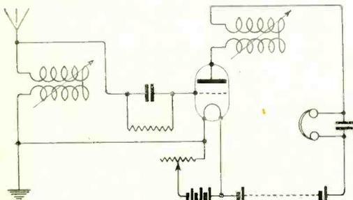
Fig. 4. Position 2. Valve detector with tuned plate circuit.
