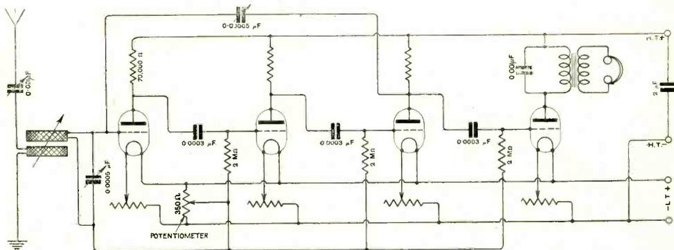
Fig. 2. "SCAMP" (Finchley). Method of joining up an amplifier on the resistance capacity principle.
