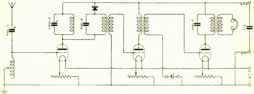
Fig. 2. "East Boldon" (Newcastle). A three-valve receiver. The first valve operates as a high frequency amplifier. The crystal rectifier and transformer are joined across the anode coil. The second and third valves operate as note magnifiers.
