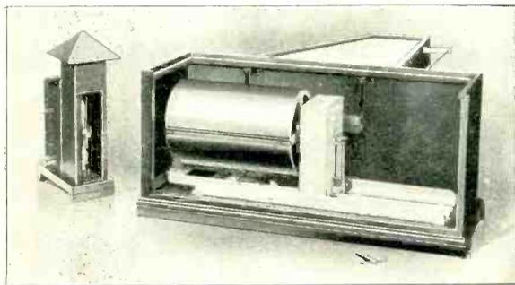
*A clearer view of the revolving drum and clock. The lamp can be seen on the left.*
