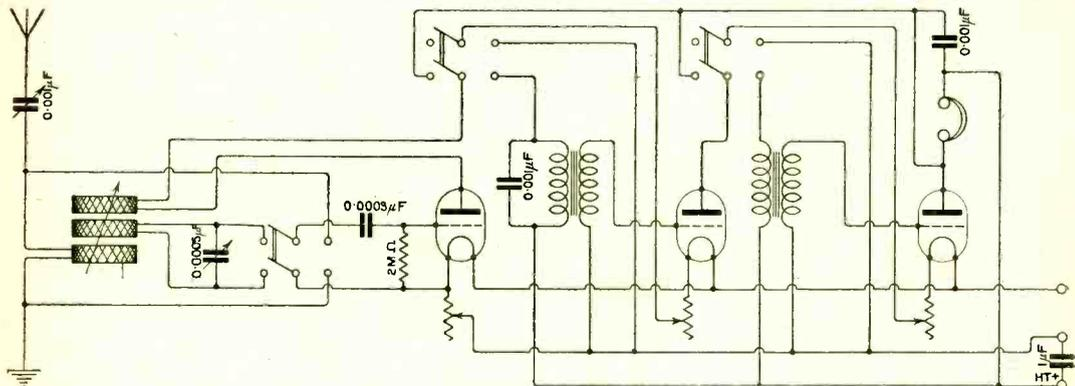
Fig. 7. “R.M.” (N.2). Diagram of a three-valve receiver. The first valve operates as a rectifier, and the others as note magnifiers. Switches are connected for the purpose of controlling the number of valves in circuit.
