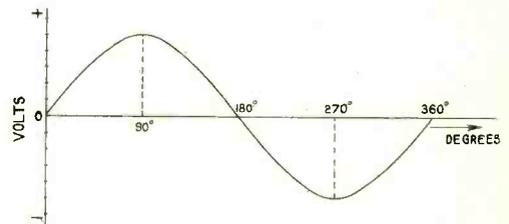
Fig. 36. The pressure induced in the loop varies as shown in the above curve, which is a sine curve, when the loop rotates in a uniform magnetic field.
