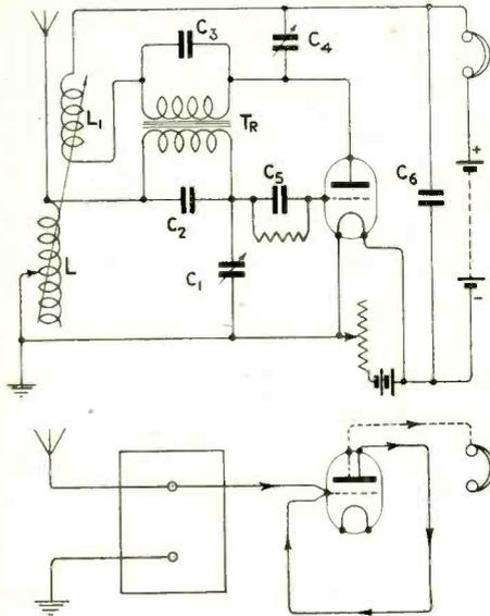
Fig. 4. Single Valve Double Magnification. This arrangement is attributed to Armstrong. The valve operates as a rectifier, and reaction effects are obtained by coupling coils  $L_1$  and  $L$ . Condenser  $C_4$  tunes the reaction coil. The rectified energy is fed back to the grid circuit through  $Tr$  and operates the telephones. The components have usual values.
