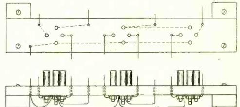
Fig. 8. Valve socket connections.
