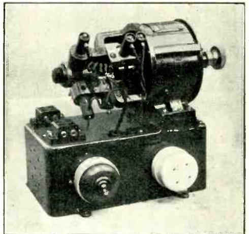
Fig. 1. The Rotary Rectifier. This model has an output of 3 amps. at 15 volts. The iron base box measures 9" x 5"
