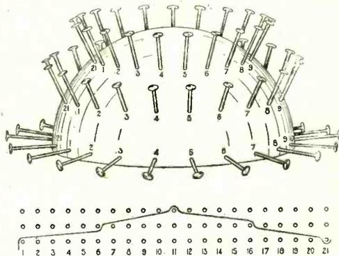
Wooden hemisphere with wire nails used for winding the variometer stator. The manner in which the wire passes over the nails is indicated.
