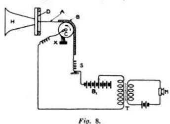
It is not essential that the semi-conductor should be in the form of a rotating cylinder or disc, as implied in the above descriptions, but, if preferred, the semi-conductor may be stationary, and merely its metal core may revolve. A number of applications of the apparatus as arranged in this form are described by Messrs. Johnsen and Rahbek in their patent specifications.
