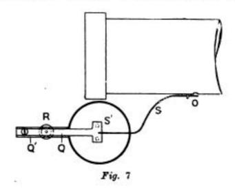
to the width of the lines forming the record. When the relay is at rest, this aperture is covered by the shutter O resting lightly on a pin or stop P. In the sketch the aperture is fully open, the shutter lever being in contact with the upper pin P'.
