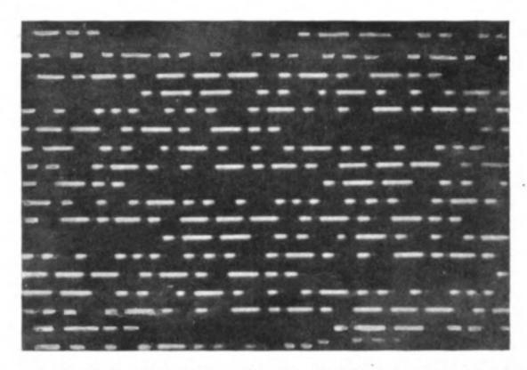
A Print made from a specimen film. It will be seen that signals broken on the righthand side are completed on the left-hand side on the next line.
