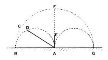
"Thus, in the diagram, if AB represent the magnitude of the field-strength vector at any horizontal distance AB from the aerial AE, then at C, any point on the hemisphere of radius AB, the vector will
