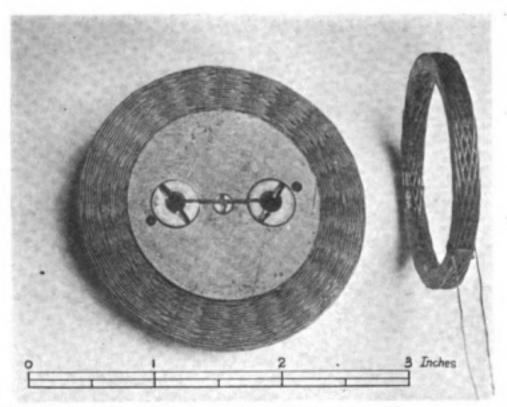
Fig. 2. Two coils, one of them with centre ebonite disc and brass hollow screws for quick connection.
