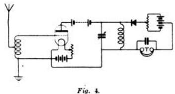
ELECTRON (South Shields) .- (1) Yes; connect the blocking condenser across the H.T. battery as well as the telephone transformer primary.
