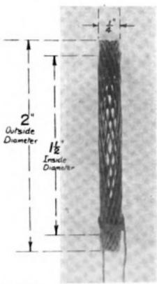
Fig. 1. Machine Wound Honeycomb Coils showing the formation of the wire.
