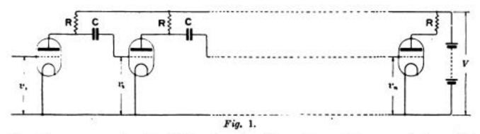
Fig. 1 represents the 1st, 2nd and n-th valves of a resistance-coupled amplifier.†
