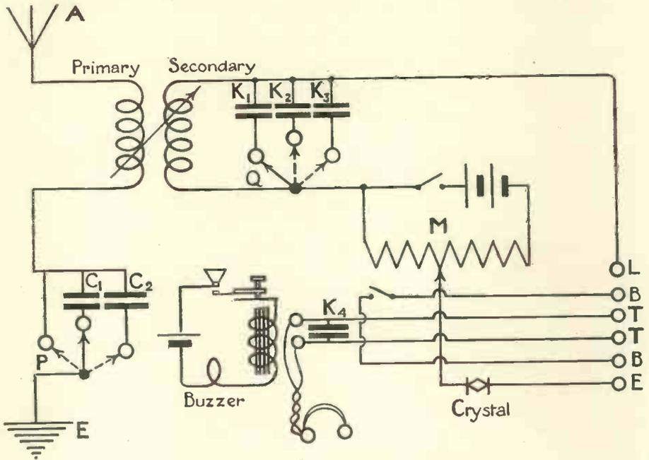
Fig. 29. Schematic wiring diagram of T6 Receiver.
