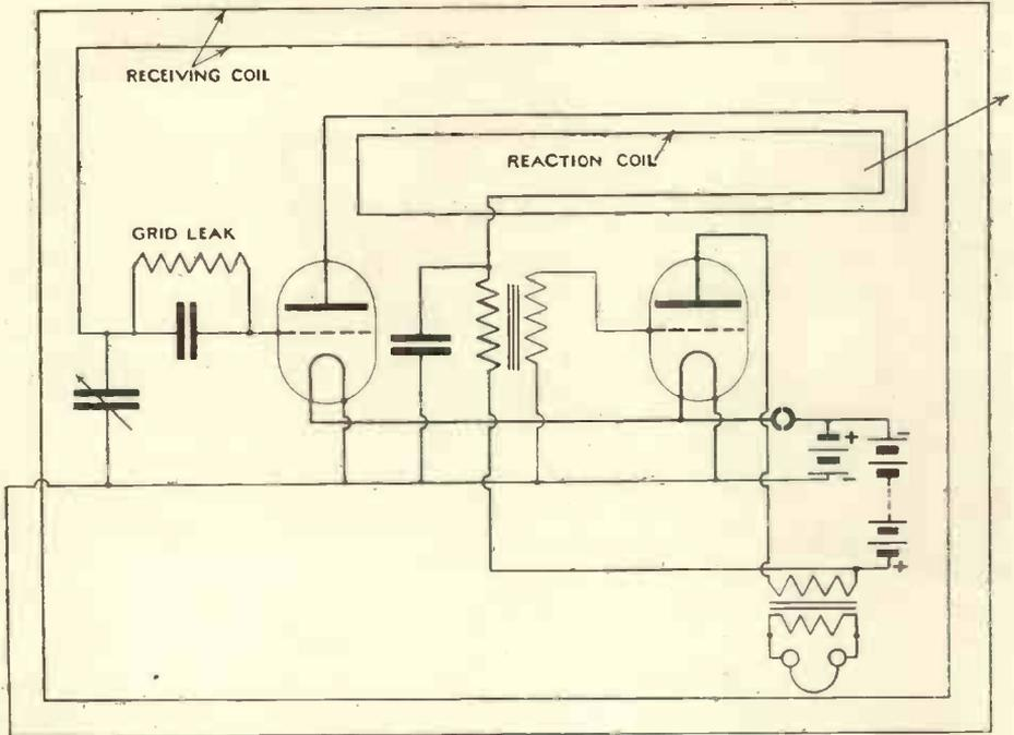
CONNECTIONS OF PORTABLE RECEIVER
