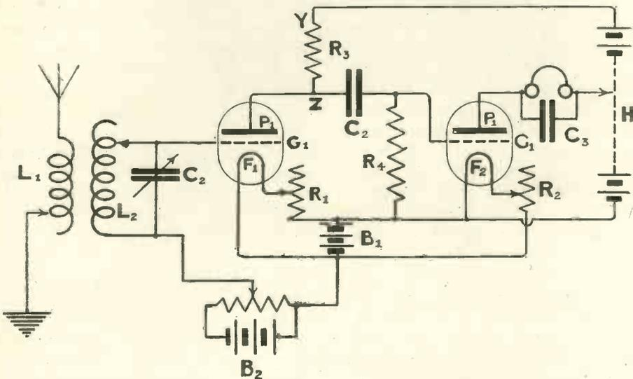
Fig. 15. Two-valve Resistance Amplifier.
