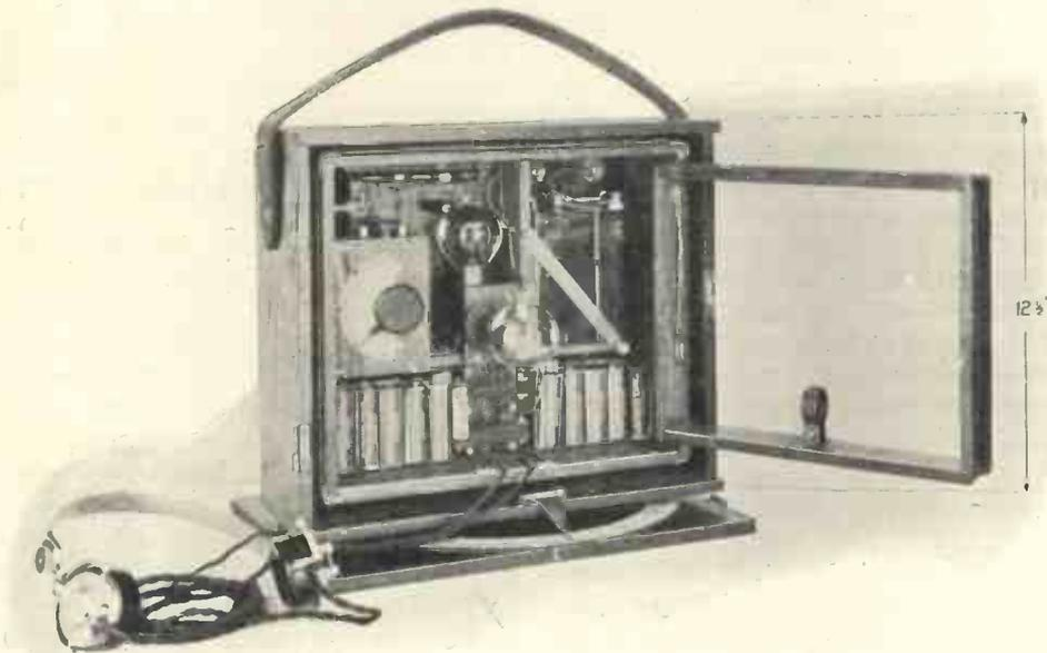
*Fig. 2. Portable Receiver on pivot.*
