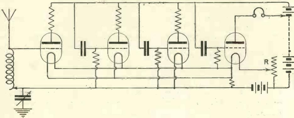
Fig. 16. Four-valve Resistance Amplifier.
