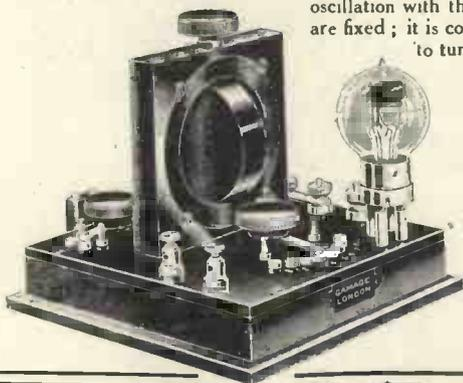
With the addition of a variable condenser and loading coil, we have received, *inter alia*, the United States Station Annapolis (N.S.S.) wavelength 16,900 metres with a single wire aerial 100 feet long and 35 feet high.
