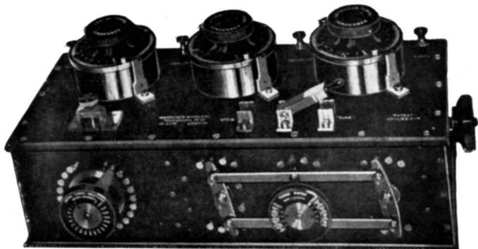
The Marconi Multiple Tuner for adjusting to the various Wave Lengths.
