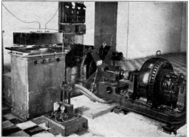
The Transmitting Apparatus, showing Rotary Spark Gap, with H.T. Signalling Key in foreground. Pipes convey the air blast to the contact.
