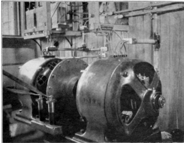
*Fig. 3.—The 5-k.w. Transmitting Sets.*
