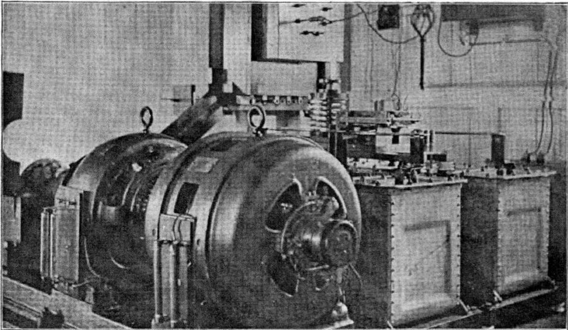
*Transmitting Apparatus at Suva—5-K.W. Disc Set.*
