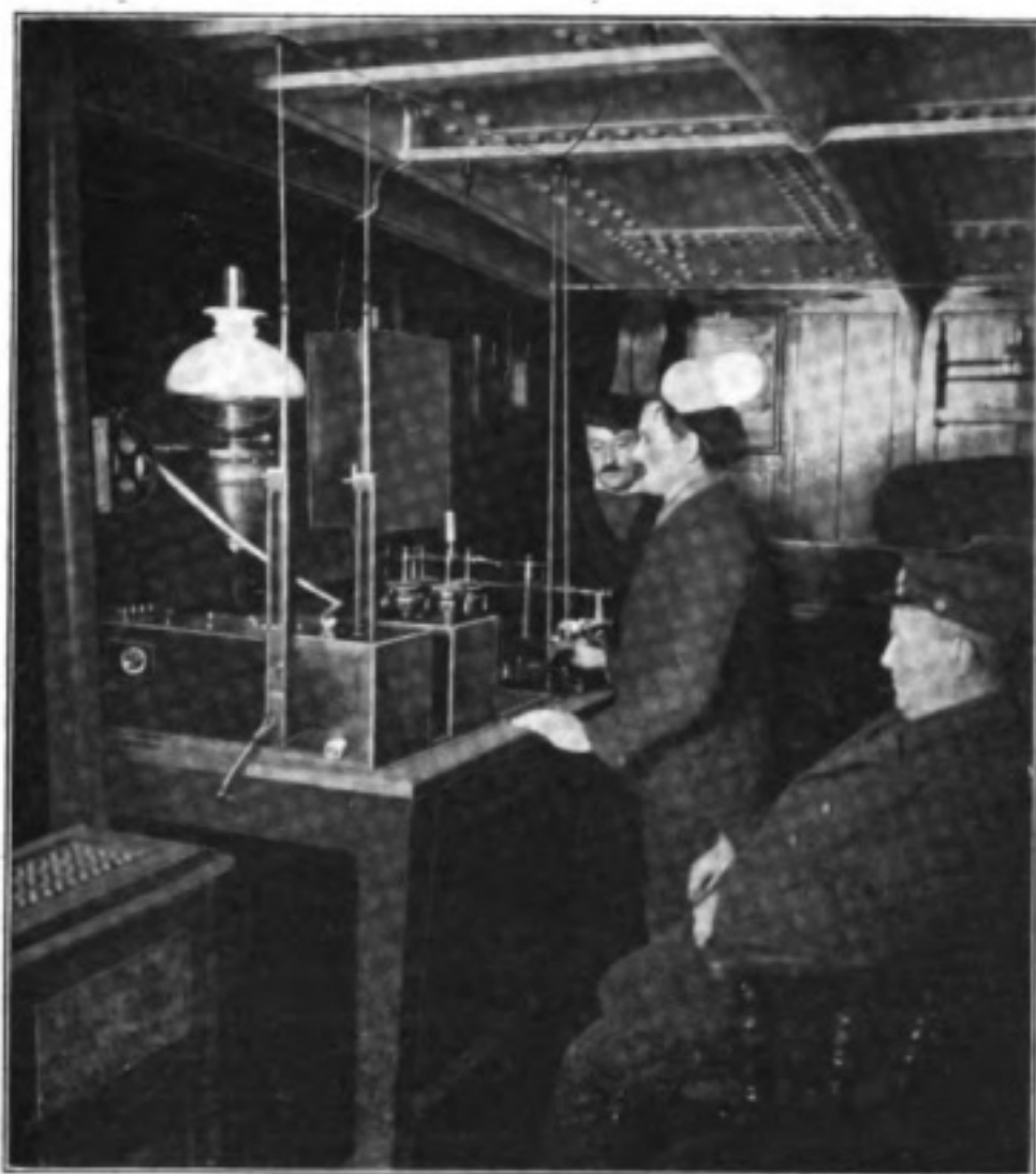
The Wireless Apparatus on the "Tongue" Lightship.
