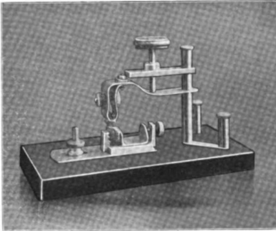
**T**HE crystal detector usually found in an amateur installation is one which has the crystals sealed into brass cups with a metal of low melting point, such as Wood's metal.
