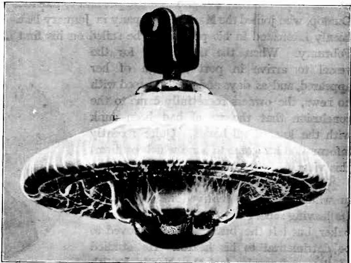
THE INSULATOR "SPARKING-OVER" ON TEST.
