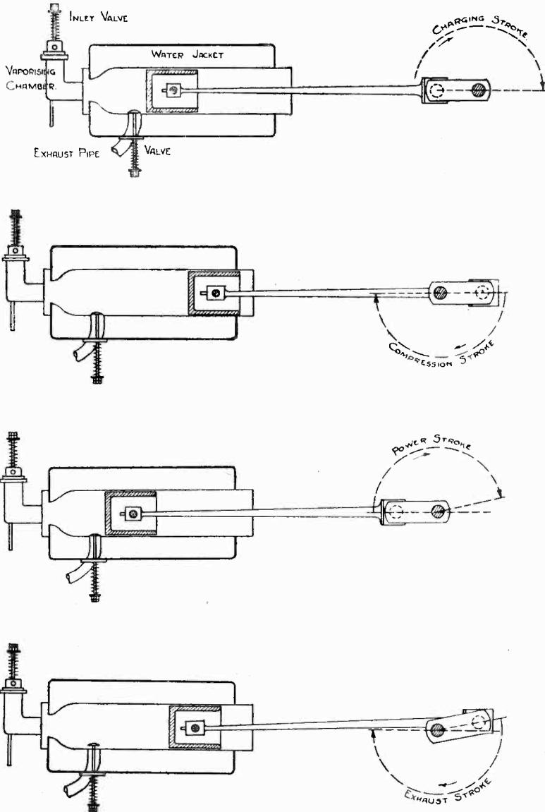
THE FOUR STROKES OF AN OIL ENGINE.
