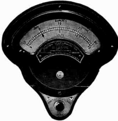
**T**HIS Model normally indicates amperes, but upon pressing the contact button the pointer indicates volts so long as the button is held down.
