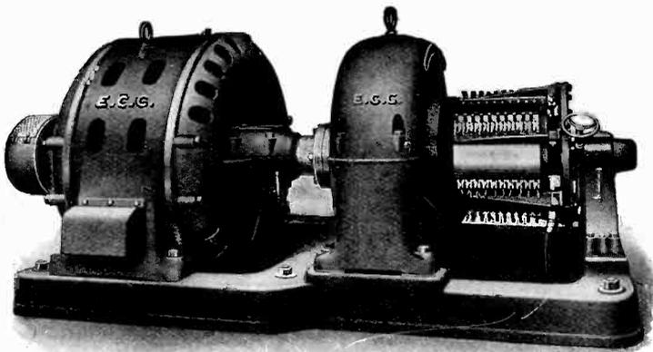
125 Kw. Singlephase to D.C. Induction Motor-Generator, 575 r.p.m.
