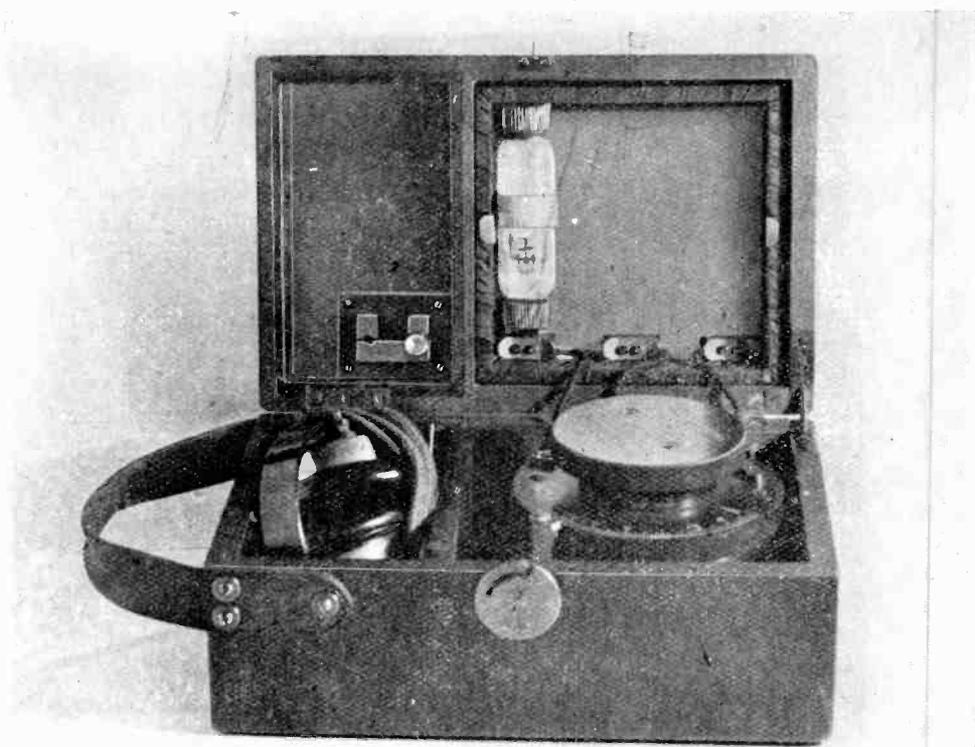
THE MARCONI VACUUM AMPERE GAUGE MOUNTED IN A WAVE-METER.
