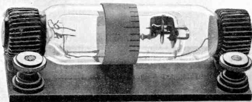
ANOTHER FORM OF THE AMMETER MOUNTED ON AN EBONITE BASE.
