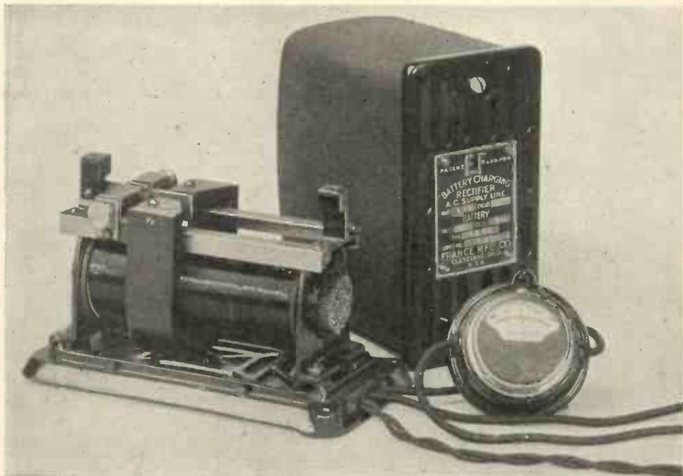
current is rectified by means of the vibrating tongue, which, actuated by magnets in circuit with the alternating supply, automatically connects the line first to one pair of contacts, then the other in exact synchronism with the supply current. The device has thus no rotary parts, and being simple of construction, can be marketed at low cost.
