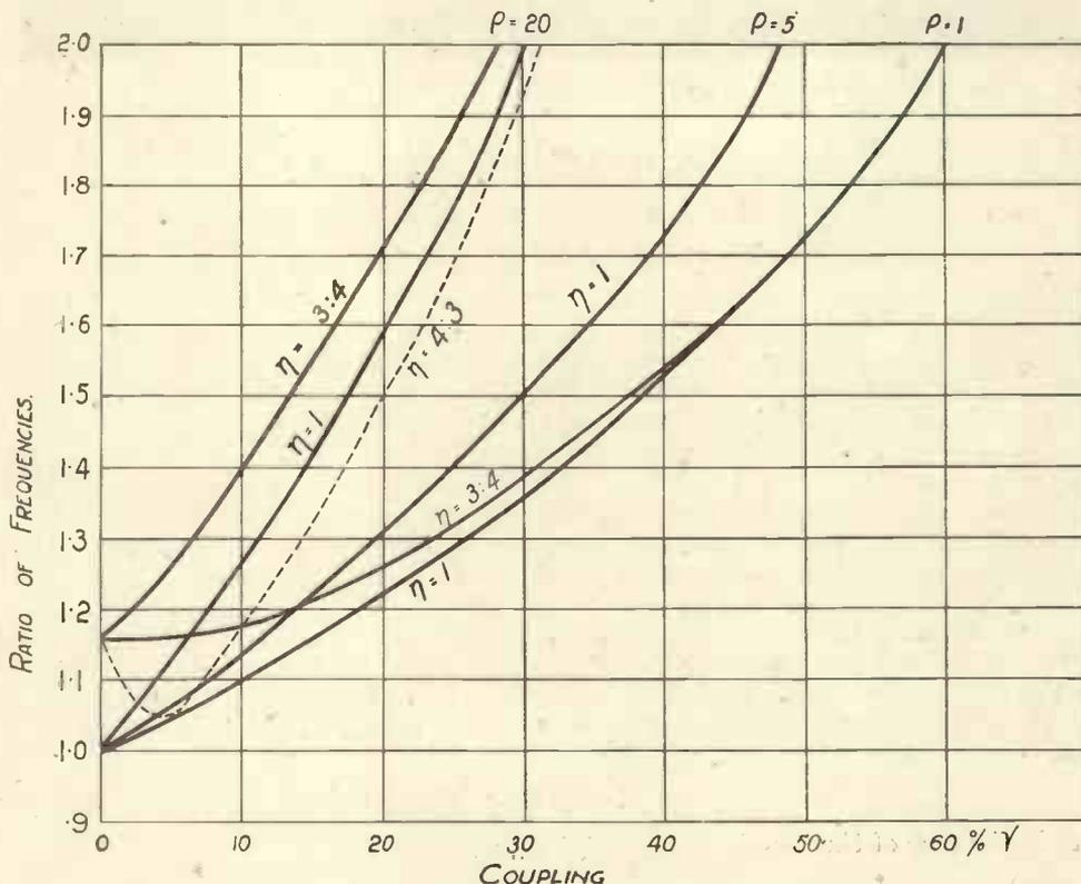
FIG. 9.—FREQUENCY RATIO AND COUPLING.
