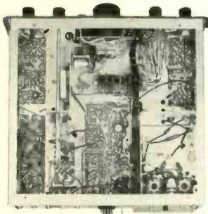
Sectionalized layout on circuit boards simplifies construction—makes components accessible and easy to locate.
