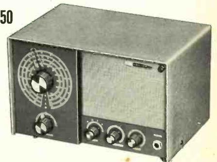
**GR-81 SPECIFICATIONS**—Frequency coverage: 140 kc to 18 mc on four bands. Tube complement: 12A7 Detector/1st Audio, 50C5 Audio Output, 35W4 Rectifier. Power requirements: 105-125 V 50/60 cycle AC only, 30 watts. Fused. Controls: Main tuning (calibrated), Bandspread, Bandswitch, Regeneration, on/off volume, phone jack. Dimensions: 10" W x 7" H x 7" D.
