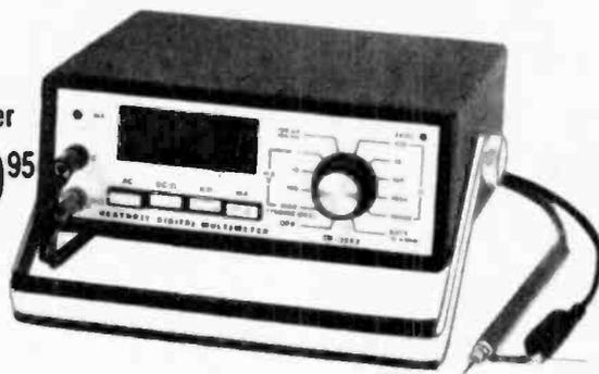
Features 26 ranges, 100% overrange capability, separate voltage and current inputs, overload protection. Battery or AC operation.
