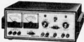
**Easy-to-use General-purpose Power Supply.** Provides 0-400 VDC output at 0-100 mA continuous (125 mA intermittent). The front panel voltmeter measures from 0-400 or 0-150 volts, the front panel ammeter from 0-150 mA. For 120/240 VAC, 50/60 Hz. 5 1/4" x 13 1/4" W x 11" D.
