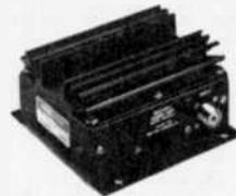
**HA-202A SPECIFICATIONS:** Power Output: 20 W @ 5 W in. 40 W @ 10 W in. 50 W @ 15 W in. Impedance: 500 ohm. Input VSWR: 1.5:1 max. Max. Stable VSWR: 3:1. Harmonic and Spurious Radiation: — 60 dB or better. Standby Current: 1 mA. Power Requirement: 12-16 VDC, 7 A max. Size: 3" H x 4" W x 5" D.
