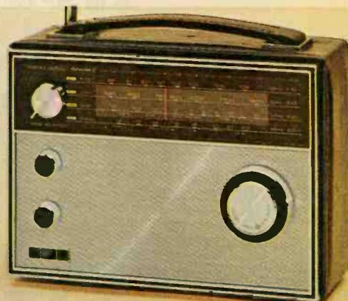
The low-priced 4-band portable that tells you what in the world is going on! FET/IC circuitry gets global broadcasts & all your FM/AM favorites. Fine-tuning on SW, tone control, 3 1/2" speaker, telescopic SW/FM antenna, built-in AM antenna, jack for external antenna. With earphone, 4 "C" cells. AC cord. 6 1/2 x 9 x 3 1/2". 12-774. U. L. listed.
