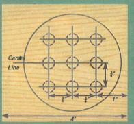
How to mark out the position of the Loudspeaker and  $\frac{3}{6}$  holes
