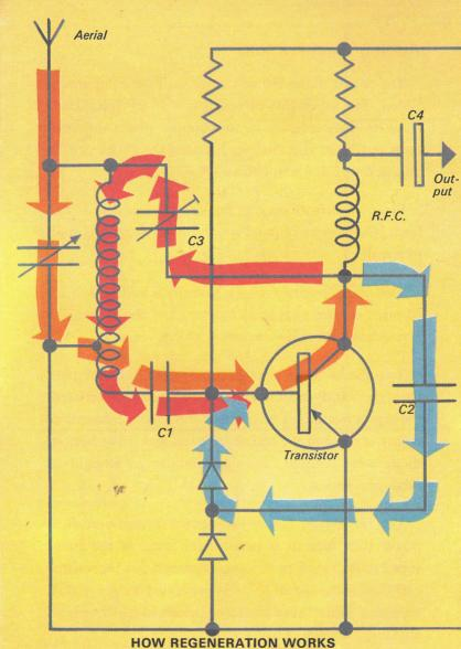
In circuit diagrams, wires which cross one another, (but do NOT touch and are NOT connected), are sometimes shown like this + (as in the diagram) or like this -. Shown like this - always means they are connected.
