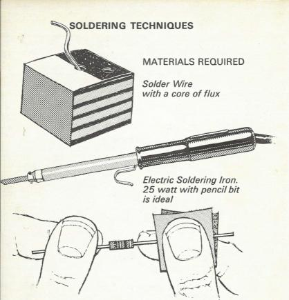
Clean both surfaces to be joined with sandpaper or the edge of a knife. The metal surfaces should be clean and bright
