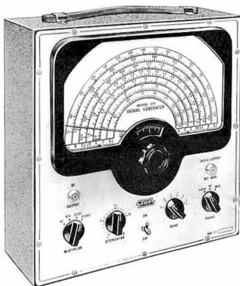
14-5. The Eico Model 315 signal generator covers a wide frequency band, and also provides 400-cps tone for audio testing.
