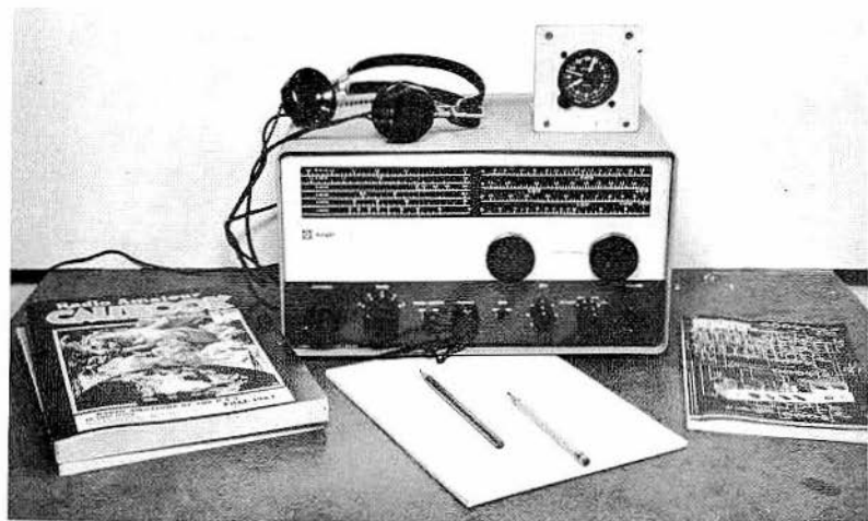
8-8. A listening post to keep a prospective amateur very busy. Completed Knight Kit R-55 receiver, with earphones and 24-hour clock on top; paper and pencils, callbook, and QST , ham magazine, on table.
