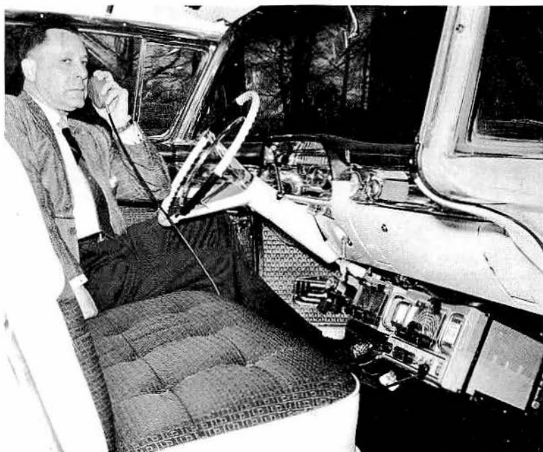
13-1. This under-dash mobile station uses separate units for transmission and reception. The operator is K2JHA, Harold Riker, M.D., of Flushing, N.Y.
