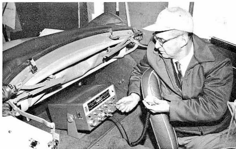
11-11. For mobile use, the Pawnee can be mounted under a dashboard, or, in a small sports car like this MG, on the jump seat behind the driver. A gimbal mount is furnished with the kit.
