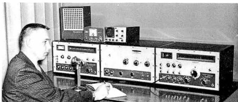
16-5. This beautiful layout is very professional looking, yet all its components were nut-and-bolt assembly jobs from Heath Kits. Left: Mohawk ham-band receiver. Center: Warrior 1-kilowatt power amplifier. Right: Marauder SSB-AM five-band transmitter. Top of receiver and amplifier: loudspeaker, phone patch, and monitor scope. The proud operator is Darwin Evans, K8ADS, Dowagiac, Mich.
