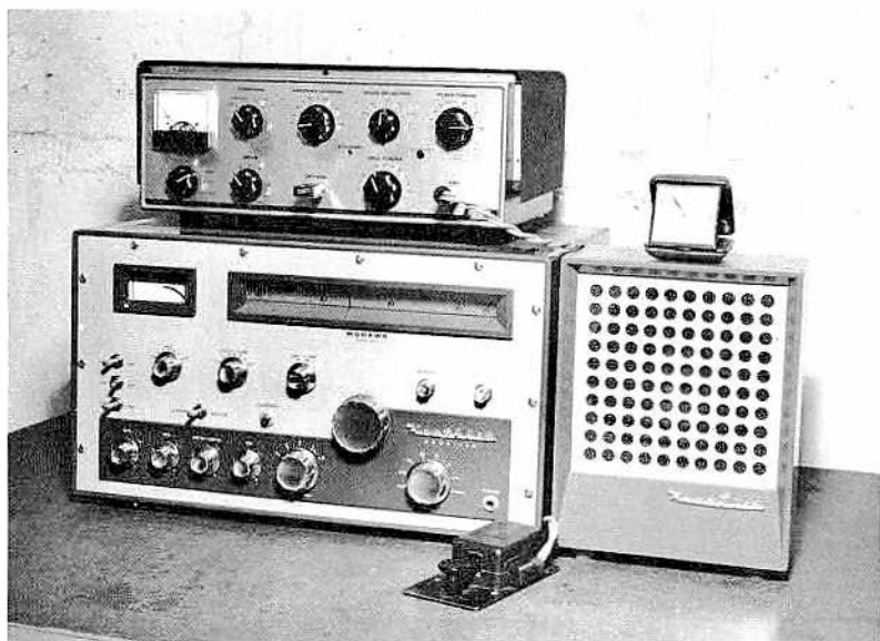
16-1. A small table in a corner of the basement holds this excellent combination of a Heath Mohawk ham-band receiver (bottom) and an Eico Model 720 CW transmitter. Both sets were made from kits. A modulator for an AM phone can be added at any time to the transmitter. The key in the foreground is completely insulated for shock protection.
