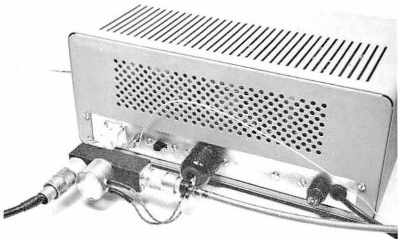
11-6. The coaxial relay, installed on the transmitter, shifts the antenna automatically from the transmitter to the receiver when the transmitter is energized.
