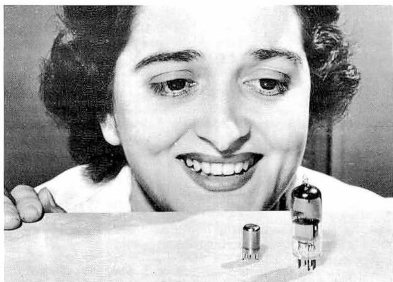
4-14. The metal-envelope Nuvistor tube (left) makes the glass "miniature" look large by comparison.
