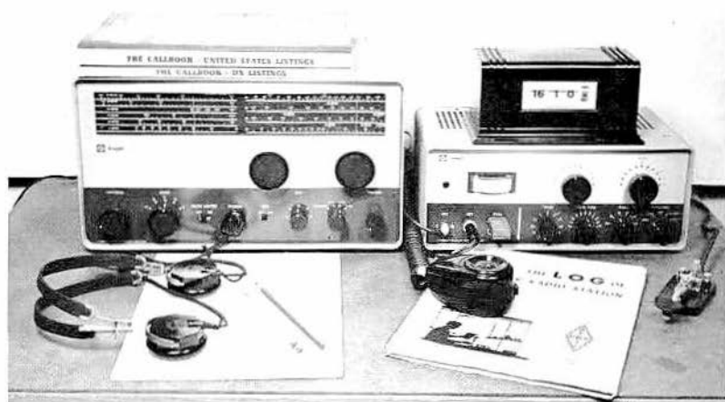
11-8. Many happy hours can be spent at this modest, attractive, and efficient amateur station. On top of the transmitter (right) is a 24-hour direct-reading clock.
