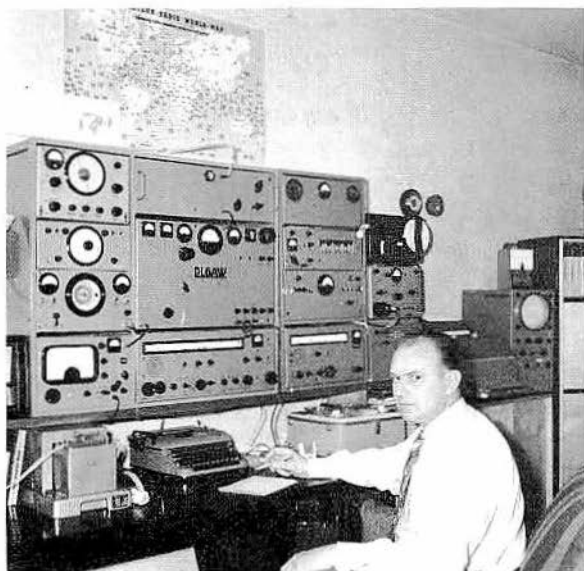
16-3. With the exception of a VTVM, an oscilloscope, and a teletype-writer sender, all the equipment in this interesting shack was handmade by the owner. He is DL6AW, Horst Rohmann, Braunschweig, Germany. A technician employed by the well-known Rolleiflex camera works, he is accustomed to precision construction to very high standards.
