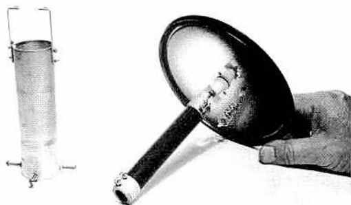
12-6. The dummy antenna consists of a noninductive resistor (right). It is mounted inside a protective shield (left).
