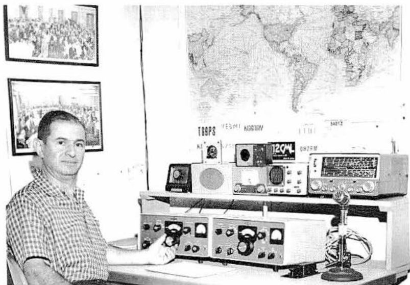
16-7. An extra shelf along the rear edge of a standard desk is a convenient location for station accessories. Left to right: beam indicator, loudspeaker for receiver (with 24-hour clock), standing-wave-ratio meter (with code oscillator), monitor scope, and Heath Mohican standby receiver. On the desk are a Collins 75S-3 receiver and 32S-1 transmitter, with an Electro-Voice microphone. This is the compact shack of W2DJJ, Robert Hertzberg, Douglaston, N.Y.
