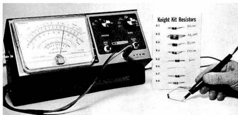
8-3. How to check small fixed resistors with VTVM to make sure their values correspond with their color-code markings.
