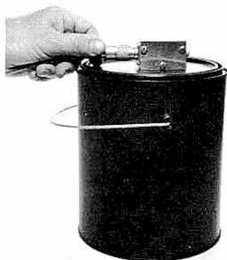
12-8. The coax from the transmitter terminates at the fitting on the top of the can. Over-all shielding keeps test signals off the air. This antenna was made from a Heath Kit.
