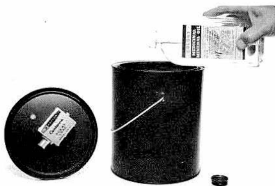
12-7. The can of a dummy antenna is filled with mineral oil to dissipate heat.
