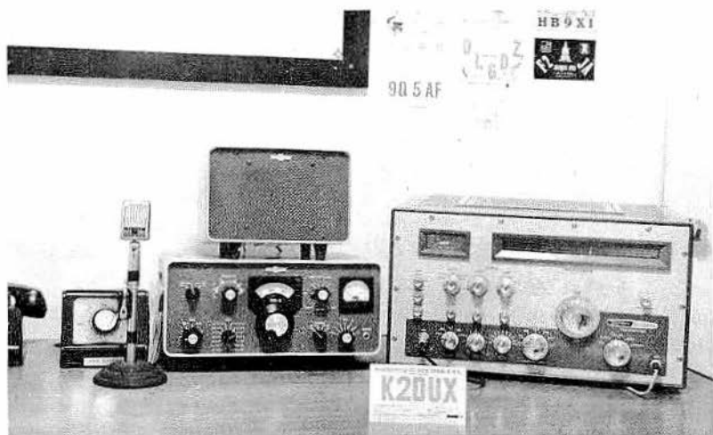
16-2. In the ham shack of K2DUX, Paul Hertzberg, Whitestone, N.Y., it is the receiver that is small and the transmitter comparatively large. The former is a Collins 75S-3, factory-made; the latter is a Heath Marauder, made from a kit. The unit behind the microphone is a beam-antenna position control and indicator. QSL cards from distant stations adorn the wall.
