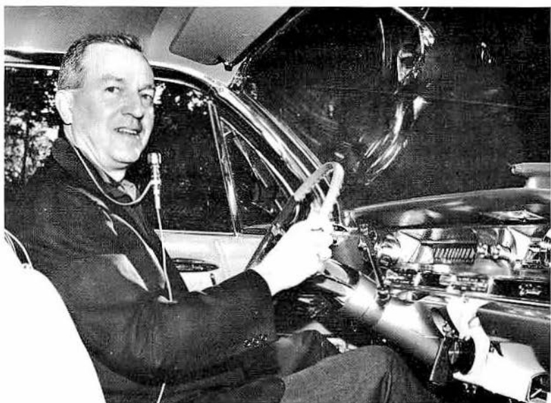
13-4. By leaving the transceiver on one frequency, and using a neck microphone and a foot-operated transfer switch, Bil can operate in motion. He has communicated all around the world with this installation.
