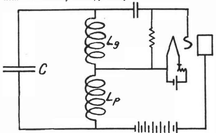
Fig. 4. Hartley Circuit as Used in the Laboratory.
