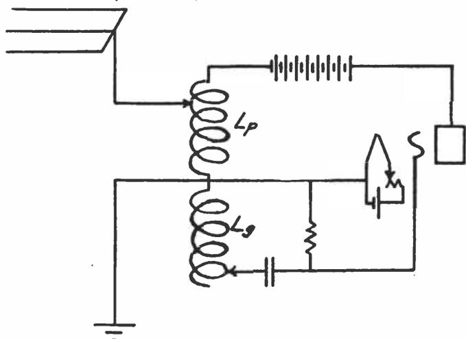
Fig. 5. Hartley Circuit as Used in Practice.
