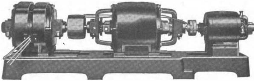
4 to 32 Volts for Filament—350 to 2000 Volts for Plate.
