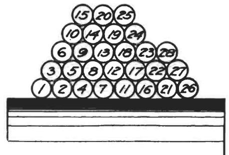
Fig. 4. Arrangement of Wiring for Five Bank Winding
