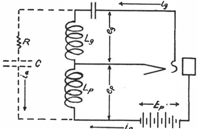
Fig. 2. Simplified Diagram of Hartley Circuit.
