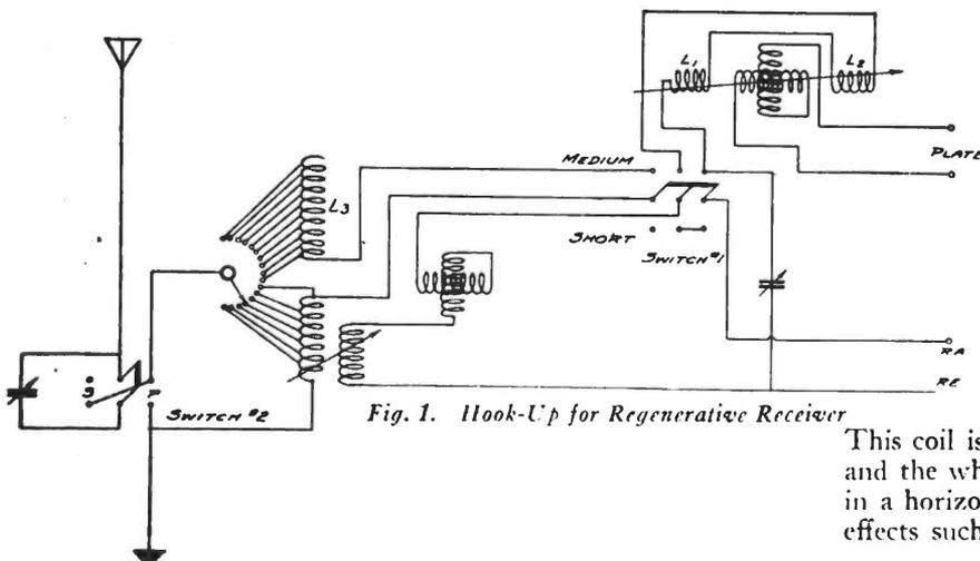
Fig. 1. Hook-Up for Regenerative Receiver
