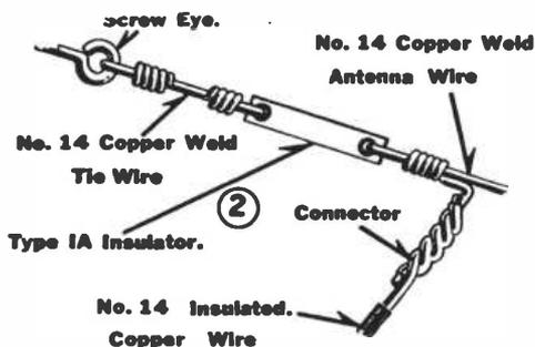
Fig. 2. Lead-In Connections
