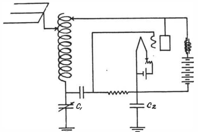
Fig. 10. Heising Circuit as Applied to the 938 set.
