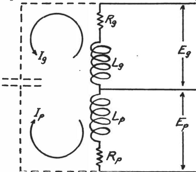
Fig. 3. Showing Direction of Grid Current and Plate Current.
