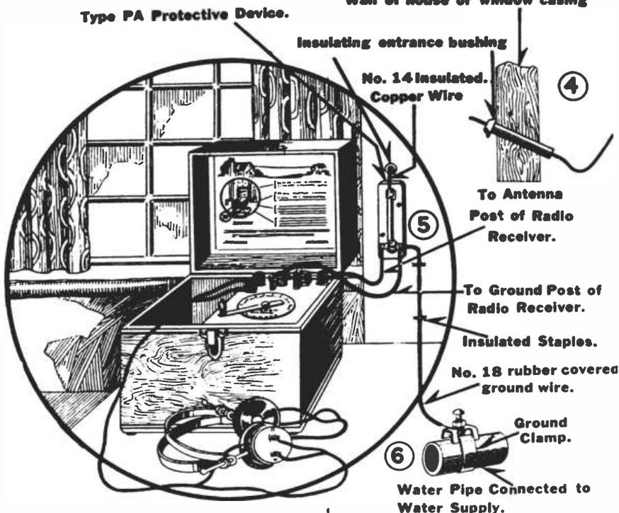
Fig. 4. Entrance, Instrument and Ground Connections
