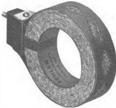
Fig. 2. Honeycomb Coil.
