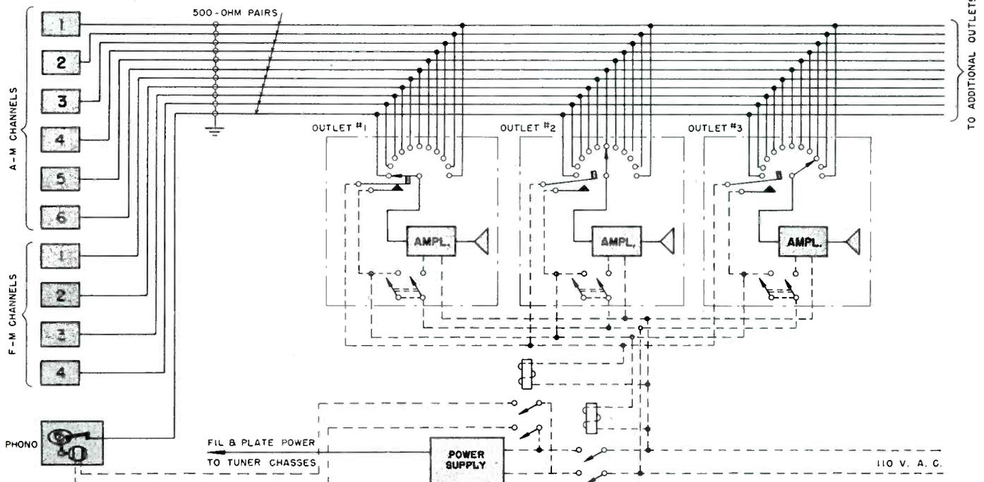
Fig. 2 The fully flexible system, providing a variety of programs available to each outlet, regardless of what any other outlet is playing. Especially suitable for large homes, particularly where there are children.
