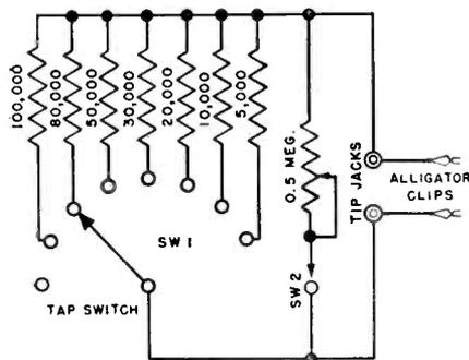
Fig. 2. Simple resistance box with switch used to determine proper value for shunt across filament dropping resistor.
