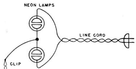
Ground detector composed of two 2-watt neon lamps, a line cord, and a test lead with a clip.
