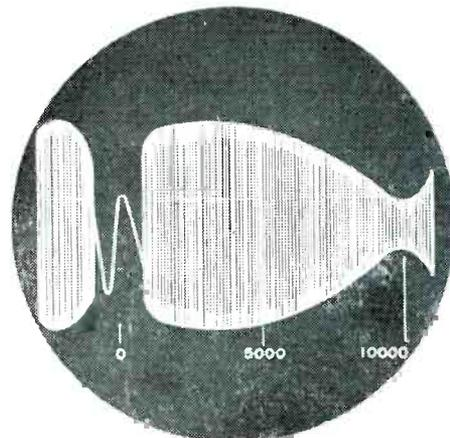
Fig. 6. Response curve obtained by beating two R-F oscillators together, one being frequency-swept, and feeding combined output to input of radio receiver of fairly good quality.
