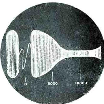
Fig. 7. Response curve of the same set as in Fig. 6, but with tone control set for minimum high frequency response.
