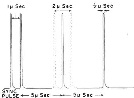
Fig. 2. Synchronizing double-pulse at left, and two pulses of the 24 used for multiplex telephony. Second pulse is shown with modulation which changes the pulse spacing.
