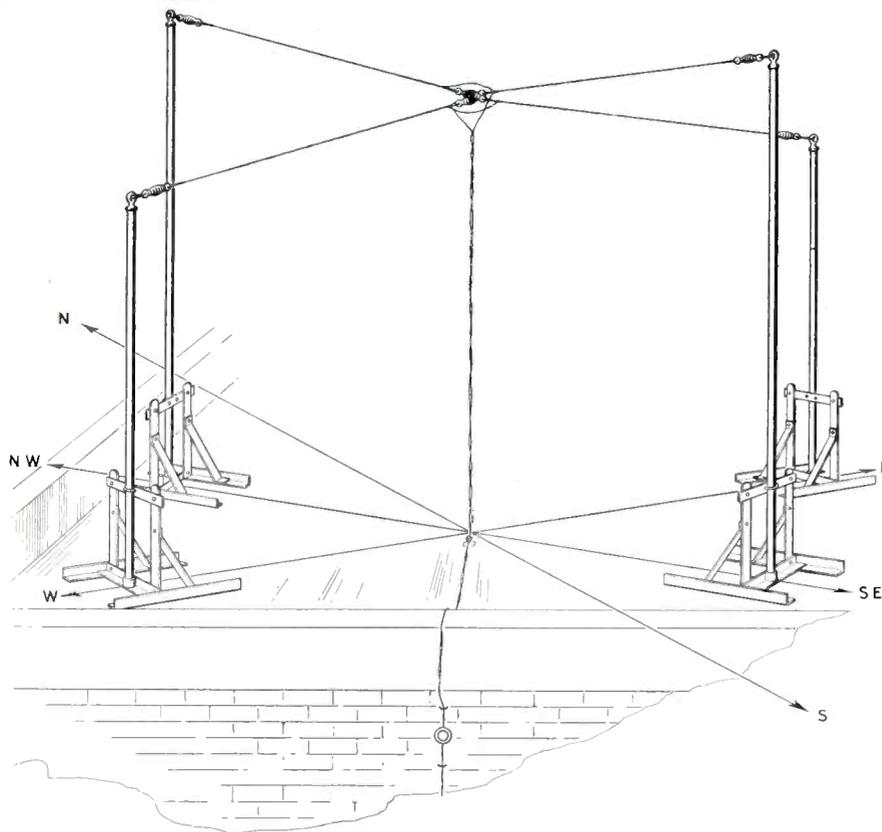
Fig. 6. One arrangement of double-doublet with one section favoring reception from one station, and the other section favoring a second station.
