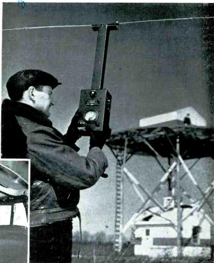
CAA Engineers making measurements on UHF range station.
