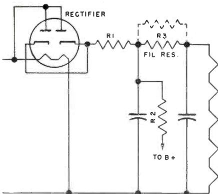
Fig. 1. Simplified schematic of typical filament circuit of AC-DC-Battery set to show location of shunt across dropping resistor.
