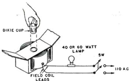
Using A-C to demagnetize the speaker temporarily enables the Dixie Cup to dislodge and remove iron filings that become attracted to the pole pieces.
