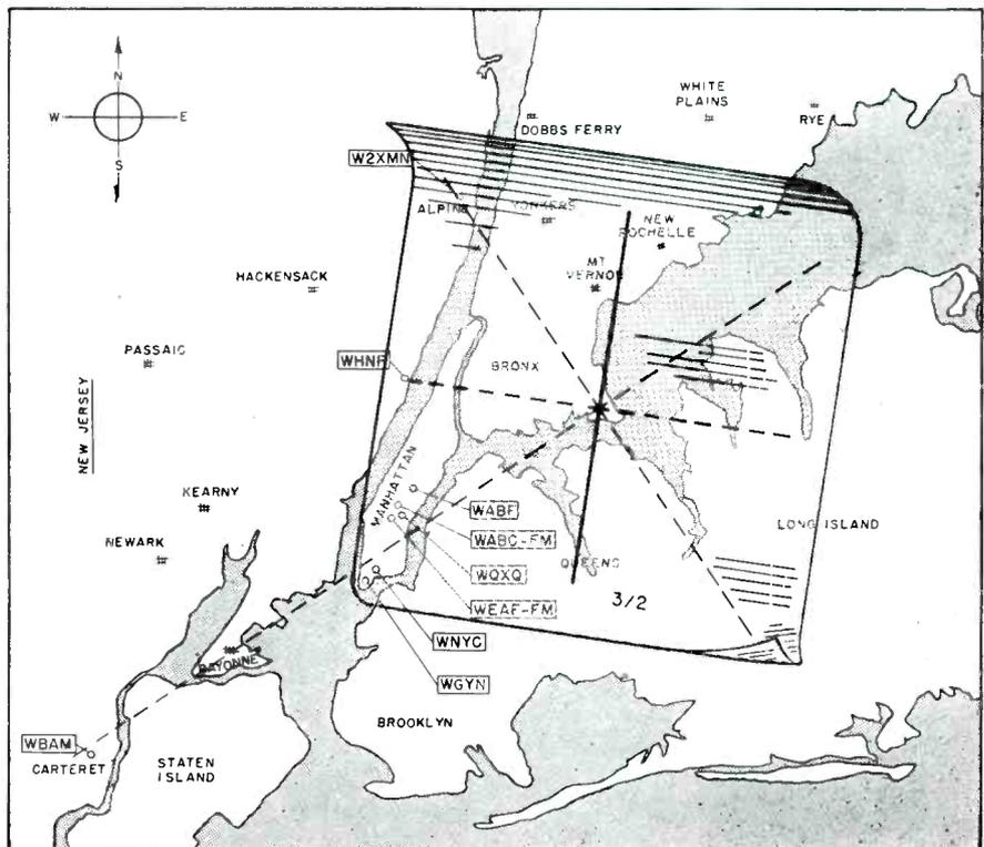
Fig. 5. Using a piece of acetate with axes of lobes of 3/2 wavelength antenna laid out on it to determine azimuth of antenna for optimum reception from several stations at customer's location.
