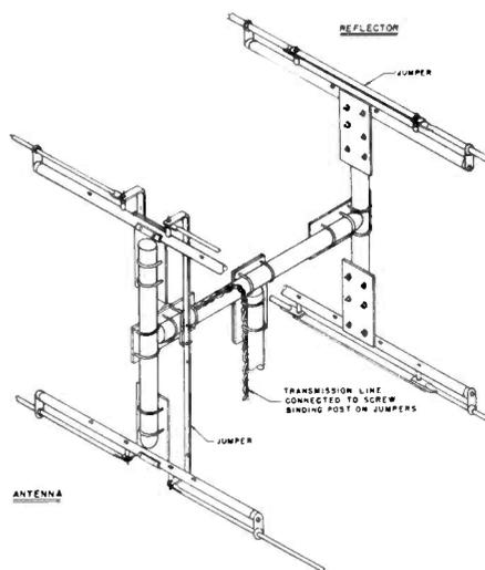
Fig. 7. Mounting of antennas and reflectors as manufactured by Technical Appliance Corp. (TACO) prior to the war.
