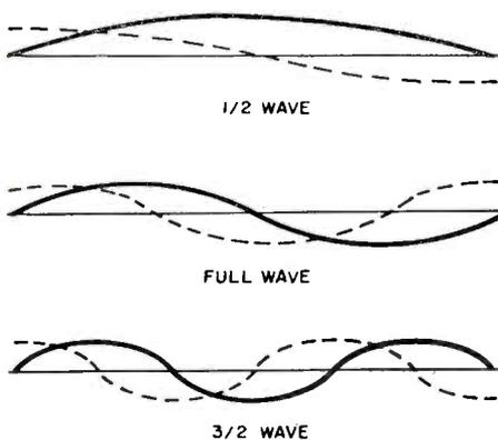
Fig. 2. Current waves (solid), and voltage waves (dotted) on antennas of various lengths.
