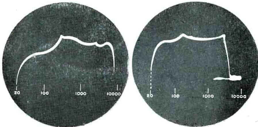
Fig. 5. Response curves obtained by method outlined in RCA Application Note 76. Left figure shows various resonances by peaks in the curve. Right figure indicates attenuation of high frequencies by tone control.
